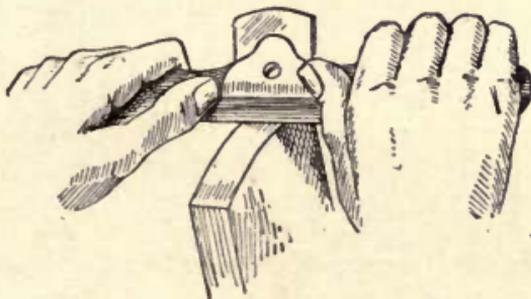
Fig. 77—Finishing with Spoke-Shave
