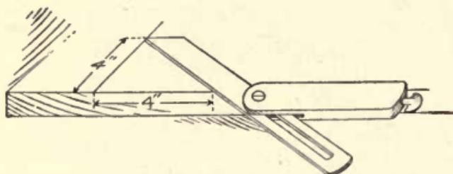
Fig. 58—Setting Angle of T-Bevel
