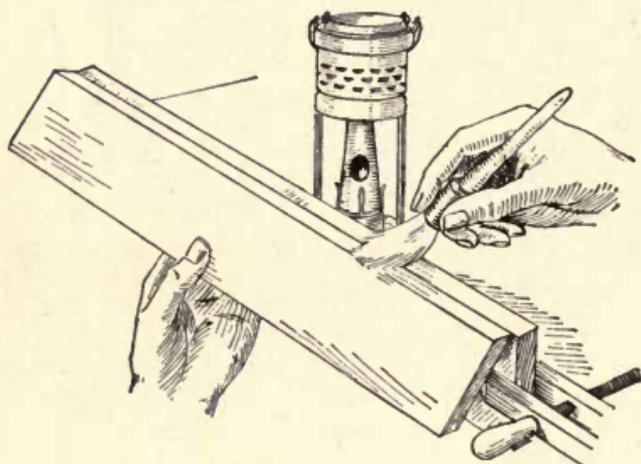
Fig. 106 — Applying Glue to the Edges
