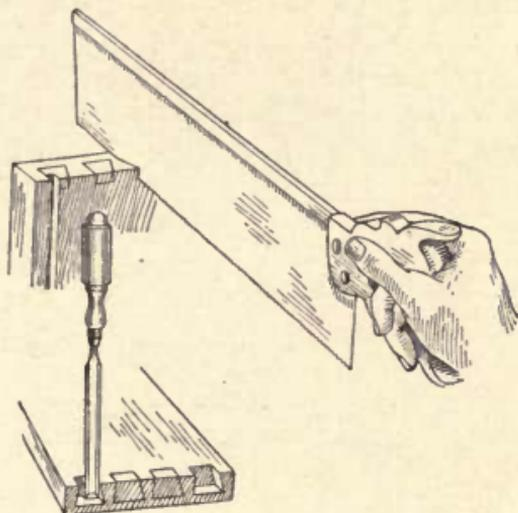
Fig. 120—Sawing the Mortises
