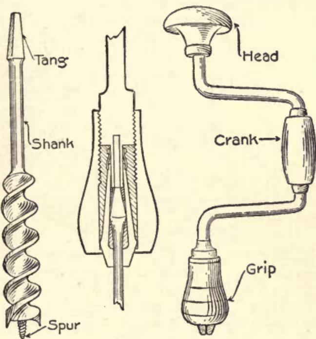
Fig. 61 — Brace and Bit
