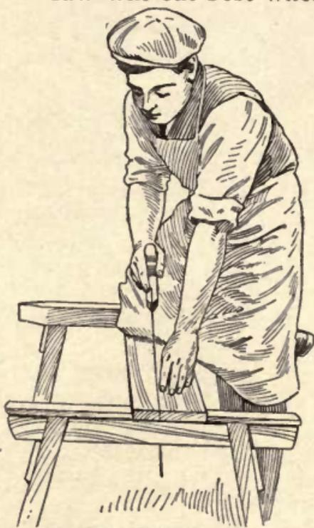
Fig. 16—Saw, Wrist and Elbow in One Plane
