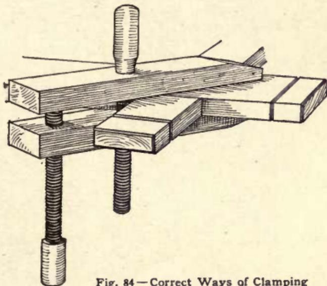
Fig. 84 — Correct Ways of Clamping
