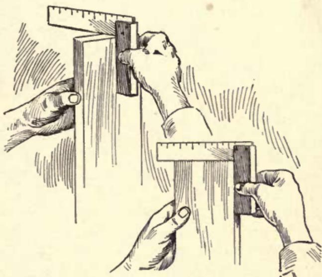
Fig. 39—End Testing
