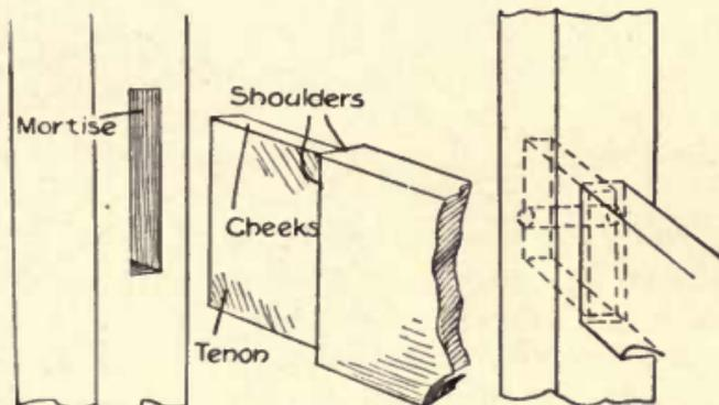
Fig. 108—Tenon and Mortise Joint
