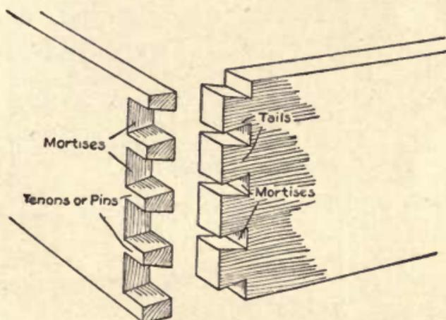
Fig 118—Dovetail Joint
