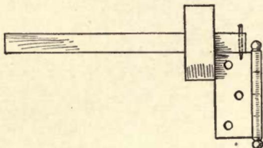
Fig. 122B — Finding Depth of Gain
