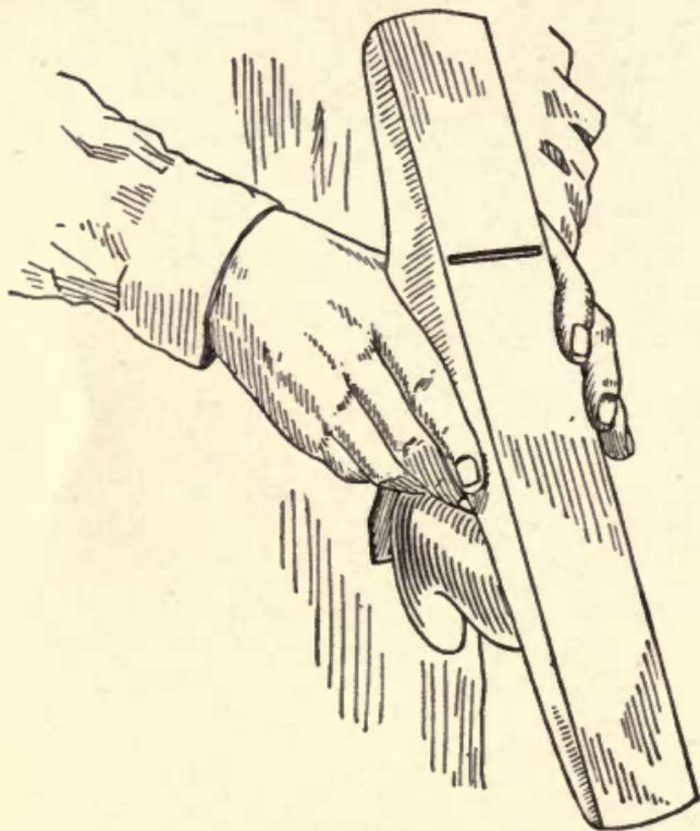
Fig. 26—Adjusting the Plane Iron
