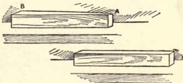
Fig. 42—Winding and a True Surface
