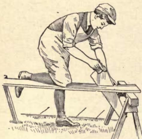
Fig. 15—Correct Angle of Saw
