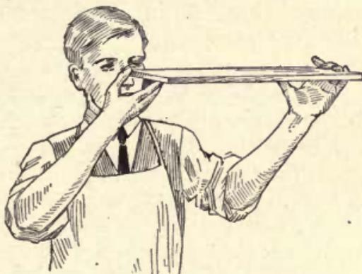
Fig. 44—Testing for Twist
