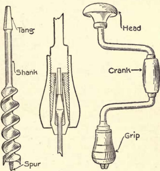
Fig. 61 — Brace and Bit
