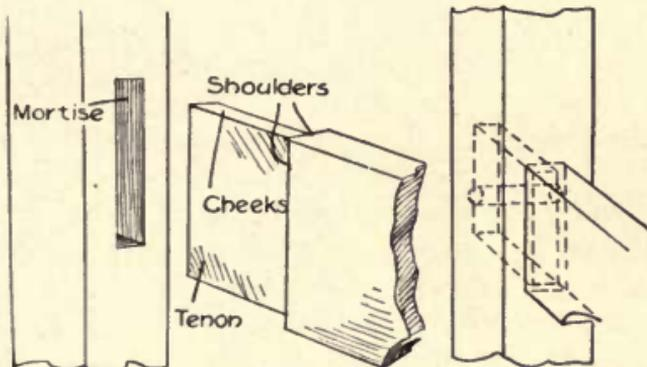
Fig. 108—Tenon and Mortise Joint
