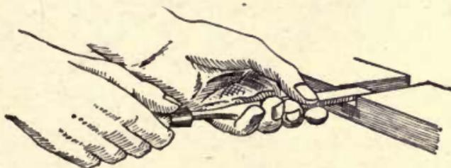
**Fig. 72B—Finishing with a Paring Cut**
