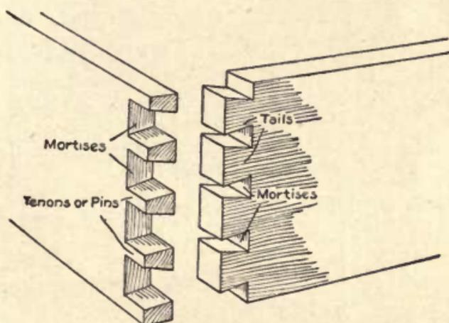
Fig 118—Dovetail Joint
