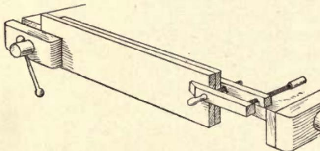
Fig. 104—Clamping Boards' Face Sides Together
