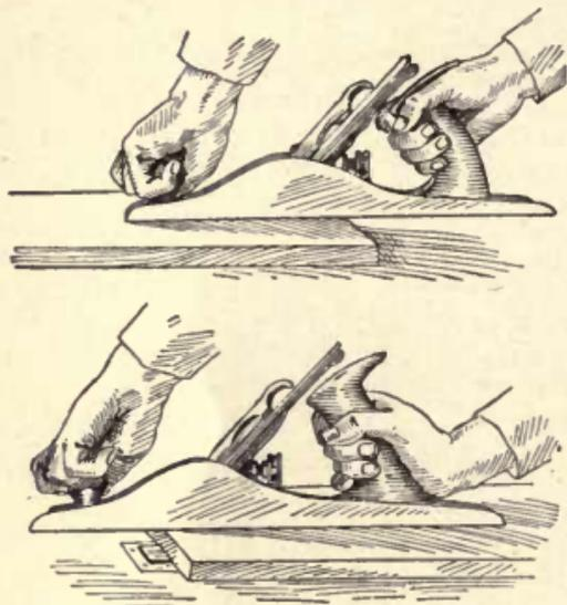
Fig. 29—Starting the Plane and Finishing the Stroke
