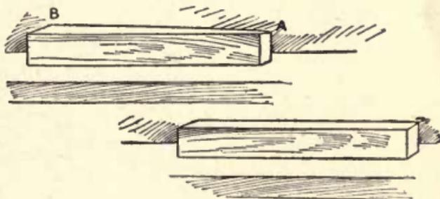
Fig. 42—Winding and a True Surface
