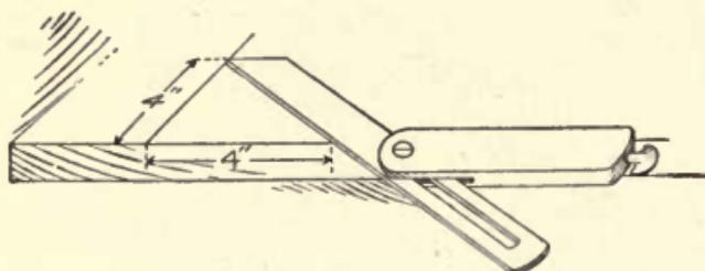
Fig. 58—Setting Angle of T-Bevel
