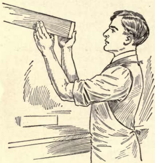
Fig. 43—Testing for Straightness
