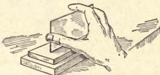
Fig. 91—Whetting and Removing the Wire Edge
