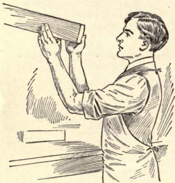
Fig. 43—Testing for Straightness
