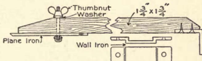
Fig. 55—Detail of Grinding Attachment
