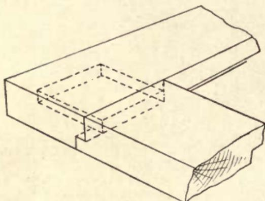
Fig. 116—Shouldered Tenon Joint for Glass Panel
