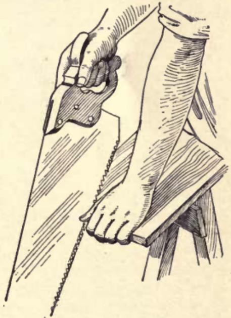
Fig. 14—Guiding the Saw with Left Thumb
