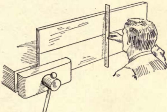
Fig. 105—Testing for Flat Surface
