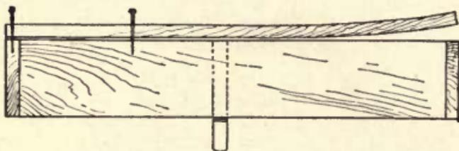
Fig. 31—Nailing Out "Dished" Board
