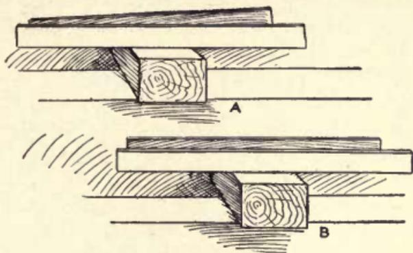
Fig. 46—Showing a Winding and a True Surface
