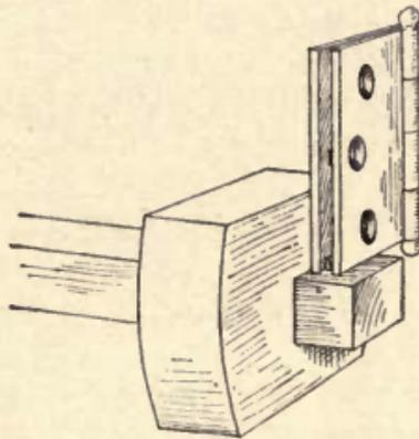
Fig. 122D—Setting Gauge for Depth
