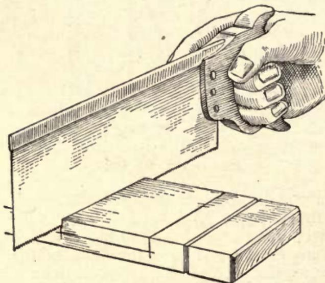
Fig. 83—Sawing on the Line
