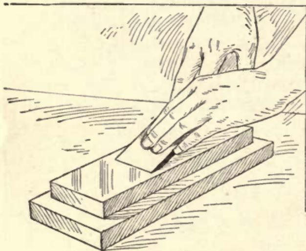
Fig. 49— Proper Pitch of Iron
