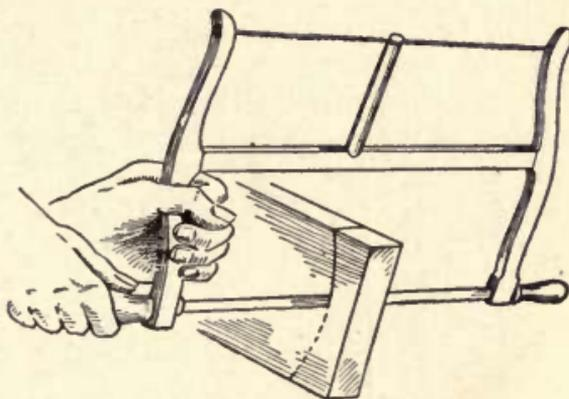
Fig. 76—Sawing the Curve
