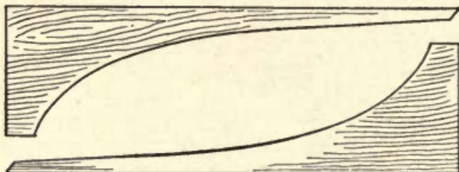
Fig. 88 — Cutting End Pieces without Waste
