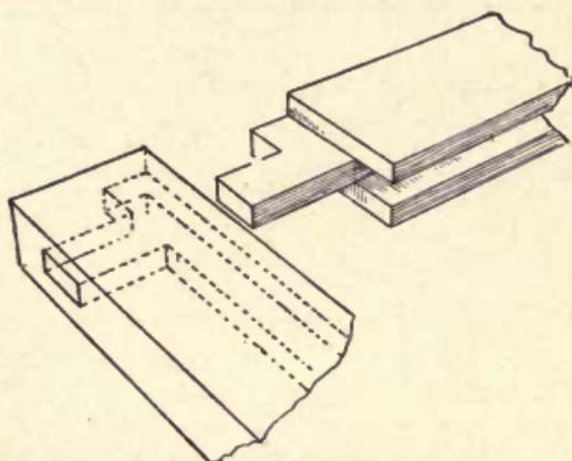
Fig. 115—Shouldered Tenon Joint
