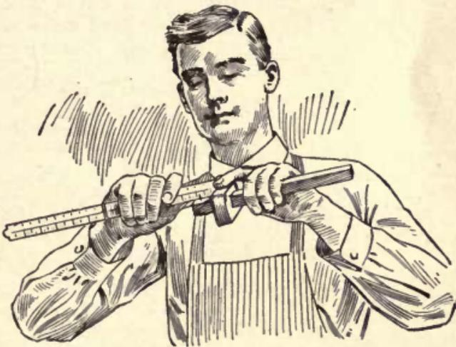
Fig. 36— Holding and Setting Marking Gauge
