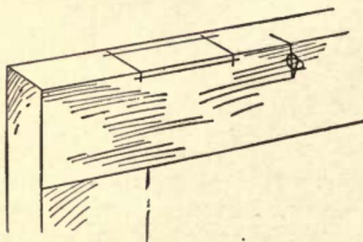
Fig. 122C — Gauged from Face Side
