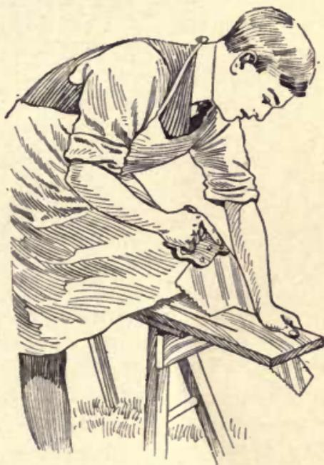
Fig. 17 — Holding Overhanging Piece
