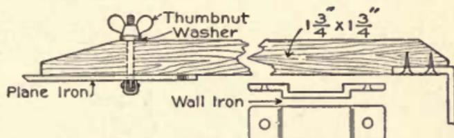
Fig. 55—Detail of Grinding Attachment
