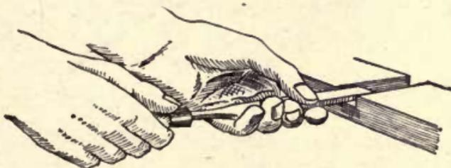
**Fig. 72B—Finishing with a Paring Cut**
