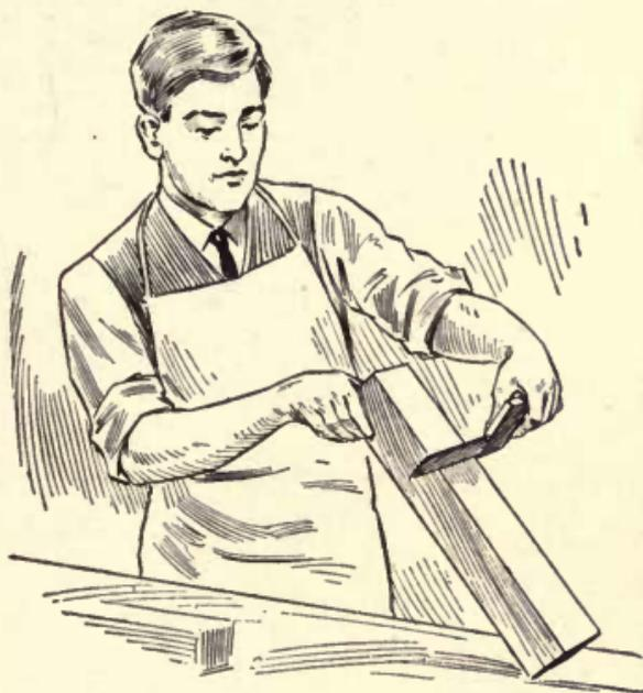
Fig. 47—Testing Across the Grain
