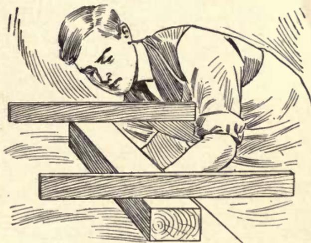
Fig. 45—Sighting for Winding of Surface
