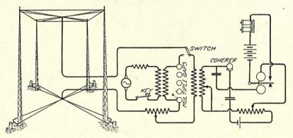
Fig. 63. Lodge-Muirhead Sending and Receiving Circuits
