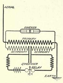
Fig. 19. Marconi Receiver-Circuit with Jigger
