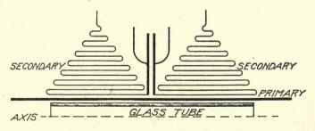
Fig. 18. Diagram of Oscillation Transformer Winding
