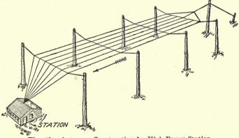
Fig. 42. Antennae Construction for High-Power Station
