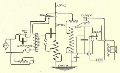
Fig. 60. Circuit Diagram, Telefunken System
