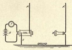
Fig. 2. Diagram of the Dolbear System
