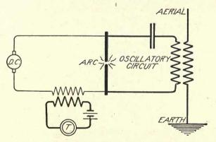
Fig. 8. Transmitter Associated with the Supply Circuit
