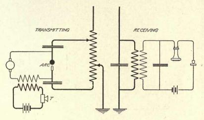
Fig. 17. Circuits of Poulsen System
