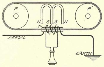
Fig. 50. Diagram of Marconi Magnetic Detector
