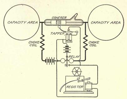
Fig. 13. Early Marconi Receiving Circuit
