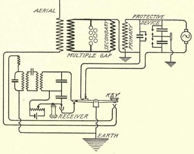
Fig. 65. Stone Sending and Receiving Circuits
