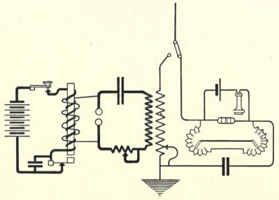
Fig. 64. Clark Sending and Receiving Circuits
