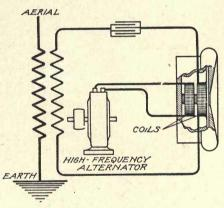
Fig. 13. Heterodyne Receiver Circuit
