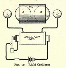
gations of this character. The dimensions of the oscillator could thereby be reduced and the amplitude of the oscillations greatly increased by reason of the fact that higher potentials could be reached before the energy was released by discharge. Righi obtained oscillations of a frequency of 12,000,000,000 vibrations per second by the use of small spheres A and B eight millimeters in diameter.
