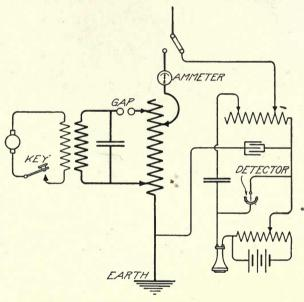
Fig. 66. Massie Sending and Receiving Circuits
