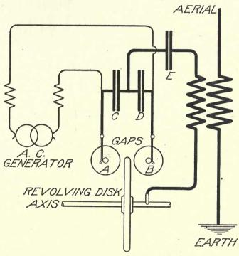
Fig. 32. Diagram of Marconi High-Speed Disk Discharger
