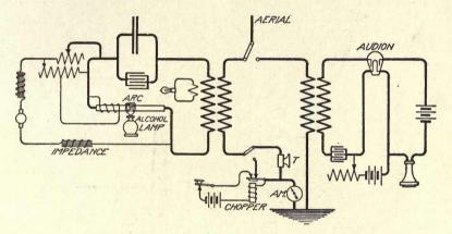
Fig. 19. Operating Circuits of the DeForest System
