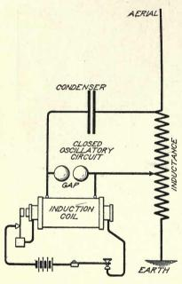
Fig. 21. "Direct-Coupled" Inductive Antennae
