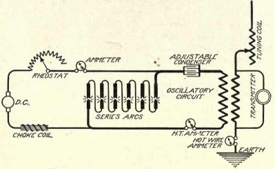
Fig. 14. Transmitter Circuit of the Telefunken System
