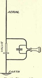
Fig. 46. Diagram of Dun woody Detector
