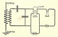
Fig. 49. Receiving Circuit with Audion Detector
