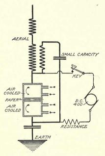
Fig. 61. Von Lepel Oscillation Generator Circuit
