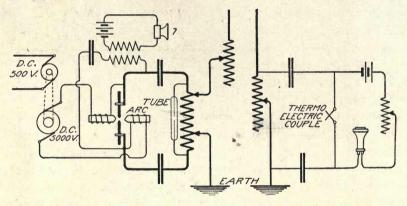
Fig. 20. Circuits of the Collins System
