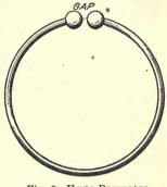
Fig. 6. Hertz Resonator
