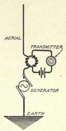
Fig. 7. Transmitter Inductively Associated with Aërial
