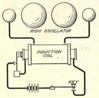
Fig. 12. Early Marconi Transmitter Circuit
