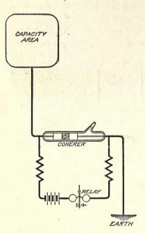
Fig. 16. Earthed Receiving Circuit
