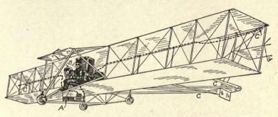
Fig. 3. Diagram Showing Location of Circuits and Equipment of a Wireless Outfit
