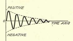
Fig. 3. Curve Representing an Oscillatory Discharge
