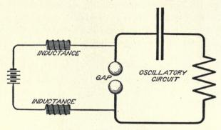
Fig. 34. Thomson Direct-Current Method of Generating Oscillations
