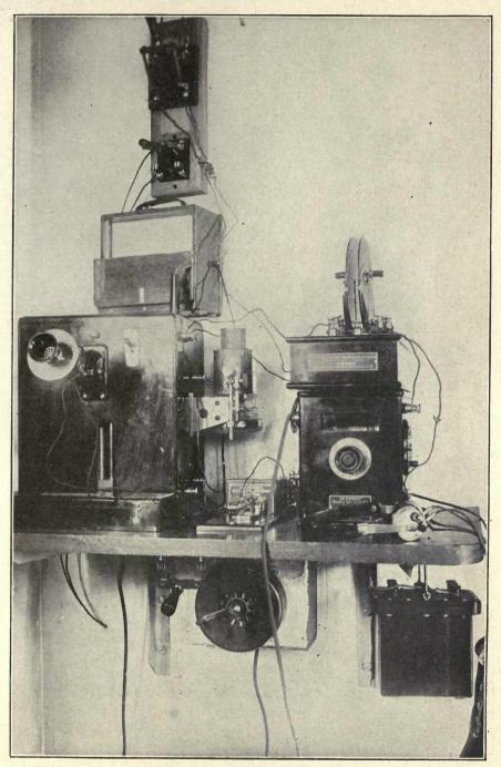
THE FIRST SIT OF WIRELESS TELEPHONE INSTRUMENTS FOR THE UNITED STATES NAVY Installed on the Flagship "Connecticut." The "Audion" Receiver with Tuning Device on the Top at Right, the Transmitter on the Left.
