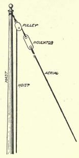
Fig. 41. Single Wire Experimental Aërial
