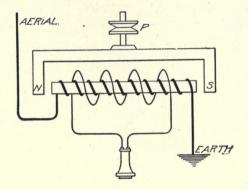
Fig. 51. Shoemaker Magnetic Detector
