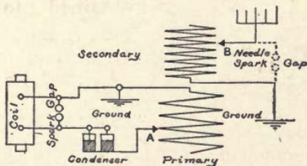
Fig. 65. Loosely Coupled Transmitting Circuit.
