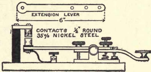
Fig. 67. Morse Key fitted with Extension Lever.
