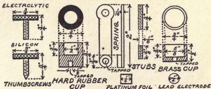
Fig. 90. Parts of Universal Detector.
