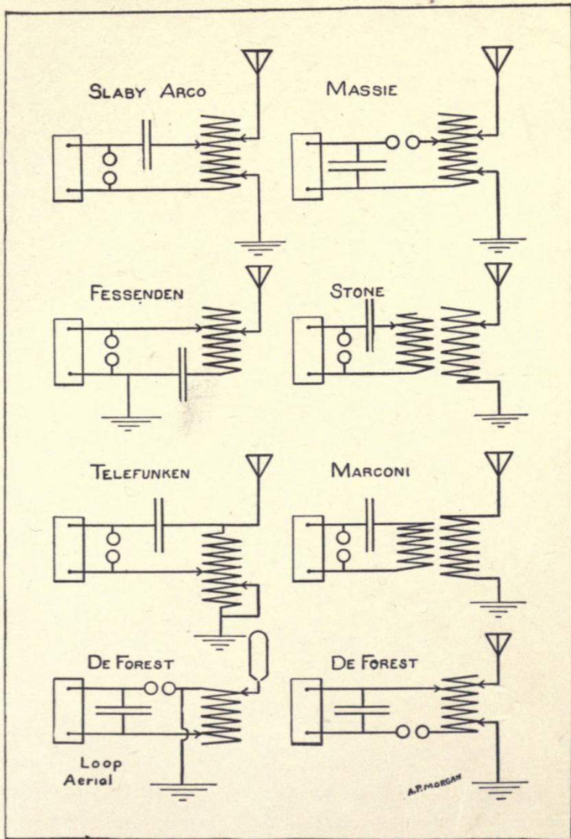
Plate III. Transmitting Circuits.
