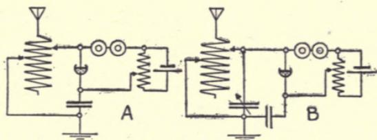
Fig. 137. Tuning Circuit with and without an Adjustable Condenser.
