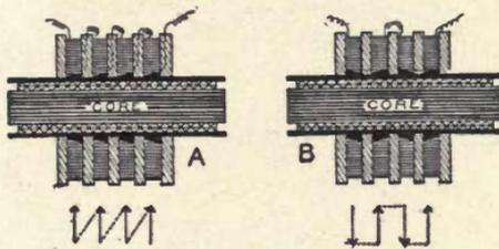
Fig. 31. Methods of Connecting the Secondary Sections.
