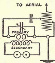
Fig. 117. Circuit of Magnetic Detector.
