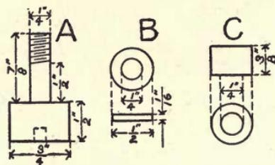
Fig. 116. Pulley Bearings.
