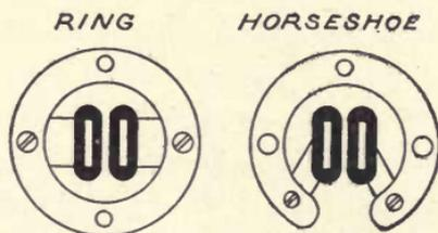
Fig. 142. Types of Permanent Magnets.
