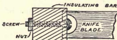
Fig. 74. Method of Fastening Knife.
