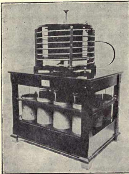
Fig. 66. United Wireless Helix, Spark Gap and Condenser.
