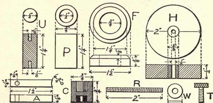
Fig. 101. Details of Electrolytic Detector.
