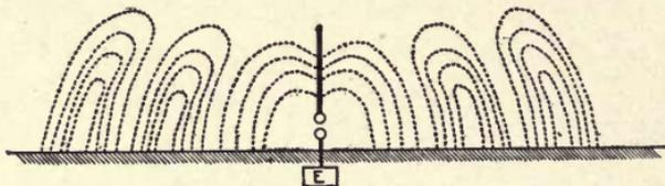
Fig. 5. Electric Waves and Lines of Strain.
