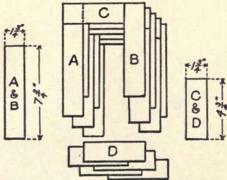
Fig. 44. Assembly and Dimensions of Core.
