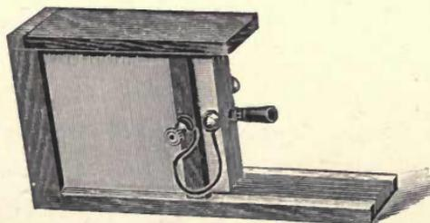
Fig. 141. Sliding Plate Variable Condenser.
