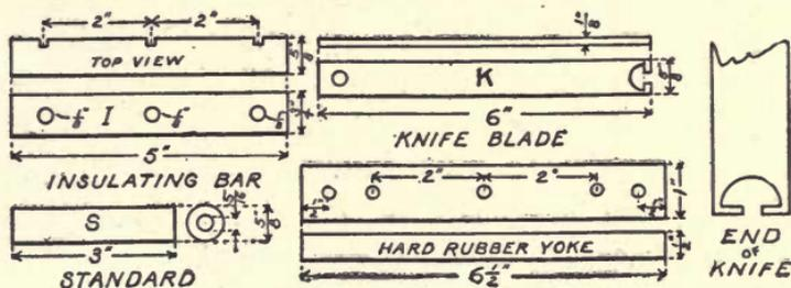
Fig. 73. Details of Switch Parts.
