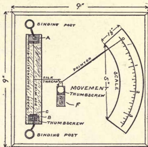
Fig. 81. Meter with Case Removed.
