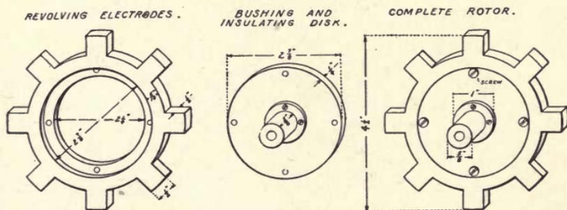
Fig. 158. Details of Revolving Parts of Rotary Gap.
