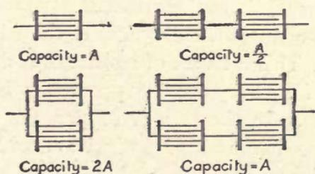
Fig. 58. Methods of Varying Capacity.
