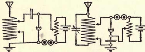
Fig. 123. Double-slide Tuning Coil Circuits.
