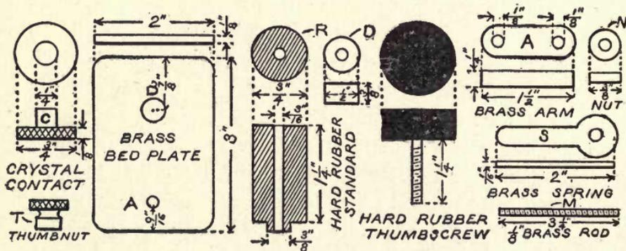
Fig. 89. Details of Universal Detector.
