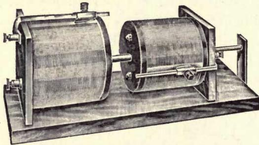
Fig. 133. Clapp-Eastham Loose Coupler.
