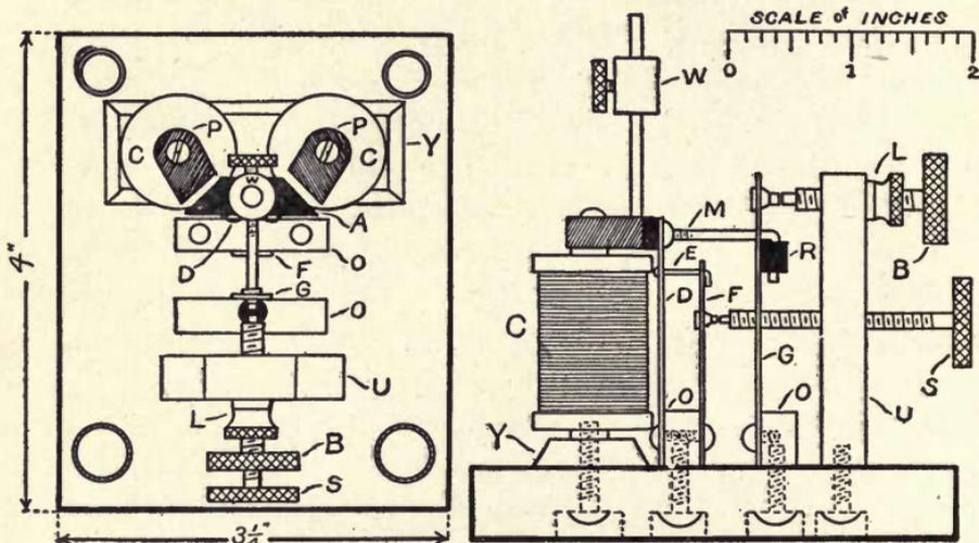
Fig. 34. Independent Interrupter.
