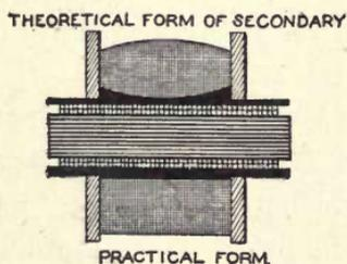
Fig. 27. Theoretical and practical form of secondary.
