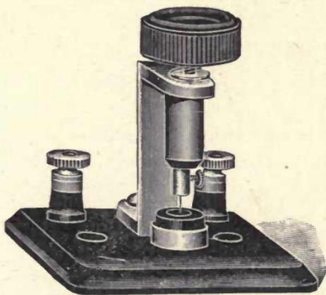
Fig. 94. Electrolytic Detector.
