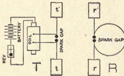
Fig. 1. Hertz Oscillator and Resonator.
