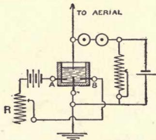
Fig. 102. Increasing the Sensitiveness of an Electrolytic Detector.
