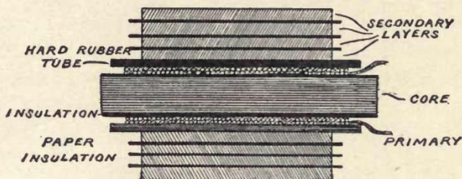
Fig. 28. Layer Winding for Small Coils.
