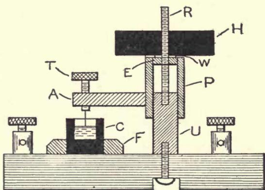
Fig. 100. Electrolytic Detector.
