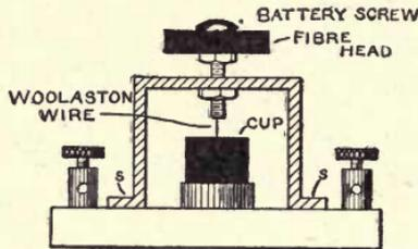
Fig. 99. Simple Electrolytic Detector.
