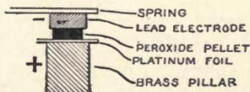
Fig. 111. Peroxide of Lead Detector.
