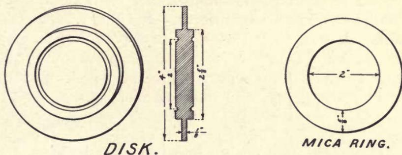
Fig. 155. Details of Disk and Ring.
