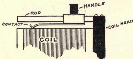
Fig. 130. Slider for Loose Coupler.
