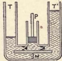
Fig. 2. Hydraulic Oscillator.
