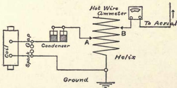
Fig. 63. Closely Coupled Tuning Circuit.
