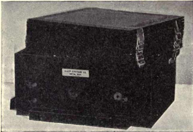
Fig. 57. Clapp-Eastham Oscillation Condenser.
