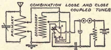
Fig. 132. Combination Loosely and Closely Coupled Tuner.
