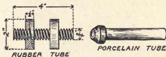
Fig. 20. Insulating Tube.
