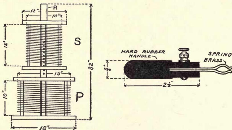
Fig. 64. Loosely Coupled Transmitting Helix and Contact Clip.
