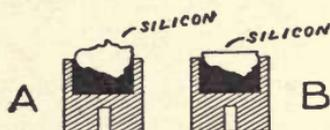
Fig. 107. Silicon Crystal in Cup.
