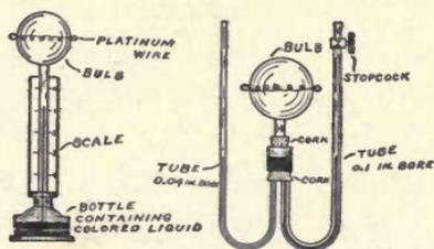
Fig. 80. Simple Hot Wire Meter.
