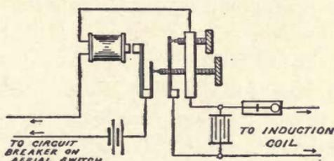
Fig. 38. Diagram of Connections for an Independent Interrupter.
