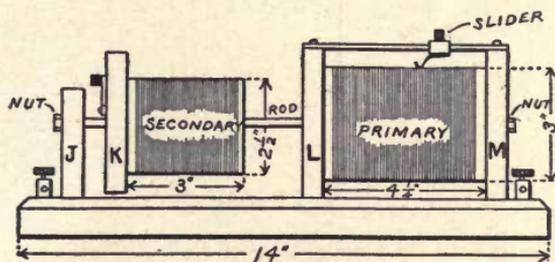
Fig. 127. Oscillation Transformer.
