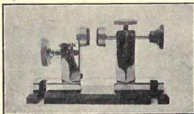
Fig. 104. United Wireless Carborundum Detector (horizontal type).
