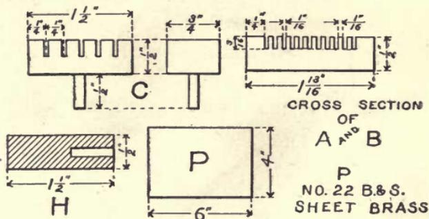
Fig. 140. Details of Variable Condenser.
