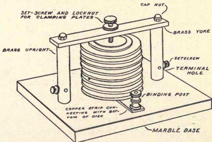
Fig. 156. Explanatory Drawing of Quenched Gap.
