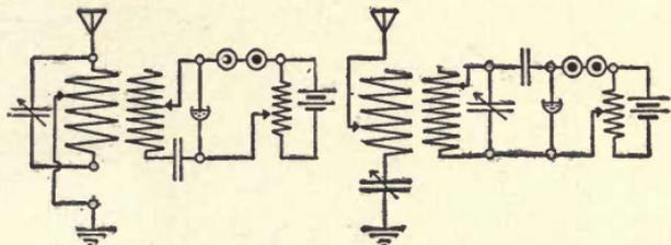
Fig. 131. Loosely Coupled Tuning Circuits.
