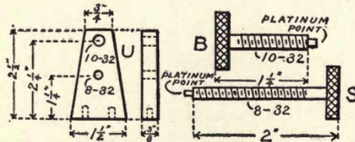
Fig. 37. Details of Standard and Screws.
