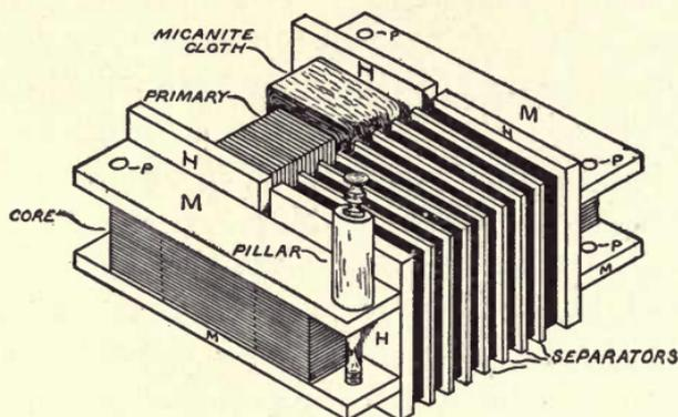
Fig. 49. Transformer with One Secondary removed.
