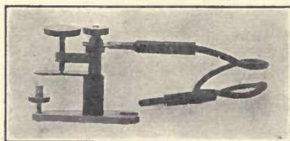
Fig. 105. United Wireless Carborundum Detector
