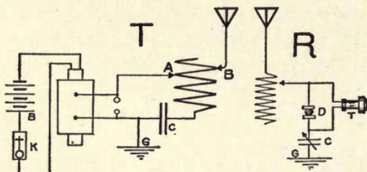
Fig. 9. Tuned Wireless Telegraph Transmitter and Receptor
