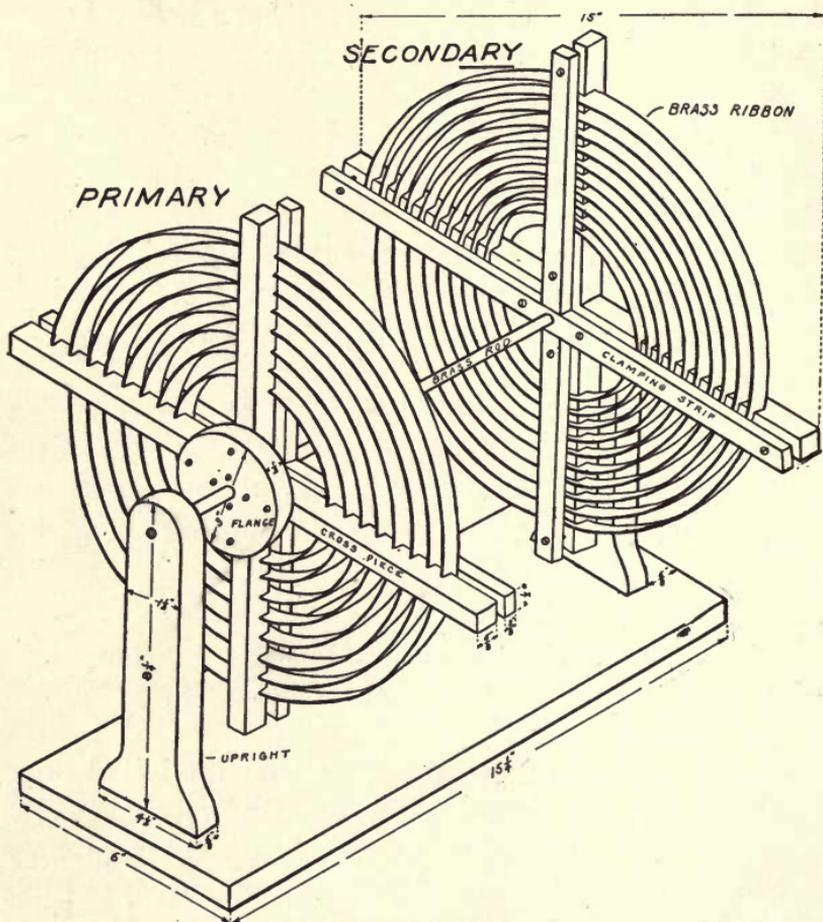
Fig. 152. Details of Oscillation Helix Construction.
