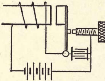
Fig. 33. Simple Interrupter.
