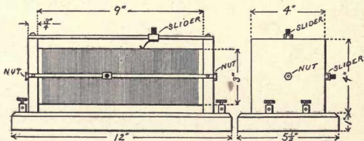
Fig. 121. Double-slide Tuning Coil.
