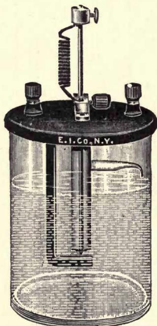
Fig. 43. Electrolytic Interrupter.
