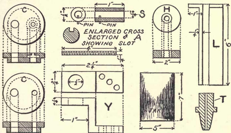
Fig. 42. Details of Electrolytic Interruptioners.
