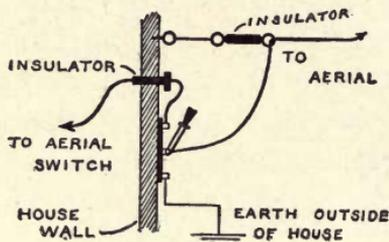
Fig. 24. Switch for Lightning Protection.
