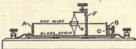
Fig. 86. Side View of Hot Wire and Movement.
