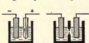
Fig. 40. Wehnelt and Simon Electrolytic Interrupters.
