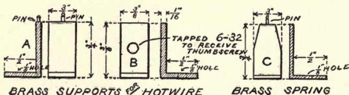
Fig. 83. Details of "Hot Wire" Supports.
