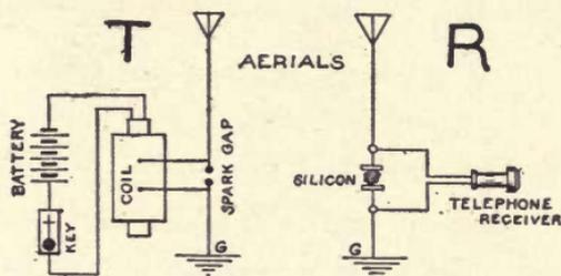
Fig. 4. Simple Wireless Telegraph Transmitter and Receptor.
