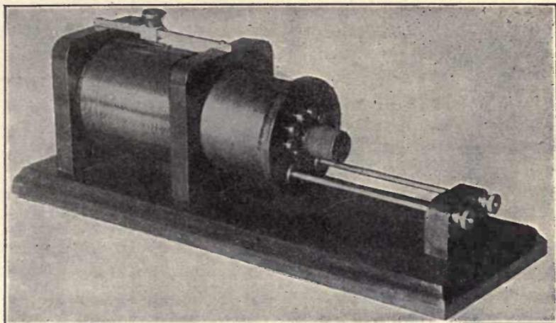
Fig. 134. A Highly Efficient Form of Loose Coupler.
