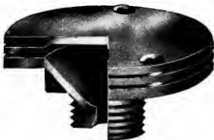
FIG. 50. —Strainer or Sand Valve.
