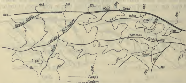
SKETCH NO. 216.—Relation between Distributaries and Contour Lines.
