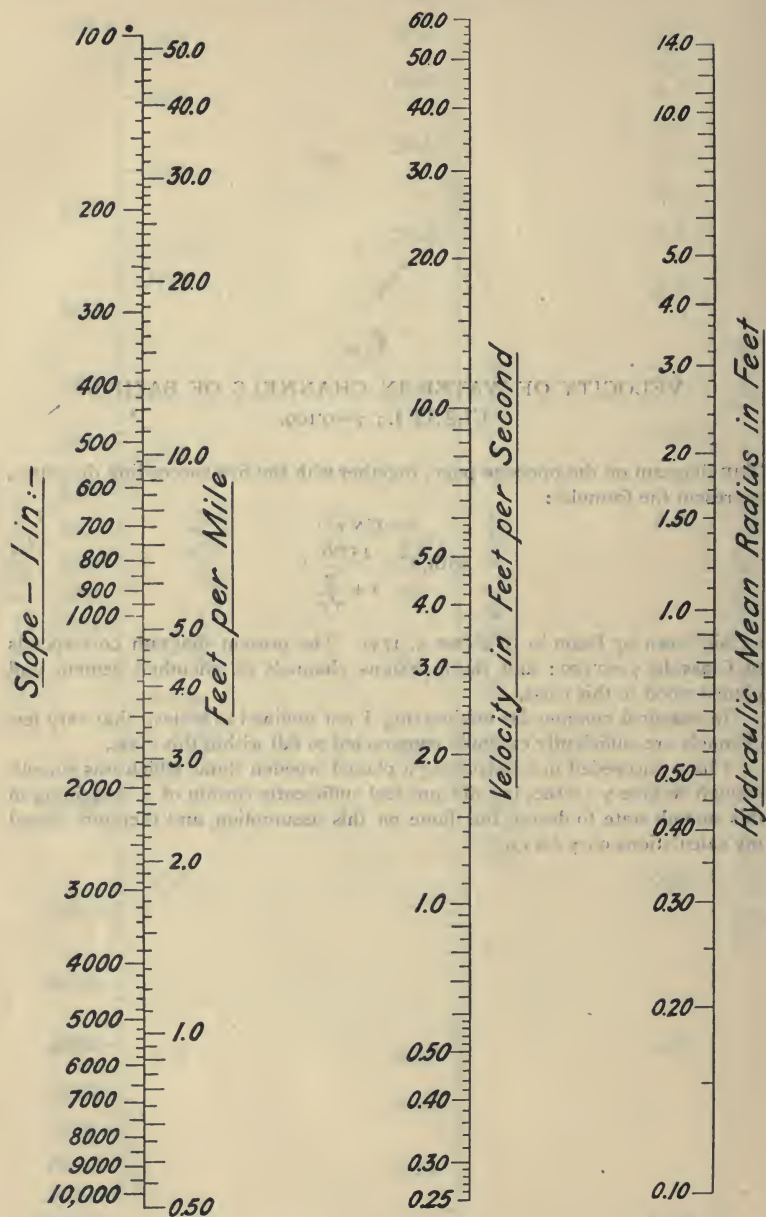
Diagram No. 7.—VELOCITY OF WATER IN CHANNELS OF BAZIN'S CLASS II.; \gamma=0.290 .
