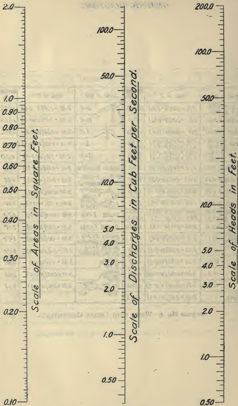
Diagram No. 5.—DISCHARGE OF ORIFICES.
