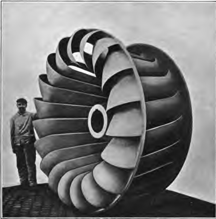
FIG. 15A.—Mixed flow turbine.
