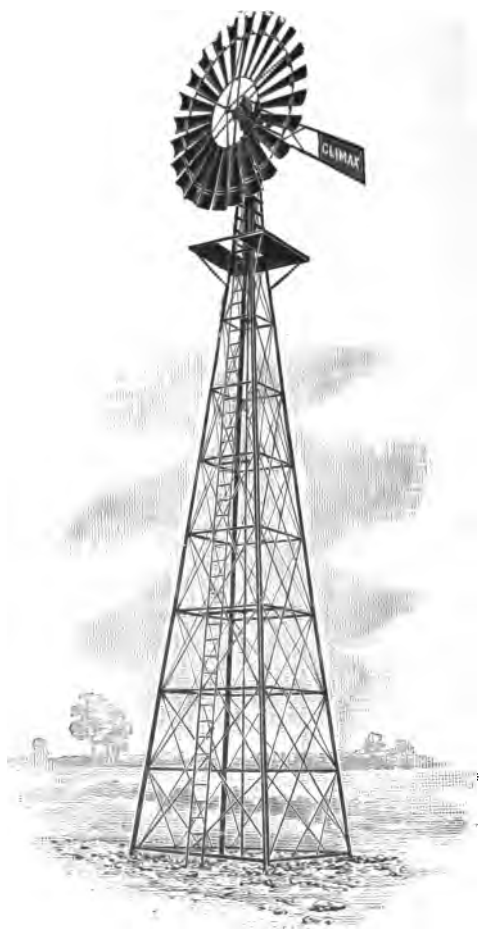
FIG. 79.—Steel Windmill and Tower.
