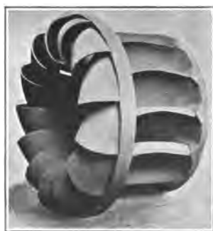
FIG. 15.—Mixed flow turbine.
