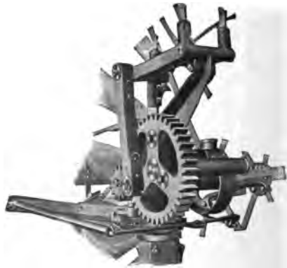
FIG. 86b.—Head of Mill showing Gearing.
