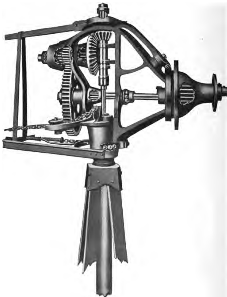
FIG. 90.—Bevel Gear Transmission.
