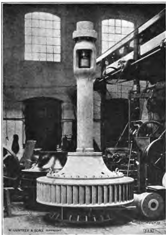
FIG. 19.—Radial outward flow Girard turbine of 525 h.-p.
