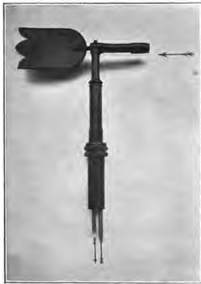
FIG. 67.—Head of Dines Wind Pressure Recorder (R. W. Munro).
