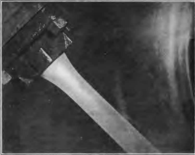
FIG. 32.—Jet issuing from nozzle at high velocity.
