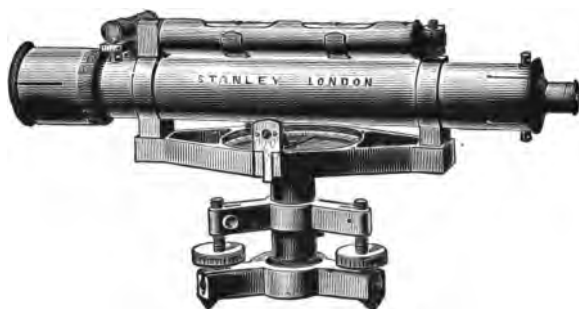
FIG. 5.—The engineers' level.
