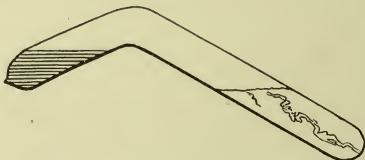
FIG. 7.—Faraday's Tube for Liquefying Carbon Dioxide.
