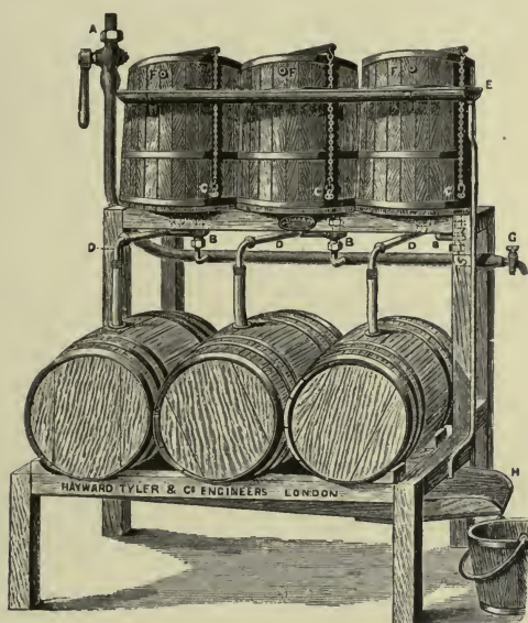
FIG. 107.—Apparatus for Filling Casks with Ginger Beer.
