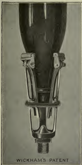
FIG. 95.—Wickham's Patent Rinser with Bottle in Position.
