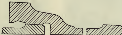
FIG. 35. — Bored Bell and Turned Spigot Pipe-joint.
