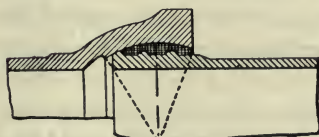
FIG. 82. — Stop Rings on Spigot.
