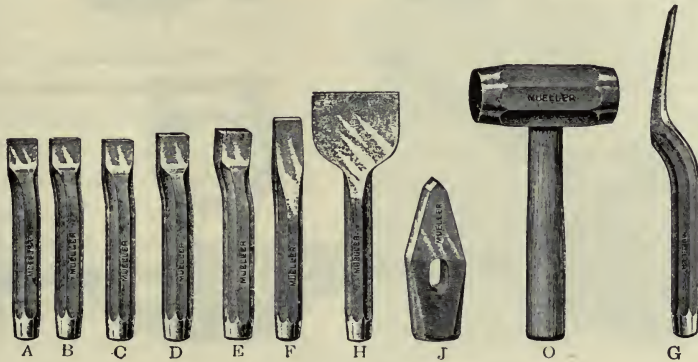
FIG. 267. — Set of Caulking Tools.
