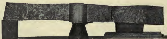
FIG. 70. — Lock-bar Pipe, Tested to Rupture.
