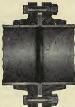
FIG. 66. — Pipe-joint for High Pressure.
