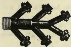
FIG. 248. — Branch-connection from Iron Service-pipe.*
