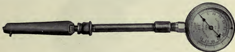
FIG. 229. — Hydrant Pitot Tube.
