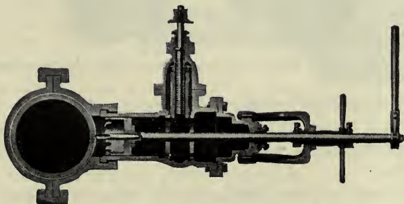
FIG. 276. — Smith Tapping Machine for Branch-connections.
