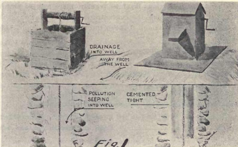
In the case of wells and springs, due to the filtering and purifying action of the soil, water from such sources is usually pure unless contaminated by some man-made cause, such as privies, cess-pools or barn yards. See Fig. 1. For wells and springs, then, the problem is primarily one of protection.
