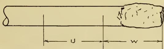
Stock left over from tension tests of which the results are tabulated in Table V. Section U was used for tests a, b, and c. Section W was used for compression tests on welded aluminum.
