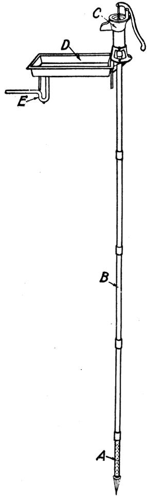
FIG. 26.—Driven well in the home. Where conditions are favorable, this is the quickest and cheapest method of getting ground water to the kitchen sink. *A*, Well point; *B*, drive pipe; *C*, pitcher or kitchen pump; *D*, sink; *E*, lead trap and waste pipe to connect with an absolutely water-tight carrier extending not less than 100 feet in a downhill direction from the well. The cost of a pump, sink, and 1½-inch well 20 feet deep installed as shown should not be more than \$20.
