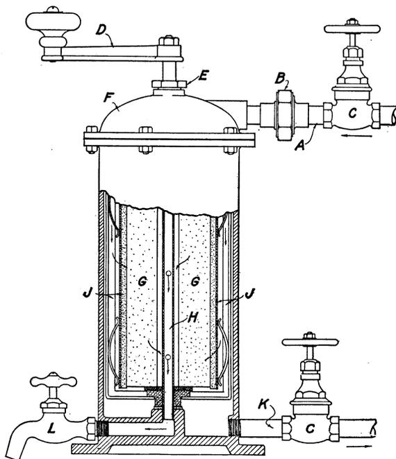
FIG. 9.—Stone pressure filter. *A*, Inlet pipe; *B*, union; *C*, gate valve; *D*, crank; *E*, stuffing box; *F*, removable top; *G*, filtering stone; *H*, center pipe; *J*, cleaning stone and holder; *K*, drain, used when cleaning the filter and flushing out; *L*, filtered water faucet.
