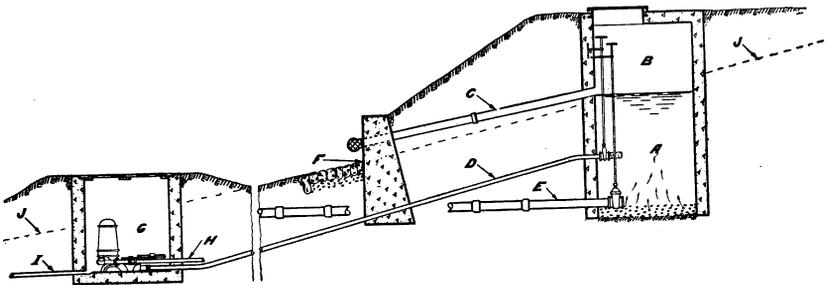
FIG. 34.—Hydraulic ram installation, Pennsylvania. *A*, Springs, yield about 5 gallons a minute; *B*, spring chamber; *C*, 4-inch screened overflow; *D*, 1½-inch drive pipe, 170 feet long, with gate, gate key, and screen; *E*, 4-inch drain pipe, with gate and key; *F*, retaining wall and pavement; *G*, ram; *H*, 1-inch delivery pipe; *I*, waste pipe; *J*, original surface of ground.
