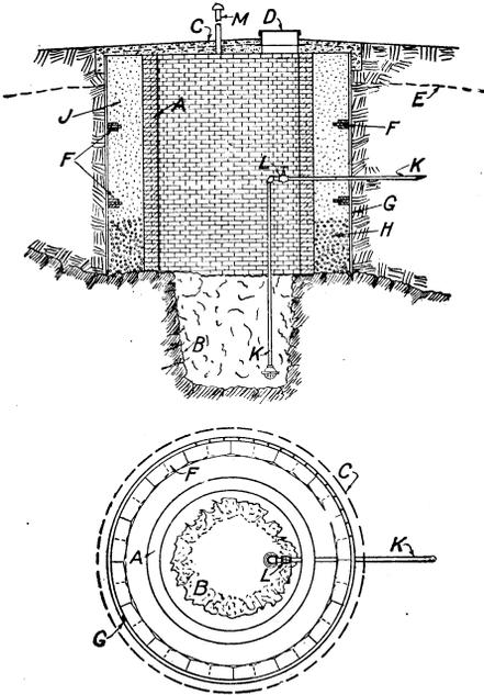
FIG. 17.—Large dug well in rock and caving earth. *A*, Masonry curb; *B*, rock excavation; *C*, platform; *D*, iron manhole frame and overhanging cover; *E*, original surface of ground; *F*, heavy wooden segmental ribs; *G*, heavy grooved sheet piling with hard pine splines or tongues greased before driving; *H*, clean gravel or stone filling; *J*, clean sand filling; *K*, suction pipe; *L*, gate valve; *M*, screened ventilator.
