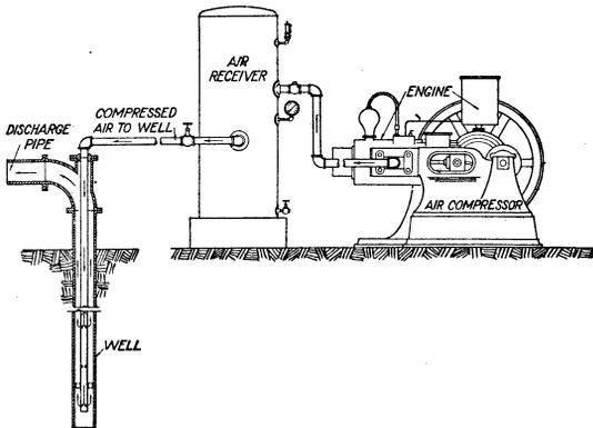
FIG. 38.—Air-lift installation.
