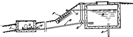
FIG. 33.—Hydraulic ram installation, St. Marys County, Md. *A*, 1½-inch well flowing 4 gallons a minute; *B*, concrete supply tank; *C*, screened overflow; *D*, 1½-inch drive pipe; *E*, gate valve; *F*, paved slope; *G*, ram; *H*, ¾-inch delivery pipe to storage tank; *I*, wasteway.
