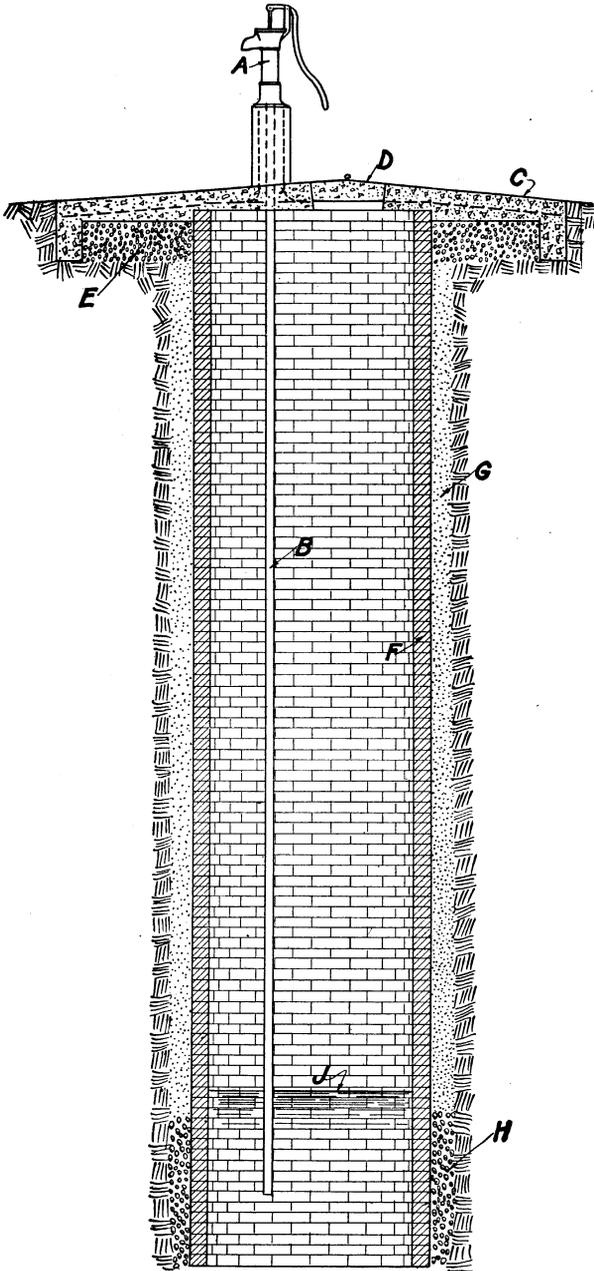
FIG. 14.—Well 23 feet deep in clay soil dug in 1915, Prince Georges County, Md. Manhole and cover shaped by using a large dish pan. Total cost \$53.18, and includes pump, 1,800 brick, and purchase of the pail, rope, pick and shovel used in excavating. *A*, Pitcher pump on concrete base 9 inches square and 18 inches high; *B*, 1 $\frac{1}{4}$ -inch suction pipe; *C*, platform; *D*, manhole; *E*, gravel foundation; *F*, brick curb; *G*, clean sand; *H*, clean gravel; *J*, water level.
