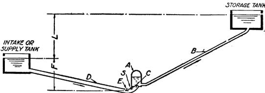
FIG. 30.—General layout of a hydraulic ram installation. *D*, Drive, feed, or supply pipe; *E*, escape, waste, impetus, dash, or clack valve; *C*, check, delivery, or discharge valve; *A*, air chamber; *B*, delivery or discharge pipe; *S*, sniff or air valve; *F*, fall, supply head, or power head; *L*, lift, discharge head, or pumping head.
