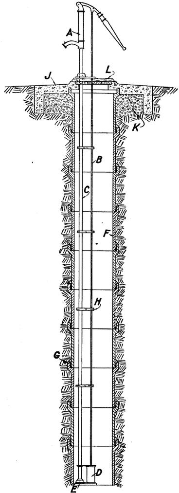
FIG. 16.—Dug well curbed with vitrified socket pipe. *A*, Pump stand; *B*, pump rod; *C*, riser pipe; *D*, cylinder; *E*, check valve; *F*, vitrified socket pipe; *G*, joints packed with a strand of oakum dipped in grout and filled with cement mortar; *H*, pump rod guides; *J*, platform; *K*, gravel foundation; *L*, cross-planked cover.
