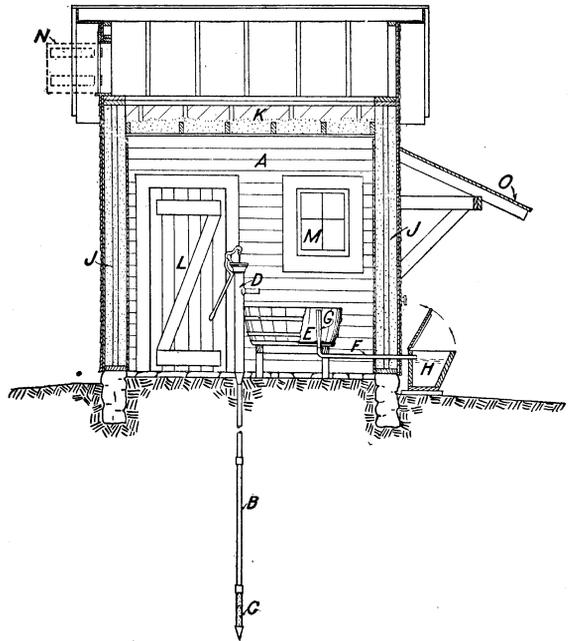
FIG. 27.—Driven well in a milk house. *A*, Milk house, sectional view, showing interior; *B*, drive pipe; *C*, well point; *D*, copper pump; *E*, cooling tub; *F*, lead waste pipe; *G*, wooden plug; *H*, watering trough; *J*, hollow walls, 10-inch space filled with dry sawdust; *L*-*M*, double doors and windows on north side; *N*, door in gable to facilitate placing sawdust; *O*, shed.
