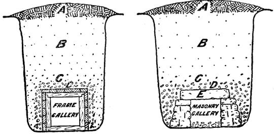
FIG. 29.—Infiltration galleries. *A*, Earth refill; *B*, sand and gravel; *C*, 6-inch layer of screened gravel  $\frac{1}{8}$  to  $\frac{1}{2}$  inch in size; *D*, 6-inch layer of screened gravel,  $\frac{1}{2}$  to  $1\frac{1}{4}$  inch size; *E*, covering stone. The frame gallery has been used constantly 27 years. Always submerged, the wood is preserved fairly well, but silt and quicksand gradually are filling up the gallery.
