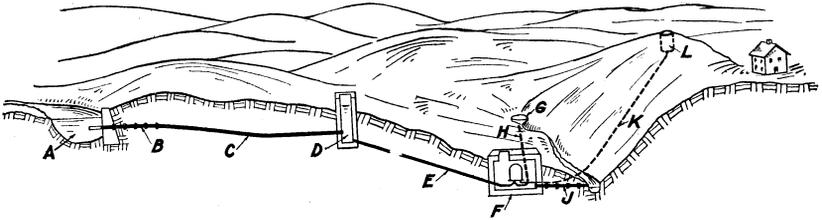
FIG. 32.—Method of using a distant surface supply to raise clear spring water. *A*, Surface supply; *B*, supply pipe (may be vitrified pipe for a portion of the way, where the pressure is small); *C*, iron supply pipe; *D*, standpipe; *E*, drive pipe; *F*, ram; *G*, spring; *H*, spring-water supply pipe; *J*, waste pipe; *K*, delivery pipe; *L*, elevated reservoir.
