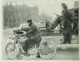
HARLEY-DAVIDSON MOTORCYCLE EQUIPPED WITH FOUR PYRENE CHEMICAL FIRE EXTINGUISHERS. ABLE TO DODGE THRU CONGESTED TRAFFIC AHEAD OF BIGGER APPARATUS AND ARRIVE IN TIME TO CHECK BLAZE WHILE IT IS STILL IN ITS INCIPENCY.
