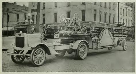
HORSE-DRAWN AERIAL TRUCK. MOTORIZED WITH A 31/2-TON GRAMM-BERNSTEIN TRACTOR. OPERATED BY THE CITY OF LIMA, O.
