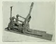
A DEVICE FOR PUSHING PIPE UNDER PAVING.
