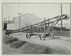
PORTABLE LOADING AND CONVEYING MACHINE
