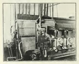
BLUE PRINT MACHINE showing controlling switches and gearing for washer.
