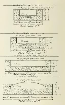
B Y REFERENCE to Fig. 1 it will be seen that the first two of these sections are of the covered gutter under the sidewalk on the lower right-hand corner, and show the differences in dimensions to suit the differences in volume of water to be carried. The first section and the third show the some for the covered gutter under the upper right-hand corner, and the fourth for that under the street pavement.
