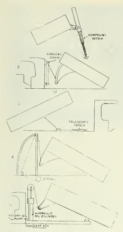
T IPPING GEAR for various American motor trucks; (1) Peerless, (2) Mack, (3) Locomobile, (4) Alco, (5) Pierce-Arrow.
