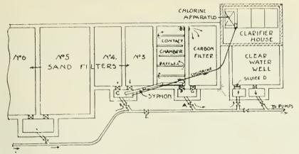
**P** LAN of emergency dechlorinating plant. Sand filter No. ? was taken for the contact chamber of the chlorinating apparatus and filter No. 1 was taken for the carbon filter to remove the taste and odor from the water due to the use of enough hypochlorite to insure destruction of bacteria.
