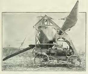
The gasoline engine on the Austin Special Street Paving Machine will propel it backward or forward and will travel over ordinary roads at the rate of about two miles an hour. The chute through which the concrete is distributed is ten feet long and can be reduced to seven feet, and from seven to five feet without stopping the machine.
