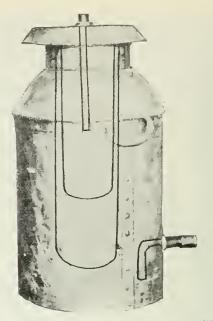
DUST COLLECTOR made from a milk can, which is very effective and inexpensive.
