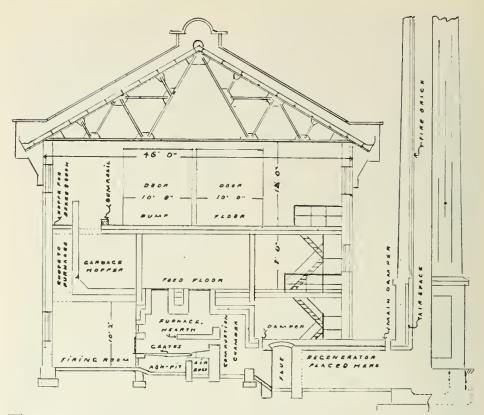
T HIS SECTION of a Wylie garbage destruction plant shows clearly its construction and method of operation.
