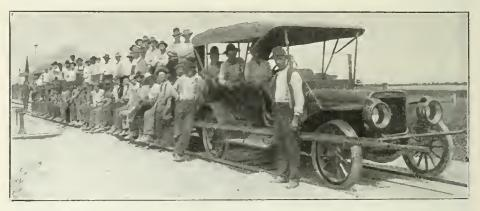
AUTOMOBILE used as a locomotive, steel wheels, turntable always at hand.
