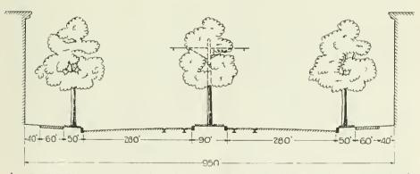
A DESIGN for a cross-section of a street with a double line of street car tracks which alternates trolley poles and trees in the wide space between tracks. Small trees give little trouble, but as they grow they must be trimmed carefully if not rendered unsightly.
