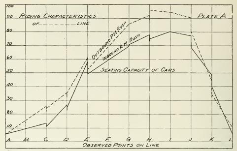
CURVE showing the variations in traffis at twelve different points on a street car line during the periods of heaviest travel in the morning and in the evening, indicating the points of maximum load and those where part of the service can be terminated. Note where the scating capacity is insufficient.
