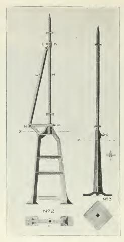
FOUNDATION POSTS for Van Dorn systen of iron fence construction.
