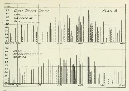
P LATE showing traffic at different moments during each of two afternoons. Each vertical line shows the number of passengers in the car passing the point of observation at the time shown at the bottom of the line.
