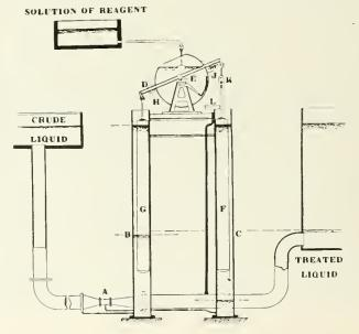
It is maintained that to insure accuracy and uniformity in the amount of reagent admitted, it is best to work with a solution of constant strength, and to adopt such a size of orifice as will give with the standard strength of solution the required amount of reagent. These elements having been once determined will be invariahle, and the apparatus will, therefore, work without further adjustment so long as the same percentage of solution is required to be added to the liquid.
