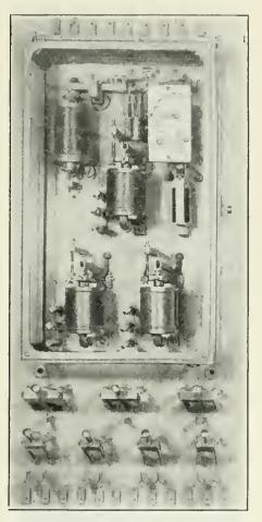
T IRRILL AUTOMATIC REGULATOR of voltage in bus-bars of feeder system.
