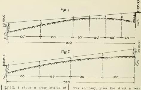
**H** IG. 1 shows a cross section of a street on a side hill which requires some guiter area on the upper side. Fig. 2 shows a side-hill street with all the water turned to the lower side. The water must be removed from the street by inlets to severs or drains at frequent intervals if either design is used.
