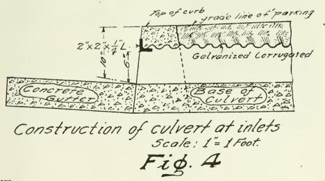
T HE CONSTRUCTION of the inlets to the culverts is shown of concrete, steel and gatvanized iron. The outlets are of the same design.
