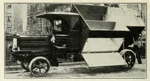
G ERMAN MOTOR TRUCK with four compartments for separating ashes and garbage, dumping on either side.
