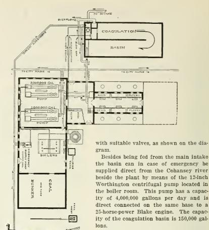
F IGURE 1 gives the plan of the pumping station, coagulation basin and filters, showing all the connections described in the article and the course of the water thru the plant.
