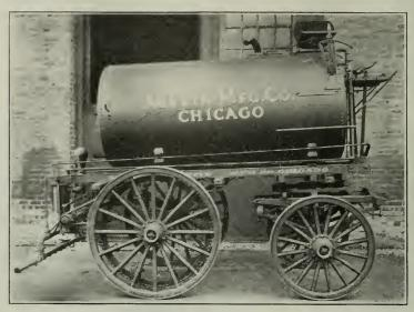
A NEW ROAD OILING MACHINE. Side View of Oiling Machine.
