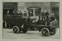
THE AUTOMOBILES OF SPRINGFIELD, Combination Hose and Chemical Car, 50-h.p., Gasoline Driven.
