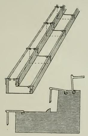
SMITH'S PLATES AND CLAMPS FOR ARTIFICIAL CURB AND GUTTER.
