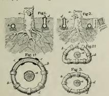
cality the best. This pipe, which may be of any suitable material, is perforated on the bottom, and is laid in a bed of gravel or slag. From one of the lengths of pipe a T extends to the surface, where it may be capped. The water or liquid fertilizer is introduced into this T and so reaches all sides of the tree.
