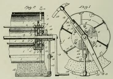
ADJUSTABLE CULVERT CENTERING. DETAIL DRAWING.
