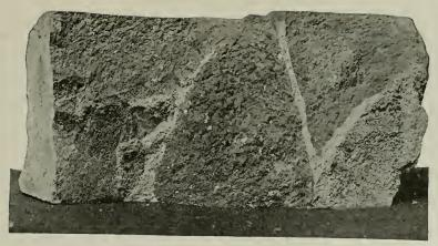
2. SHOWING STRENGTH OF BOND OF WIRE-CUT LUG BRICKS.
