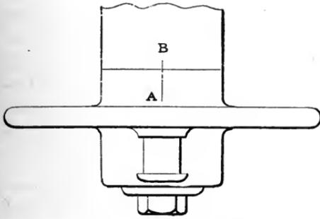
FIG. 57. — CENTRAL MARKS ON HUB OF WRIST PLATE.
