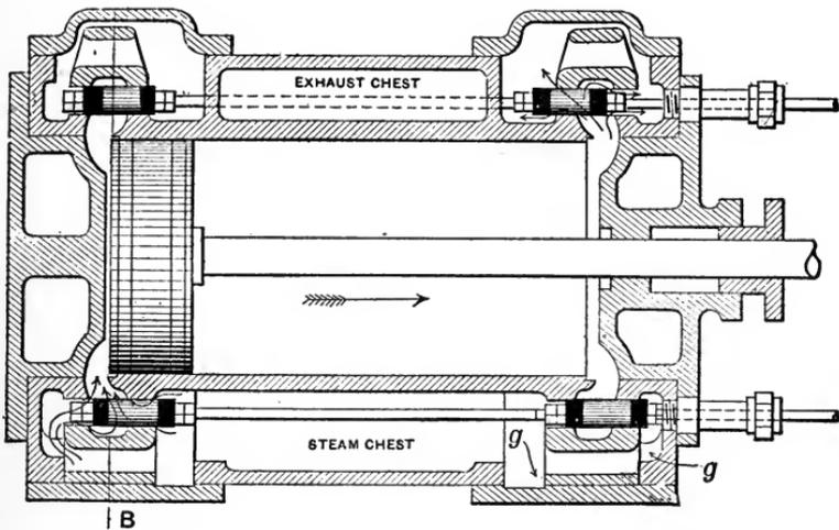
FIG. 108. — HORIZONTAL SECTION OF CYLINDER.
