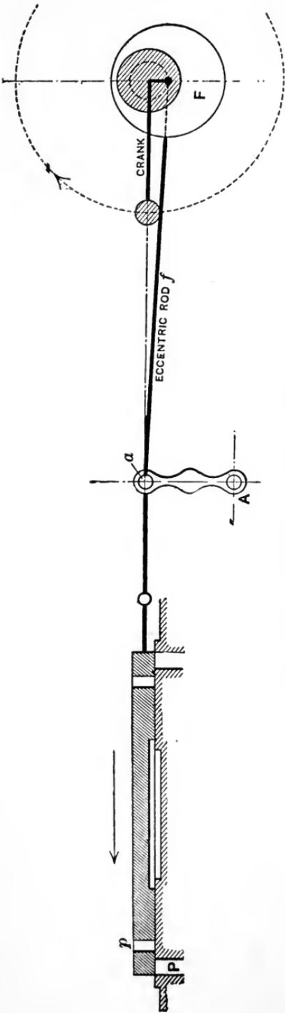
FIG. 104.— VALVE IN CENTRAL POSITION.
