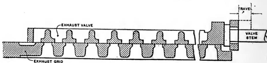
FIG. 90.—EXHAUST VALVE IN EXTREME INNER POSITION.
