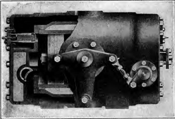
FIG. 196. — AIR CYLINDER WITH AUTOMATIC DISCHARGE.
