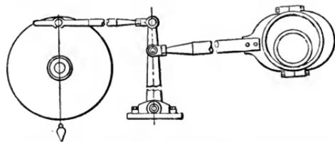
FIG. 56.—PLUMBING WRIST PLATE AND ROCKER ARM.
