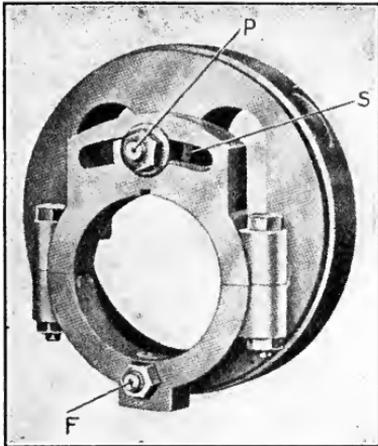
FIG. 143. — ADJUSTABLE LOW-PRESSURE ECCENTRIC.
