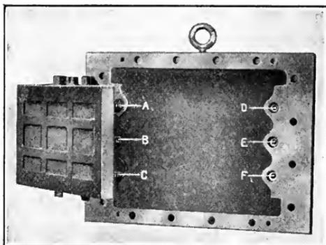
FIG. 140.—BACK PLATEN OF LOW-PRESSURE VALVE.
