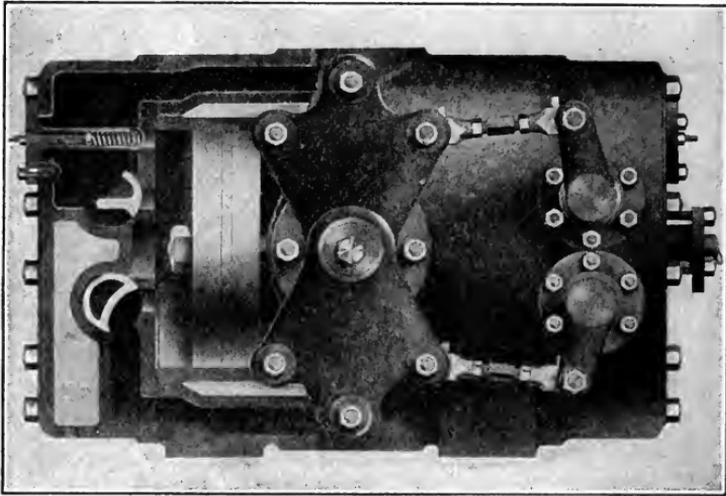
FIG. 198. — AIR CYLINDER WITH MECHANICAL DISCHARGE VALVE.
