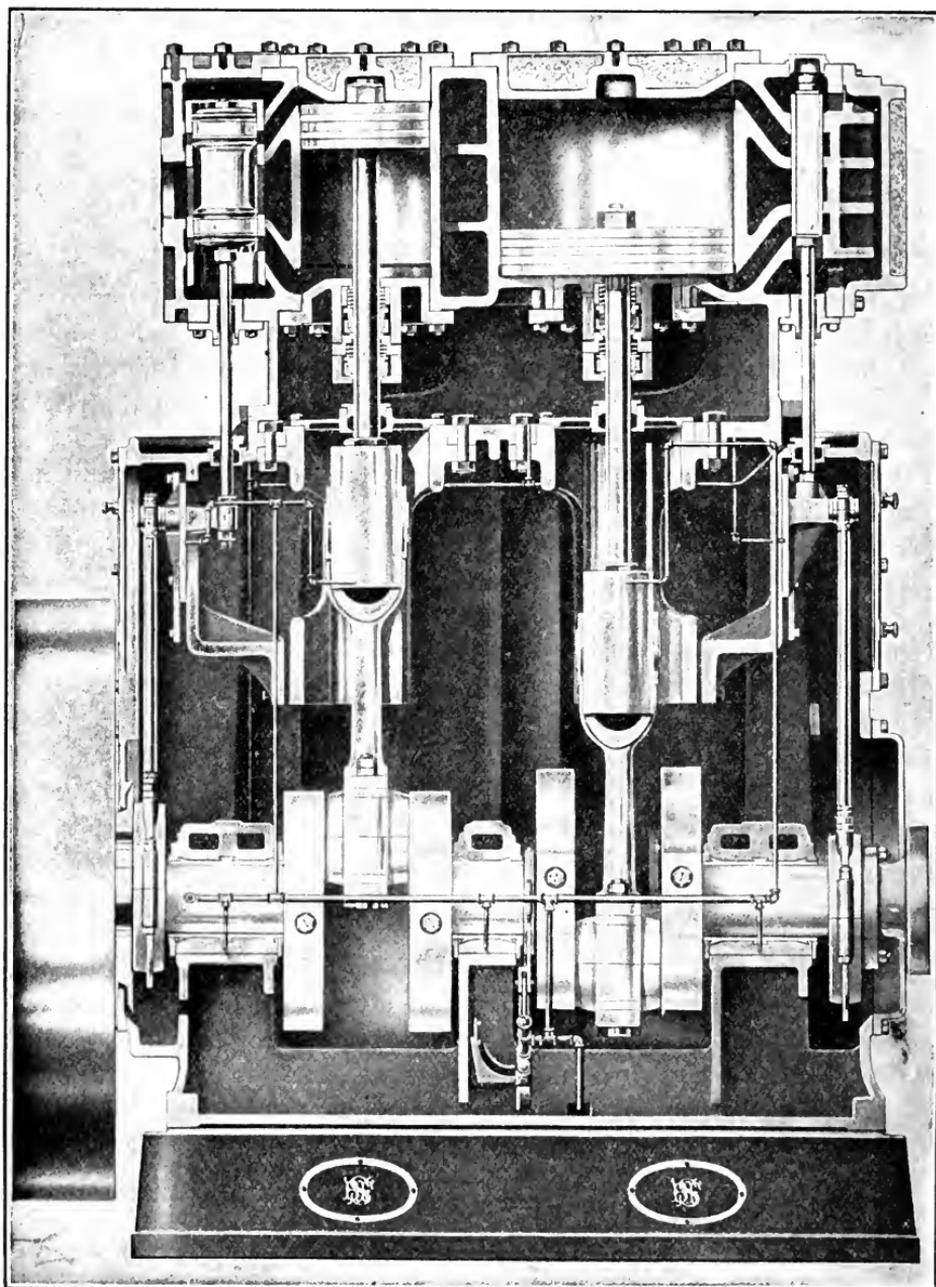
FIG. 139. — SECTION THROUGH CYLINDERS AND VALVES.
