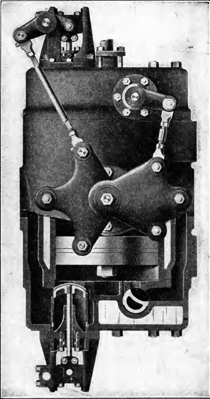
FIG. 197. — AIR CYLINDER WITH MECHANICAL DISCHARGE VALVE.
