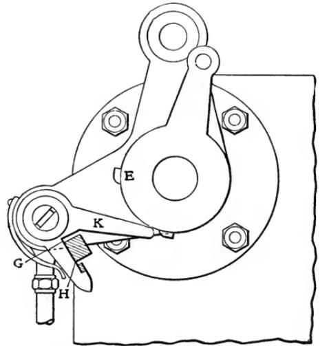
FIG. 60. — ADJUSTING CLEARANCE AT CATCH BLOCK.
