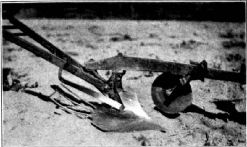
FIG. 7.—A good sweet potato digger. The rolling colter cuts the vines, and the rods projecting from the moldboard aid in freeing the potatoes from the soil and vines.
