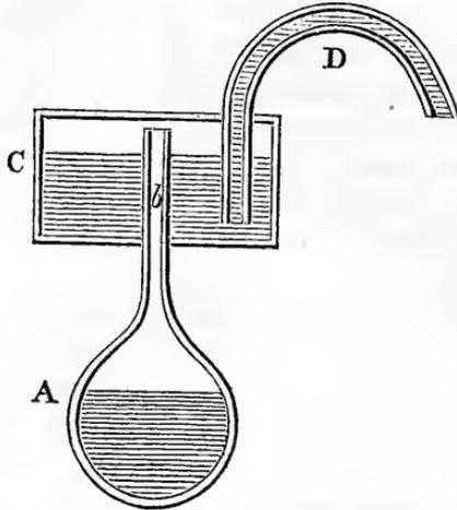
Water is boiled in a vessel A, placed upon a furnace. The steam rises through the pipe *b* into the upper part of the box or vessel C, the lower part of which is filled with water. The pressure of the steam on the surface of the water forces it up the rising pipe D.
