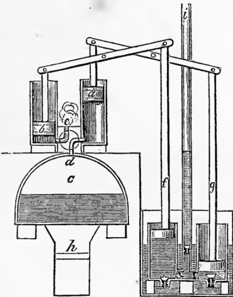
Steam is generated in the boiler *c*, and flows thence through the pipe *d*; it is represented as passing through one of the passages in a four-way cock, beneath the piston *a*, while the steam which had filled the other cylinder is escaping into the air through the passage *e*. The piston *a* works a lever and the pump-rod *g*, while *b* works another lever and the pump-rod *f*. *h* is the fire-place.
