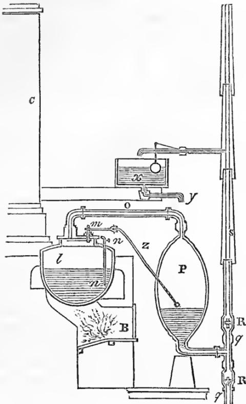
*l* is the boiler in which the steam is generated.
