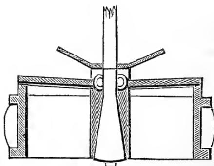
92. On the side of the Air-pump, and near its top, is cast a rectangular passage, which is closed by a valve *v*, similar in form and structure to the foot-valve, and which is called the Delivering-door or Clack-valve.
