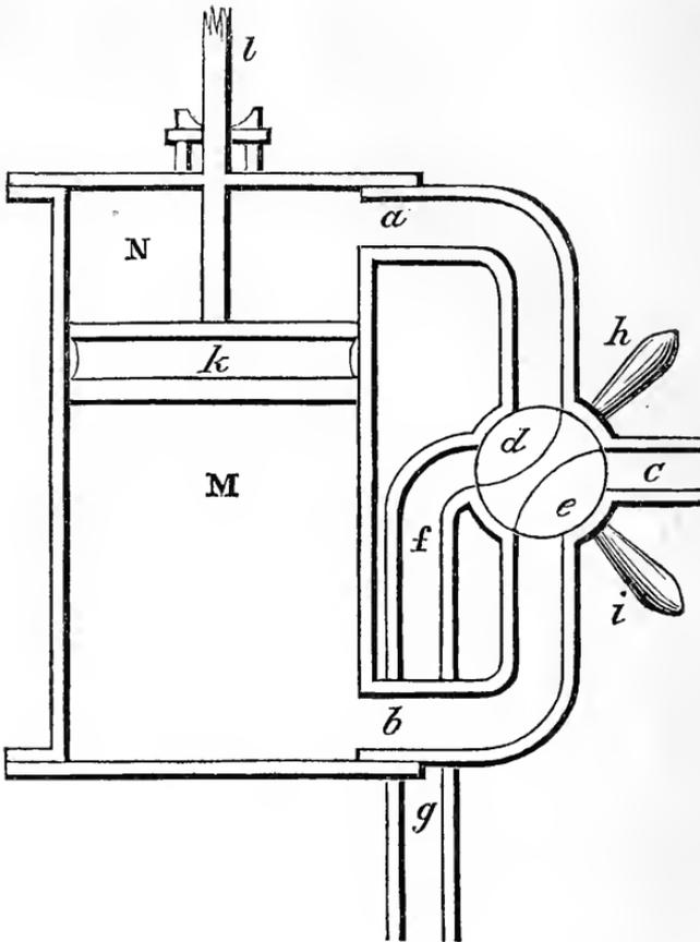
For this, in almost all high pressure engines, has been substituted a short slide valve, which has been found by experience to be more advantageous. This valve is worked by an Eccentric placed upon the axis of the crank; a convenient mode of doing this is represented upon *Pl. IV.* at *Fig. 3*, where,
