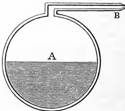
It is composed of a globe or other hollow vessel A, to which a pipe B, is adapted. If a portion of water be introduced, and the vessel placed over a fire, steam will be generated, and issue forcibly from the narrow aperture. If it be mounted on wheels, it will recoil by the reaction of the escaping vapour ; and a rotary motion may be produced, by two pipes, but in opposite directions, as in the machine of Hero.
