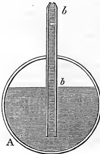
A spherical vessel *A* has a pipe *b b* inserted, until it nearly reaches its lower part. The vessel is partly filled with water, which is boiled, and the steam accumulating in the upper part, forces the water up the pipe. Here it will be observed that the heated water is itself raised, and the powers and utility of the engine are evidently far less than those of the machine of Porta.
