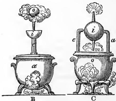
In the figure marked B, *a* is a vessel in which water is boiled; the pipe *c* proceeds nearly to its bottom; the steam will therefore accumulate in the upper part of the vessel, and force the water in a jet through the pipe *c*. A fountain may thus be formed, on which may be supported the ball *o*.
