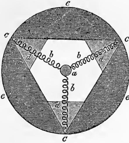
In applying a metallic piston, accuracy in the boring is absolutely essential, nor can they be introduced except when this part of the workmanship is of the best description.
