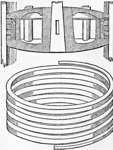
a screw-formed ring, compressed between the plates of the piston. The several convolutions of the screw are united by solder, until they are turned down to the proper dimensions. The solder is then melted off.
