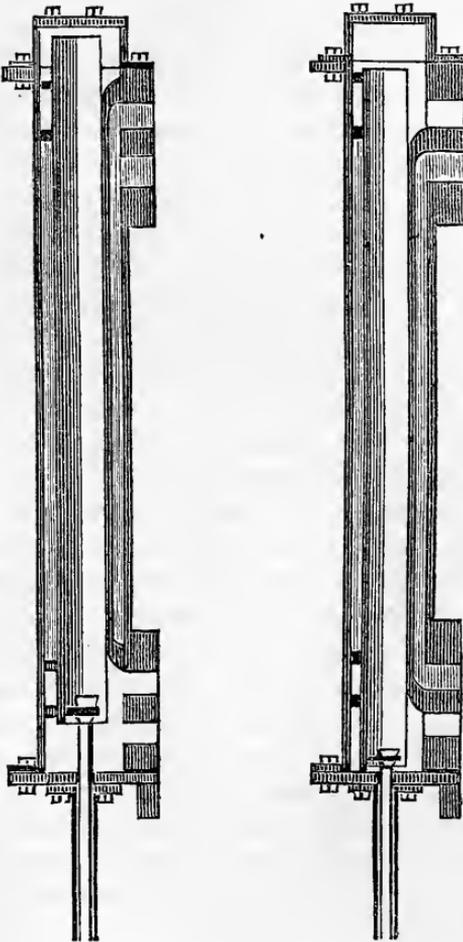
circular surfaces, where they come in contact, at the upper and lower extremities, must also be accurately fitted.
