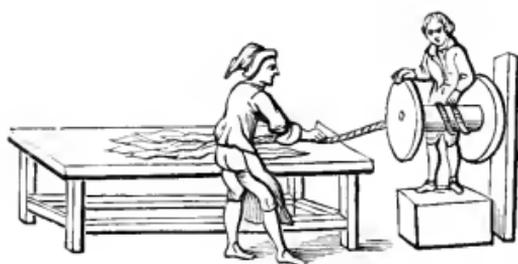
Sometimes this kind of tobacco was twisted in the manner of coarse cord, into a thick ball larger than a man's head, which formed a stock from which to "cut and come again."
