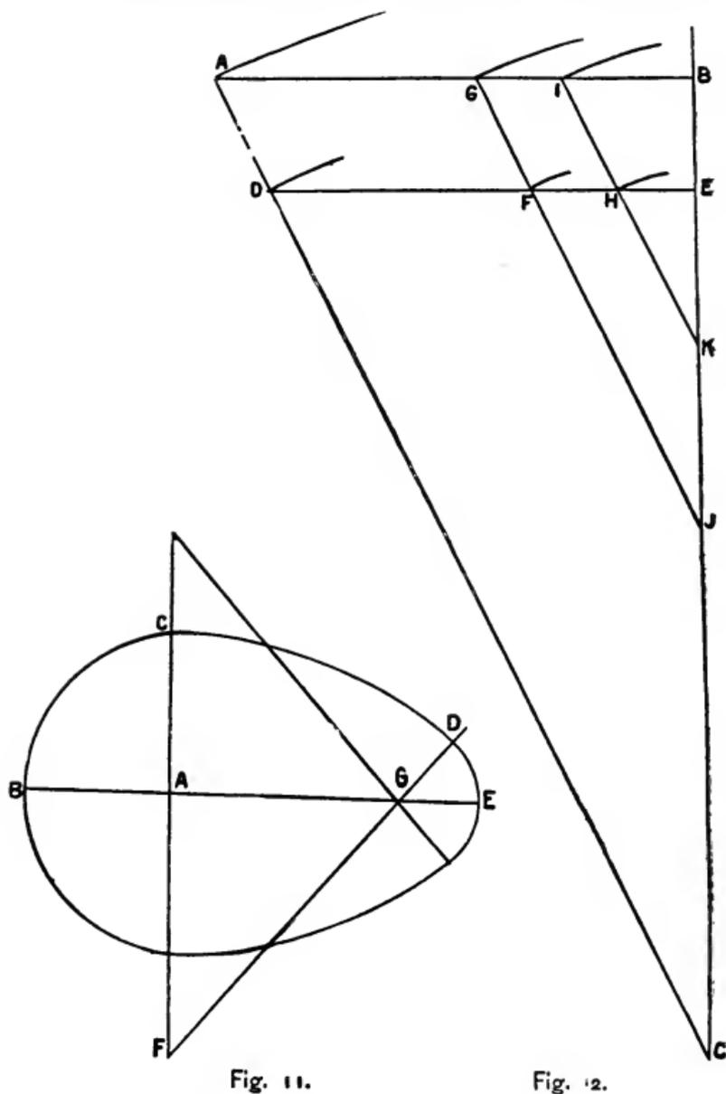
*in Two Sections.*—Describe the bottom, the length and breadth required as in Fig. 11, then describe the body as
