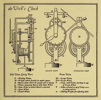
so called from a Latin word meaning "turning around." On this verge were fastened two flat projections called *pallets*, diverging from each other at about an angle of one hundred degrees. The width between the pallets, from center to center of each, was equal to the diameter of the wheel, so that one would mesh with the teeth at the top of the escape-wheel and the other with the teeth at the bottom.
