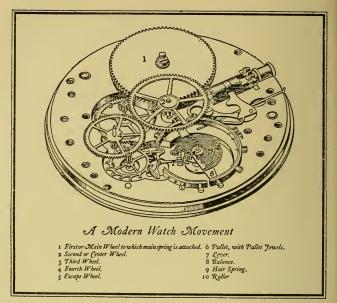
tooth before the other pallet-jewel is thrust in to stop it. It is a beautiful thing, to watch, like the beating of a tiny heart, or the breathing of a small quick creature. The hairspring (9) almost seems to be alive. And indeed, it is in a way, the very pulse of the machine.
