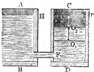
If the cross-section of the communicating pipe or orifice  $= F$ ; that of the vessel to be filled  $= G$  and initial difference of level  $O O_1$  of the two surfaces of water  $= h$ , we have, since in this case the level of the water in the second vessel rises with a uniformly retarded motion, the time required to fill it or the time in which the second surface of the water rises to the level  $H R$  of the first
