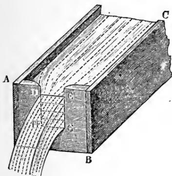
which the efflux takes place, is rectangular; let us denote its width  $D E = G H$  by  $b$  and its height  $D H = E G$  by  $h$ . If we decompose this surface  $b h$ , by horizontal lines, into a great number  $n$  of horizontal strips of equal width, we can consider the velocity to be constant for each of them. Since, if we proceed from above downwards, the heads of water of these strips are
