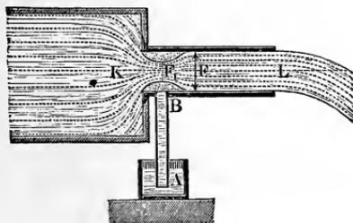
throwing small light bodies into the water. Upon so doing, we observe that near the entrance  $K$  there is a motion of translation in the middle of the cross-section  $F_1$ , but that, on the contrary, at the periphery of the same the water forms an eddy. It is, however, the capillarity or adhesion of
