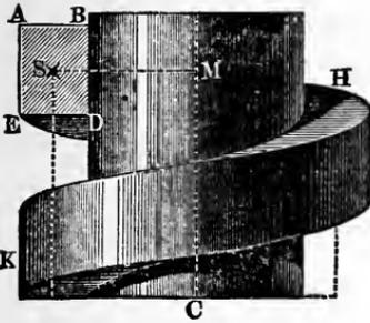
In many cases we can combine the use of the properties of Guldinus with that of Simpson's rule. E.G., to find the contents of the curved embankment  $A_0 D_0 B_1 D_2 A_2$ ,
