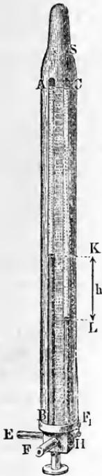
REMARK—1) Although Pitot's tube is not so accurate as the tachometer, yet, on account of its simplicity, it can be highly recommended. The author has discussed this instrument at length in the "Polytechnisches Centralblatt, 1847," and gives there a series of numbers, determined by experiment, and the values of the coefficient  $\psi$  deduced from them. With fine instruments, when the velocities were between 0,32 to 1,24 meters, we found  $v = 3,545 \sqrt{h}$  meters.
