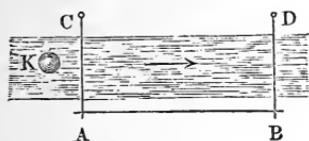
the other side of the river that the lines  $C A$  and  $D B$  shall be perpendicular to  $A B$ . Placing ourselves behind  $A$ , we note the instant the float  $K$ , which has been placed in the water some distance above, arrives at the line  $A C$ , and then passing be-
