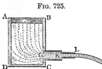
in Fig. 725, where the short tube  $KL$  is inserted into another short tube  $GK$ , and the latter into the vessel  $AC$ . Here, when the water enters the smaller from the larger tube, the stream is imperfectly contracted, and the coefficient of efflux is determined by the last rule. If we put the coefficient of resistance corresponding to this coefficient of efflux  $= \zeta_1$ ,
