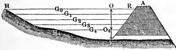
Fig. 789, we must employ some method of approximation, such as Simpson's Rule. If we divide the whole quantity of water into 4 equally thick layers and denote the heads corresponding to the different horizontal sections  $G_0, G_1, G_2, G_3, G_4$ , by  $h_0, h_1, h_2, h_3, h_4$ , we obtain, according to Simpson's Rule, the duration of the efflux
