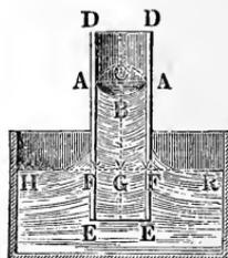
If we make the force, with which the wall of the tube attracts to itself the column of fluid  $B G$ , Fig. 651, proportional to the circumference of the tube, if, E.G., for a *cylindrical tube* we put this force  $P = \mu 2 \pi a$ , in which  $\mu$  denotes a coefficient, we have
