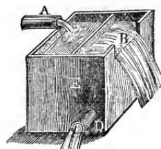
regulated by means of a lever and a float  $K$ , so that the same quantity of water is discharged through  $B$  as through  $F$ .
