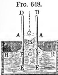
only on the outside, but also between them and the cross-section of its surface is nearly a semi-ellipse. One semi-axis of the elliptical cross-section is the half width  $C A = a$ , the other semi-axis  $C B = b$  is equal to the difference  $A F - B G = h_2 - h_1$  of the maximum and minimum elevations of the elliptical surface  $A B A$  above the general water level. According to the "Ingenieur," page 171, the radius of curvature of the ellipse at  $A$  is
