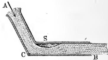
Fig. 754, is longer, an eddy  $S$  is formed beyond  $C$ , and, when the tube is again filled, the velocity of efflux  $v$  is smaller. This diminution of the velocity of efflux must be treated exactly in the same manner as the resistance produced by a contraction in the pipe. If  $F$  is the cross-section of the tube and  $F_1$  that of the contracted vein, we have the coefficient of contraction of the latter
