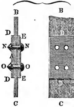
There are two modes in which bodies may be fastened together in this way; either the plates  $A B$  and  $C D$  to be joined together are laid upon one another, as in Fig. 330, and then fastened together by the bolts or rivets  $N N$  and  $O O$ , or, as is represented in Fig. 331, the plates are butted together and covered with splicing pieces  $D D$  and  $E E$ , and they are then fastened together by means of the rivets  $N N$  and  $O O$ ,
