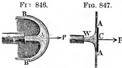
represented in Fig. 846, the water quits the surface in a direction opposite to that in which it struck it. In general the impact is greater against *concave* than against *convex* surfaces; for in the former case the angle is obtuse and its cosine negative
