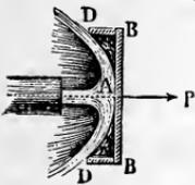
one inch thick and the cylindrical border 3 inches in diameter and  $3\frac{1}{2}$  lines high, the water flowed from the surface in nearly the opposite direction and the impulse was
