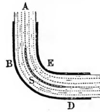
The resistance to water flowing through bends can be *diminished* by enlarging the cross-section of the pipe, as in  $B D E$ , Fig. 765, or by inserting in it a *thin partition*, like  $S$  in  $B D E$ , Fig. 766; for in the first case the velocity  $v$ , and in the second the ratio  $\frac{a}{r}$  is smaller, and consequently the coefficient of resistance  $\zeta$  is rendered less.
