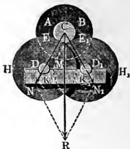
By the use of friction-wheels instead of plumber-blocks, the work done by the friction is diminished. In Fig. 270  $AB$  is a shaft, whose journal  $CE$  rests upon the circumferences  $EH$  and  $E_1H_1$  of the wheels (friction-wheels), which revolve around  $D$  and  $D_1$  and lie close behind one another. The given pressure  $R$  upon the shaft gives rise to the pressure
