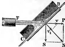
But if the impinged plane  $BC$ , Fig. 853, has a border upon two opposite sides only, the stream divides itself into two unequal parts, the angle of deviation  $a$  of the larger part  $Q_1$  is less than that  $180^\circ - a$  of the smaller part  $Q_2$ , and the total impulse in the direction of the stream is
