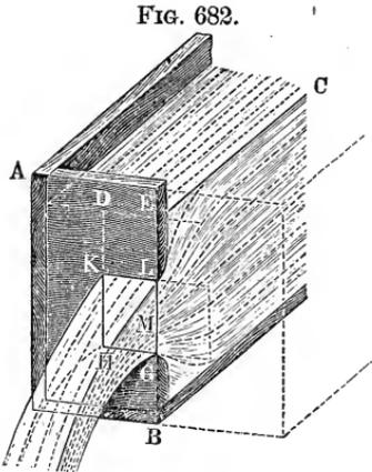
base  $G H$ , does not reach to the level of the water, we find the discharge through it by regarding it as the difference between two notches in the side  $D E G H$  and  $D E L K$ . If  $h_1$  is the depth  $E G$  of the lower and  $h_2 = E L$  that of the upper edge, we have for the discharges through these notches
