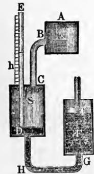
3) *Kopp's Volumeter*.—The pressure of the air enclosed in the space  $ABCD$ , Fig. 665, is the same as that of the exterior air, when the surface of the mercury  $DG$  touches the lower opening  $D$  of the manometer  $DE$ . If by means of a piston  $P$  we press the mercury into  $DG$ , until it rises to a certain height and its surface reaches the point
