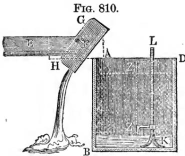
by means of which the water can be made to flow into the vessel or alongside of it. In order to determine accurately the depth of the body of water, we employ a scale *K L*. If, before we begin the measurement, we lower the pointer *Z* until it touches the surface of the water, which, perhaps, may only cover the bottom, and read off on the scale the depth of the
