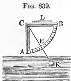
This instrument consists of a quadrant  $A B$ , Fig. 839, divided into degrees and parts of a degree, and of a string attached to its centre  $C$ , at the other end of which is fastened a metal or ivory ball  $K$ , 2 or 3 inches in diameter. The velocity of the water is given by the angle  $A C E$  formed by the stretched string with the vertical, when the plane of the instrument is placed in the direction of the stream, and the
