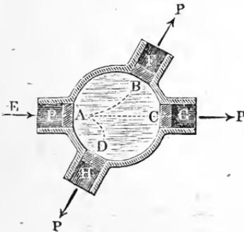
an apparatus filled with water, like the one whose horizontal cross-section is represented in Fig. 574. The tubes  $A, B, C, D$ , etc., which are of the same size and at the same distance above the base, are closed by pistons, which are easily movable and which fit the tubes perfectly; the water will then press upon each of them, by virtue of its weight, exactly as much as upon the others.
