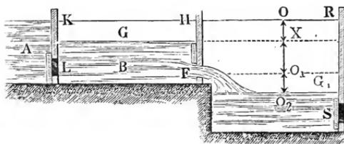
1) If we put the mean horizontal cross-section of the chamber of a single lock =  $G$ , the distance  $O O_1$  of the centre of the opening in the upper gate below the surface  $HR$  of the water in the head bay =  $h_1$ , its distance  $O_1 O_2$  above the water in the tail bay =  $h_2$  and the cross-section of the orifice in the gate =  $F$ , we have the time necessary to fill the lock to the middle of the orifice, during which the head is constant,
