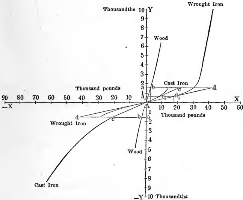
As next to iron *wood* (Fr. bois; Ger. Holz) is most generally employed in construction, the relations of the elasticity of fir, beach and oak wood are graphically represented in the figure by a curve. The average modulus of elasticity of these kinds of wood is
