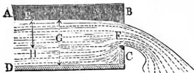
latter case, as there is no contraction upon the sides of the orifice, the discharge is greater than through orifices of the first kind. The author has made experiments upon these cases of efflux and deduced from the results obtained formulas, by means of which the coefficient of efflux can be calculated with sufficient accuracy, when the ratio  $n = \frac{F}{G}$  of the cross-sections is known.
