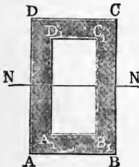
The moment of flexure of the *single-webbed girder*  $A B C D$ , Fig. 355, is determined in exactly the same manner.
