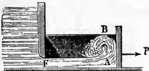
but a portion of the periphery; it limits, moreover, both the stream and the impinged surface. The impinging stream is turned in the direction of the portion of the periphery, which has no border, and is therefore deviated  $90^\circ$  from its original direction;
