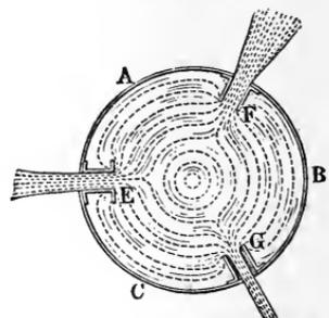
moves with different velocities in different parts of the cross-section, viz., upon the side  $C$  more quickly than upon the opposite one.
