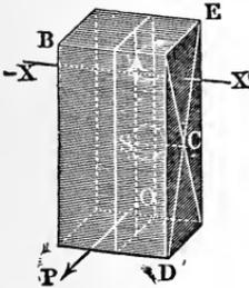
§ 344. **Ballistic Pendulum.**—The principles discussed in the preceding paragraphs are applicable to the theory of the ballistic pendulum of Robins (Fr. pendule ballistique; Ger. ballistische Pendel). It consists of a large mass  $M$ , Fig. 566, which is capable of
