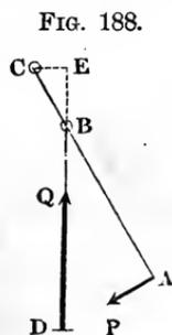
chinery. The knee lever  $A B C D$ , Fig. 188, which is sometimes cited as a peculiar sort of lever, is simply a bent lever. The arm, which is movable around an axis  $C$ , is acted upon by a force at its
