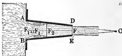
given by substituting for  $F_2$  the cross-section of the pipe, where the stream touches the wall. If  $\delta$  denotes the semi-angle of divergence *ACB* of one, or the semi-angle of convergence of the other tube, and if we assume that the length  $F_1 F_2$  of the eddy is equal to the width  $AB = d$  of the orifice, we have the width of pipe, where the stream reaches its wall,
