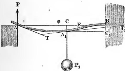
practice. If, for example, a girder  $AB$ , Fig. 345, is at one end imbedded in a wall and at the other merely supported, the question arises, what is the bending force at  $A$ , or what force has the support at  $A$  to bear, when the beam is loaded with a
