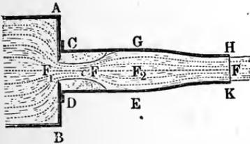
Let  $F$  denote the cross-section,  $v$  the velocity and  $p$  the pressure of the water at the outlet  $H K$ ,  $F_1$  the cross-section of the inlet,  $a F_1$  that of the contracted stream of water,  $v_1$  the velocity and  $p_1$  the pressure of the water in the latter; in like manner let  $F_2$  be the cross-section of the tube, where the stream of water again touches the wall,  $v_2$  the velocity and  $p_2$  the pressure of the water at that point. Then we have
