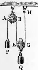
Let the weight of the pulleys  $A B$  and  $E G$  be  $= G$  and  $G_1$ , their moments of inertia  $G k^2$  and  $G_1 k_1^2$ , their radii  $C A = a$  and  $D E = a_1$  and their masses reduced to the circumference  $M = \frac{G}{g} \cdot \frac{k^2}{a^2}$  and  $M_1 = \frac{G_1}{g} \cdot \frac{k_1^2}{a_1^2}$ . If the weight  $P$  sinks a certain distance  $s$ ,  $Q + G_1$  rises  $\frac{1}{2} s$  (§ 164), the work done is therefore  $P s - (Q + G_1) \frac{s}{2}$ . Now if
