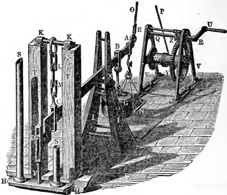
iron pillars give the necessary resistance to the bed-plate  $H H$ , through which  $F$  passes. The piece of iron  $L M$  to be experimented upon is suspended by means of a chain to the support  $K K$ , which reposes upon the two columns  $T T$  and is connected by a bolt and clevis to the stirrup  $C$  of the lever  $A C D$ . To the longer
