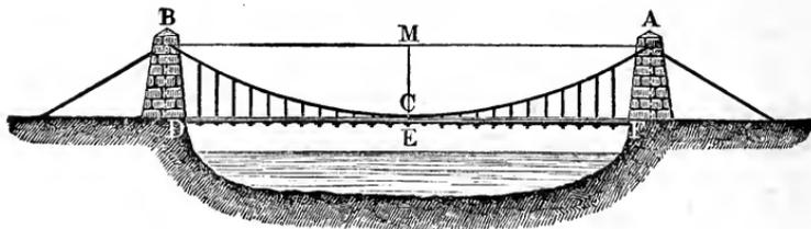
without weight or very light in proportion to that of the loaded bridge  $DEF$ , the latter weights alone would have to be considered, and the chain  $ACB$  would form a parabola.
