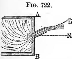
$K L$ , Fig. 722, with the normal  $K N$  to the plane  $A B$  of the orifice, and if  $\zeta$  denotes the coefficient of resistance for tubes cut off at right angles, we have for the coefficient of resistance of inclined tubes
