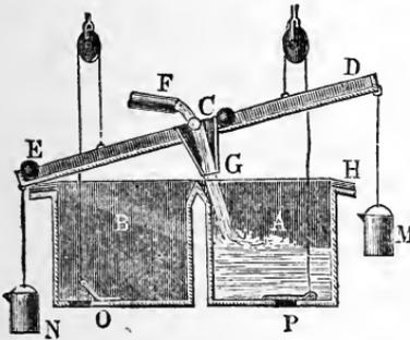
which is often met with in salt works. Here there are two measuring vessels  $A$  and  $B$ , which are alternately filled and emptied. The water, which is brought to them by the pipe  $F$ , passes through a short tube  $CG$ , which is rigidly connected with the lever  $DE$  which turns about  $C$ . If one of the vessels, as, e.g.,  $A$ , is filled, the water flows through a small trough  $H$  and fills the little bucket  $M$ , which then draws the lever down and the
