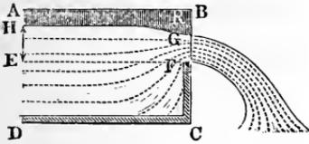
Fig. 701, the stream is contracted on three sides and a diminution of the discharge is produced. The discharge through this orifice is
