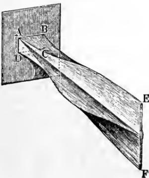
Bidone observed the discharge from various kinds of orifices; Poncelet and Lesbros have made the only accurate measurements of the stream issuing from square orifices (see the *Allgemeine Maschinenencyklopädie*, article "Ausfluss"). The last measurements have led to a small coefficient of contraction 0,563.
