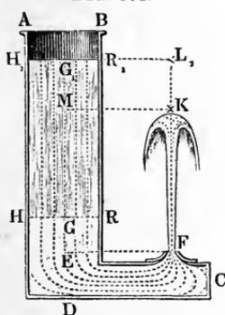
If above the level  $H R$  of the water  $H E R$  in a vessel  $A C D$ , Fig. 673, there is still a column of liquid  $H R_1$ , whose height  $G G_1 = h_1$  and whose heaviness  $= \gamma_1$ , while that of the water is  $= \gamma$ , we can replace the latter by a column of water whose
