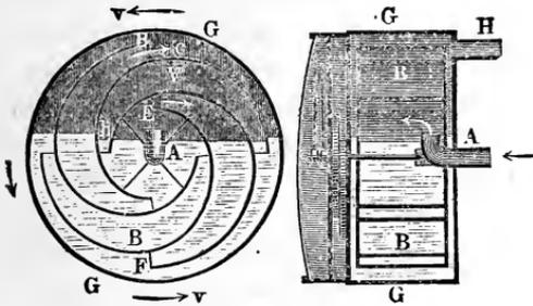
The gas, which arrives, enters by a bent pipe *A* into the interior of the measuring wheel *B B*, in which it depresses the surface of the water a certain distance *h*, which depends upon the tension of the gas passing through the instrument. From this
