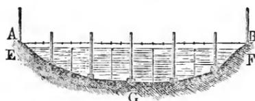
easily found for canals and small creeks  $E F G$ , Fig. 831, by stretching a measuring chain  $A B$  or laying a rod, etc., across the stream. When the river is wide, we make use of a plane-table  $M$ , placed at a proper distance  $A O$  from the cross-section  $E F$ , Fig. 832, to be measured. If  $a o$  upon the plane-table is the reduced distance  $A O$
