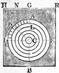
of approximate formulas obtained in the following manner. Let us decompose the circular orifice by concentric circles into small rings of equal width and let us consider each ring to be composed of elements, which may be regarded as parallelograms. If  $r$  is the radius,  $b$  the width and  $n$  the number of elements of one of these rings,  $\frac{2 \pi r}{n}$  is the length of one of these elements
