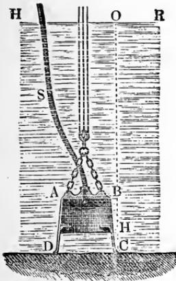
at the beginning the bell with its opening  $C D$  stands above the level of the water  $H R$ , so that the whole space  $V$  is filled with air at a pressure equal to that of a column of water, whose height is  $= b$ . If afterwards the bell sinks to a depth  $O C = x$  and a volume  $W$  of water is thus introduced into it, the volume of the inclosed air, when none is pressed back through the hose, becomes  $V - W$  and the height of the water barometer becomes  $b + x - y$ ; hence
