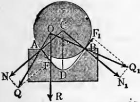
If the bearing  $A D B$ , Fig. 274, is triangular, the axle is supported at two points  $A$  and  $B$  and at both of them friction must be overcome. The resulting pressure  $R$  is decomposed into two components  $Q$  and  $Q_1$ , each of which is again decomposed into a normal stress  $N$  or  $N_1$  and into a tangential one, which
