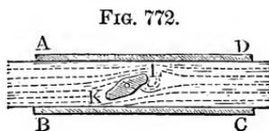
sections of the maximum contractions have very peculiar forms. The stream is divided by the *throttle-valve* (or disc and pivot valve), Fig. 772, into two parts, each of which passes through a contracted orifice. The cross-sections of the contracted openings are rectangular in parallelepipedical pipes and crescent-shaped in cylindrical ones. The following examples will sufficiently explain the use of the foregoing tables.
