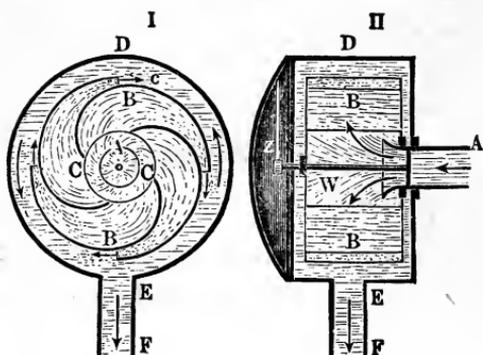
and passes through 4 canals *C B, C B . . .* to the exterior circumference, where it is discharged into the case *D E*, from which it is conveyed away by a tube *E F*. The shaft *W* of this wheel carries a pointer *Z*, or rather a train of wheel-work, which indicates the number of revolutions of the wheel, and by it the volume of the water,
