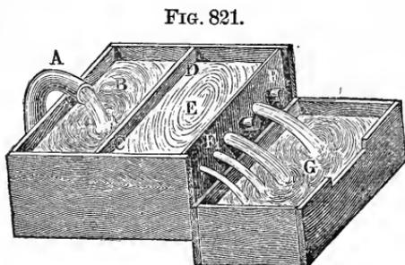
The water to be measured is discharged from the pipe *A* into a box *B*, from which it passes through holes, made in the partition *C D* below the level of the water, into the box *E*; from it the water is discharged through circular orifices *F* one inch in diameter, which are cut out of sheet iron, into the
