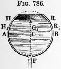
1) The time required to empty a *segment of a sphere*  $A F B$ , Fig. 786, which is filled with water, whose radius  $C A = C F = r$  and whose height  $F G = h$ , is
