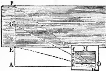
the corresponding points from the shore; for the engineer, who is at the plane-table, can sight at the sounding-rod, when it is placed in the line  $E F$ .
