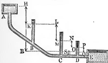
the conduit, friction, etc., can be measured by means of the columns of water maintained in the vertical tubes *B K*, *C M*, *D O* which are attached to the pipe; when they serve for this purpose only, they are called *piezometers* (see § 386).
