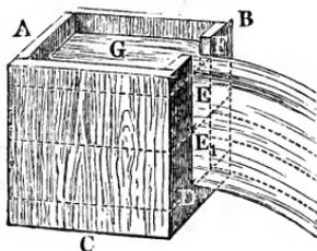
782, into which there is no water discharged, the duration of the efflux is found in the following manner. Let us denote the cross-section of the vessel by  $G$ , the width  $E F$  of the notch by  $b$ , and the height  $D E$  by  $h$ , and let us divide the whole orifice of efflux into small strips, the length of each being
