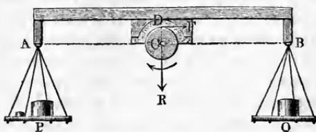
which he called a friction balance (Fr. balance de frottement, Ger. Reibungswage). Here  $C$  is an axle, which is kept in constant rotation, as, E.G., by a water-wheel,  $D$  is the bearing, and  $A D B$  is a lever of equal arms, which produces the pressure between the journal and its bearing by means of the weights  $P$  and  $Q$ . The pressure on the axle  $R = P + Q$  produces the friction
