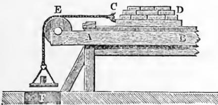
weight necessary to bring the sled from a state of rest into motion, and the coefficients of friction of motion were determined by aid of the time required by the sled to describe a certain space  $s$ . If  $G$  is the weight of the sled and
