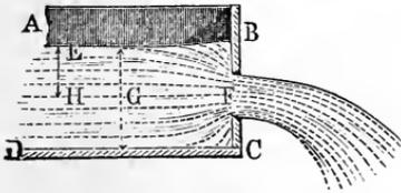
In the experiments made by the author with Poncelet's orifices the head of water was measured 1 meter back from the plane of the orifice; they gave
