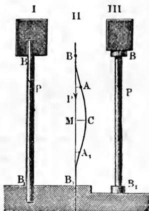
I. and III., the ends of the pillar are rounded or when they are movable around bolts. An example of the latter case is the *connecting rod* of a steam engine.
