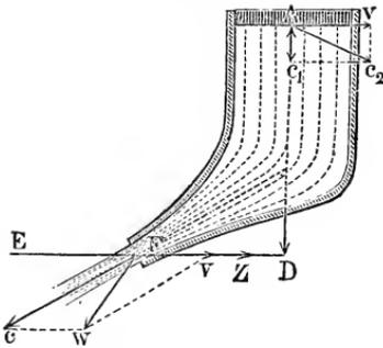
has an opening  $F$ , through which the water issues, this force undergoes a change not only because a portion of the wall of the vessel is absent, but also because the water, which issues from the orifice, like every other body, which changes its conditions of motion, reacts by virtue of its inertia. The change in the motion of a body may consist either of a change of velocity, or of a change of direction, and, therefore,
