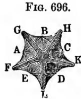
orifice  $A B C D E$ , Fig. 696, is a five-pointed star  $E G H K L$ , etc. The cross-sections are very different at different distances from the orifice; they decrease for a certain distance and then increase again, etc.; the stream consists, therefore, of ribs of variable width and forms, as can be best observed when the pressure is very great, bulges and nodes similar in form to the cactus plant. If the orifice  $A B C D$ , Fig. 697, is *rectangular*, the cross-section at a small
