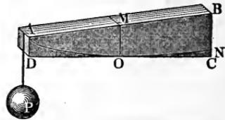
Instead of the parabolic girders, Fig. 405, we generally make use of girders, Fig. 409, with plane surfaces. In order to economize as much material as possible the girder is made in the middle *M* of the same height  $M O = h_m = h \sqrt{\frac{1}{2}}$ , as the parabolic girder would have been, and the limiting plane surface *C D* is made tangent to the corresponding parabolic surface. We have
