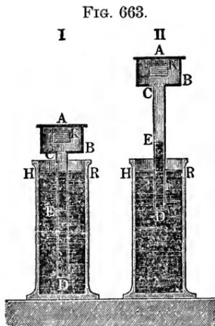
Now if  $V_0$  is the volume of the space  $AB$ ,  $V_1$  the required volume of the body  $K$ , which is placed in it,  $V$  the volume of the column of air  $CE$ ,  $b$  the height of the barometer and  $h$  that of the column of mercury  $DE$ , we have, according to Mariotte’s law, since the same quantity of air occupies the volume  $V_0 - V_1$ , when the tension is  $b$ , and the volume  $V_0 - V_1 + V$ , when the tension is  $b - h$ ,
