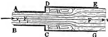
the aid of Borda's formula we can calculate the various relations of the pressure in a discharge pipe, the diameter of which is not constant. Let  $p_1$  be the pressure and  $v_1$  the ve-
