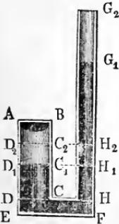
if we then compress it by pouring in quicksilver, until it occupies one-half, one-quarter, etc., of its original volume, we will find that heights  $G_1 H_1$ ,  $G_2 H_2$ , etc., of the surface of the mercury in the tube are equal to the height of the barometer  $b$  multiplied by one, three, etc. Consequently, if we add the height corresponding to the pressure of the atmosphere, we find that the tension is double, quadruple, etc., that of the original volume.
