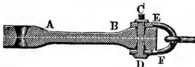
*experimenting upon rupture by extension* we employ bodies with large heads *A* and *B*, Fig. 320, through which holes are bored exactly in the axis. In the middle of each hole a circular
