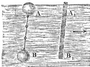
The two balls are united by a string, wire or thin wire chain. We first determine by a single ball the superficial velocity  $c_0$ , and we then determine the mean velocity  $c$  of the two connected balls; now if we denote the velocity at the depth of the second ball by  $c_1$ , we can put
