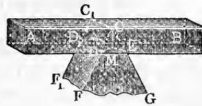
The amount of friction of a beam  $A B$ , Fig. 288, oscillating on a knife-edge  $C C_1$ , can be found in like manner. If  $a$  is the half angle of convergence  $D C M$ ,  $l$  the length  $C C_1$  of the edge and  $R$  the pressure, we have
