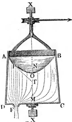
If the vessel, from which the water flows, is moved horizontally or at an acute angle to the horizon, the surface (see § 354) becomes oblique to the horizon and a variation of the velocity of efflux is the result.
