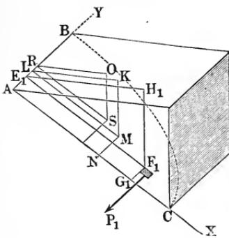
E.G., if the other circumstances are the same, a wall  $ABCD$ , Fig. 596, has to resist the same pressure whether it dams up the water of a small trough  $ACEF$  or that of a large dam  $ACGH$  or that of a lake. From the width  $AB = CD = b$  and the height  $AD = BC = a$  of the rectangular wall we obtain the surface of the same
