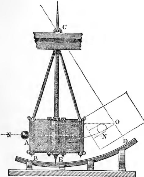
turning around a horizontal axis  $C$ . It is set in oscillation by means of a cannon-ball, which is shot against it, and serves to determine its velocity. In order to render the impact as inelastic as possible, upon the side where the ball strikes, a large cavity is made, which from time to time is filled with fresh wood or clay, etc. The ball remains, therefore, after every shot, sticking in this mass, and oscillates together with the whole body. In order to determine the velocity
