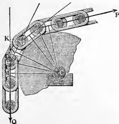
against the links, since the former are turned through a certain angle in their bearings. If  $A B$ , Fig. 297, is a link of the chain and  $B G$  the following one, if  $C$  is the axis of rotation of the pulley, upon which the chain, stretched by the weight  $Q$ , winds, and if finally  $C M$  and  $C N$  are perpendiculars let fall upon the major axis of the links  $A B$  and  $B G$ , then  $M C N = \alpha^\circ$  is the angle
