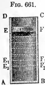
While the piston describes a very small portion  $E_1 E_2 = \sigma$  of the space, the tension  $p_1$  can be regarded as constant, and the work done is =  $F p_1 \sigma = \frac{F p s \sigma}{s_1}$ ,  $F$  denoting the area of the piston.
