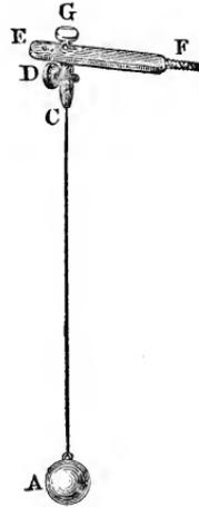
whose upper end is fastened into a ferrule  $D$  by a clamping screw. This ferrule has upon its end a screw, which passes through the arm  $E F$  and is made fast by a nut  $G$ , when the arm has been screwed into a door-frame or some other solid support. If the length is  $C A = 0,2485$  or nearly  $\frac{1}{4}$  meter, then this pendulum will beat half-seconds for almost an hour, although the arcs in which it oscillates will continually decrease.
