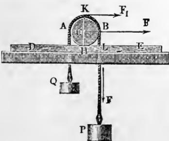
a few experiments with rollers of lignum-vitæ and elm from 2 to 10 inches thick, which were rolled upon supports of oak by winding a thin string around the roller and attaching to the ends of it the unequal weights  $P$  and  $Q$ , Fig. 289. According to the results of these experiments, the rolling friction is directly proportional to the pressure and inversely to the radius of the
