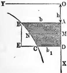
$\frac{a}{n}$  from each other will divide this orifice into strips of equal height, and the discharge  $\frac{Q}{n}$  through each of them should be the same. For the upper strip, whose width is  $b$  and for which the head is  $h$ , we have
