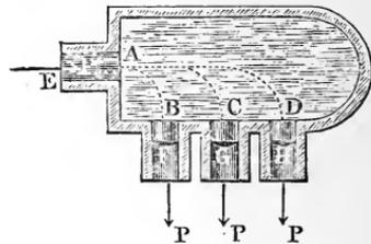
If the axes of the pipes  $B F, C G$ , etc., Fig. 576, are parallel to each other, the forces acting on the pistons can be combined so as to give a single resultant; if  $n$  is the number of the equally large pistons, the total pressure upon them will be
