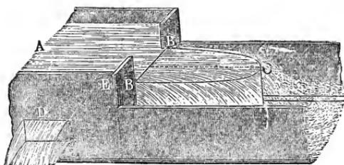
REMARK.—Such an apparatus for dividing the water was constructed of sheet iron for the *Wernergraben* at Freiberg by *Oberkunstmeister Schwamkrug*. It discharges through a rectangular orifice  $D$ , which is 5 feet long and 1 foot high, almost invariably 40 cubic feet of water per second, while the remaining water passes over the overfall, the sill of which lies 2 feet above the upper edge of the orifice, and flows on in the ditch to where it is wanted.
