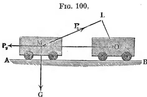
and is obliged to overcome a horizontal resistance  $P_2 = 450$  produced by the friction, what work must the force  $P_1$  do, in order to change the initial velocity of 2 feet of the wagon into a velocity of 5 feet?
