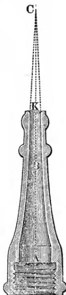
Hence  $l_1 = 51,54$  and  $l_2 = 20,46$  lines and the width at  $B$ , where the conical surfaces meet each other, is  $d_3 = d_2 + 2 l_1 \text{ tang. } \delta = 7 + 2 \cdot 51,54 \cdot 0,04362 = 11,53$  lines. Since this place is rounded off, we can put  $d_3 = 13$  lines; hence for the outlet piece
