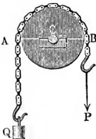
round a roller  $ACB$ , Fig. 298, when the weight acting vertically is  $Q = 110$  pounds, the weight of the roller and chain is 50 pounds, the radius  $a$  of the roller, measured to the middle of the chain, is  $a = 7$  inches, the radius of the axle  $C$  is  $= \frac{5}{8}$  of an inch and that of the bolts of the chain is  $= \frac{3}{8}$  of an inch? If we put  $\phi = 0,075$  and  $\phi_1 = 0,15$ , we obtain, according to the last formula, the force
