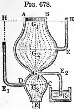
If from the cross-section  $G_2$  we carry a tube  $E R$  upwards the latter will fill with water, which will rise above the level  $H R$  of the water, when  $G_2 > G_1$  or  $v_2 < v_1$ ; for, since the pressure  $p_1$  upon the surface of the water is balanced by the pressure of the air upon the mouth of the tube, we can put the height, which measures the pressure in  $G_2$ ,
