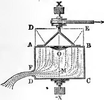
EXAMPLE—1) If the vessel  $AC$ , Fig. 689, which when filled with water weighs 350 pounds, is drawn upwards by a weight  $G$  of 450 pounds by means of a cord passing over a pulley, it rises with an acceleration
