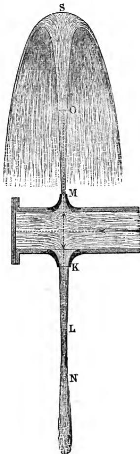
remains continuous and is not broken up by the air, its cross-section  $L$  decreases more and more as the distance  $K L = x$  from the orifice increases. If  $c$  is the velocity of efflux and  $v$  the velocity at  $L$ , we have
