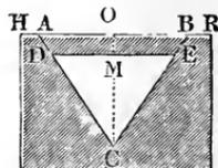
Further, the discharge through a triangle  $C D E$ , Fig. 685, whose base is  $D E = b_1$ , whose altitude is  $O M = h_1$  and whose apex  $C$  is situated at a depth  $O C = h$  below the level  $H R$  of the water, is  $Q =$  discharge through  $A B C$  minus that through  $A E$
