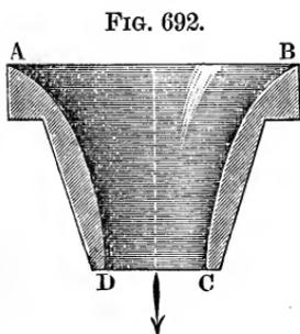
under a pressure of 10 feet 98 per cent., under a pressure of 5 feet 97 per cent., and under a pressure of 1 foot 96 per cent. of the discharge calculated theoretically (Experiments with large orifices, see *Untersuchungen in dem Gebiete der Mechanik und Hydraulik, Zweite Abtheil.*). If the efflux through such a mouth-piece is to be as free from disturbance as possible, the rounding must not be in the form of a circle, but in that of a curve  $A D = B C$ ,
