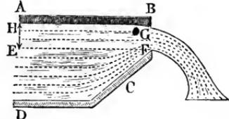
slope of one-half to one. For the overfall, represented in Fig. 707, where, as in Poncelet's sluice, contraction takes place upon one side only, the author found  $\mu = 0,70$  or  $\mu_1 = \frac{2}{3} \mu = 0,467$  for an inclination of  $45^\circ$ , and  $\mu = 0,67$  or  $\mu_1 = 0,447$  for an inclination of  $63\frac{1}{2}$  degrees.
