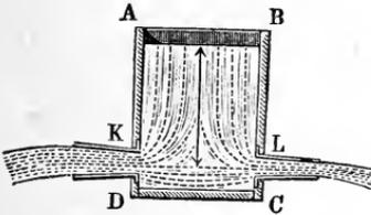
outlet orifice is smaller than the inlet, and in the second case the inlet is smaller than the outlet. The coefficients of efflux through the former tubes are greater and those of efflux through the latter smaller than for cylindrical tubes. The same conical tube discharges
