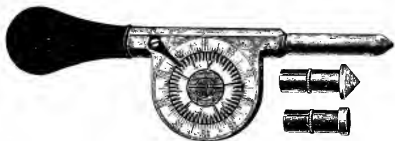
FIG. 59.—Revolution or speed counter.
