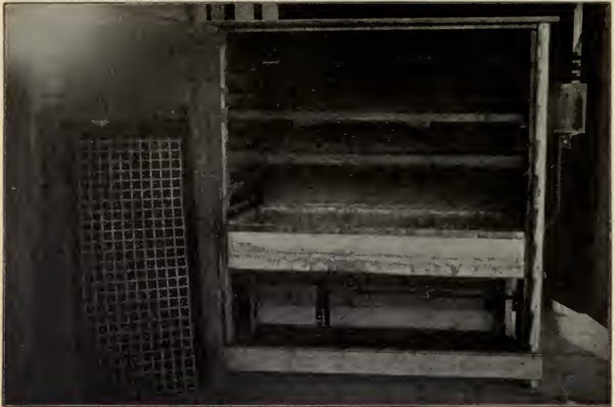
PLATE 4. AN INCUBATOR USED FOR GERMINATING CORN. A GASOLINE STOVE PROVIDES SOURCE OF HEAT.
