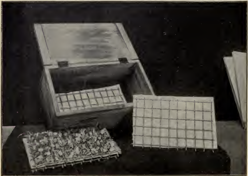
PLATE 6. SHOWING THE WOODEN BOX, BLOTting PAPERS, WIRE GAUZE, AND GROUP OF KERNELS ALREADY SPROUTED.
