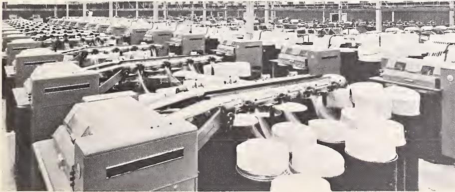
*Figure 18 Drawing—The drawing process follows carding except for combed yarns. This process improves the uniformity of the sliver by converging six or eight slivers and passing them through four sets of rolls, each revolving at a different speed, which draws them out without twisting and reduces them to about the same diameter as one of the original strands.*
