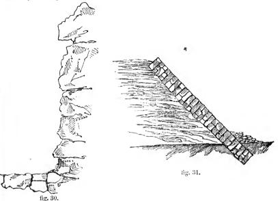
EXAMPLE 27, fig. 31, represents the method of delineating an embankment faced with rubble masonry.
