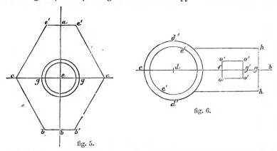
and b; from these points draw lines parallel to cc, from ab measure to bb', e'e'. From e measure to cc; join ce', cb', ce', cb'. The radius of the circle in the centre is eg.
