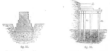
EXAMPLE 32, fig. 36, represents piles of wood driven into the ground, supporting masonry. A section of a coffer-dam in a bed of 'beton' is shown in
