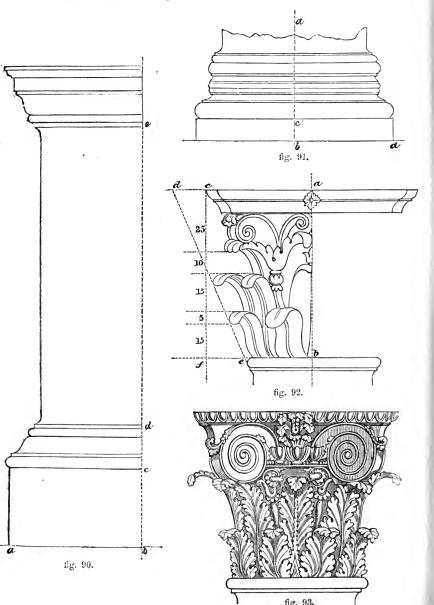
**EXAMPLE** 89, fig. 91, represents the base of the order. Heights, beginning with b c, 10, 7,  $\frac{1}{2}$ ,  $2\frac{1}{2}$ ,  $\frac{1}{2}$ , 2,  $\frac{1}{2}$ , 2,  $\frac{1}{2}$ ,  $4\frac{1}{2}$ , 2, 1; projections, beginning with b d, 42, 42, 38, 36, 37, 37, 36, 36, 37, 36, 34.
