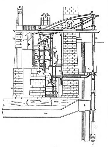
wheel j; and the extremity of m returning, the lever o turns the cock f a quarter round; this admits the steam to the upper-side of the piston, and allows that beneath it to pass into the atmosphere.
