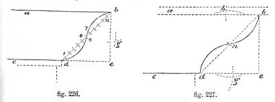
intersection as centre describe an arc dn; from n and b, with same radius, describe arcs cutting in h; from h, with hb, describe an arc meeting the arc dn in n.
