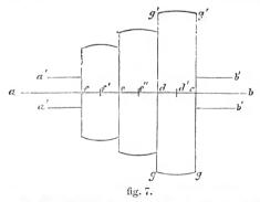
g'g. From c measure to d, through this draw a line parallel to gg'; measure from c and d to g', g. Bisect the distance d c in d'; from d' as a centre, with d' g' as radius, describe the arcs joining the lines through gg', g'g. In like manner, measure from c to e and f: the points f', c' will be the centres of the arcs joining the lines drawn through e and f.
