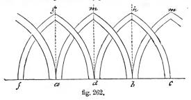
be the breadth of an arch; divide it in b, draw b h; make da equal to db, and draw ag; bh, ag are the centre-lines of two of the arches; dm is the centre-line of the third.
