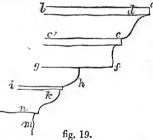
a once perceive that the proportions are very incorrect: thus the distance between the two upper lines as at d is too small, the fillet being too narrow; again the point c, which regulates the extent of the curve from a, is too far from a, while the line cc'is too near the line d; the space between cc' and the line below it is too wide, and the line f is not perpendicular, but slopes outwards towards f; the distance between the line fg and the one immediately above
