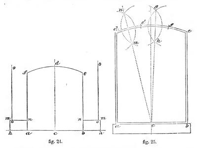
EXAMPLE 25. To draw the circular-headed window in fig. 25. Let ab be the width, bisect it in c, draw cg perpendicular to ab. From a, b parallel to cg draw lines to d and e, the termination of the curve. To find the centre from which the curve dfe is described, take any points e' and f in the copy, and from these points, with radius greater than half the distance between them, describe arcs cutting in g, h. From d and e' in like manner
