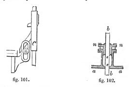
Fig. 101 is a sketch in which the governor connection is dispensed with altogether; the stud m being adjusted by hand to a bracket fixed to the nozzle, the side of the slot in the bracket having a scale to which an index on the stud may be pointed, in order that the engineer may at once place it in a position that the steam may be cut off at the particular portion of the stroke required.
