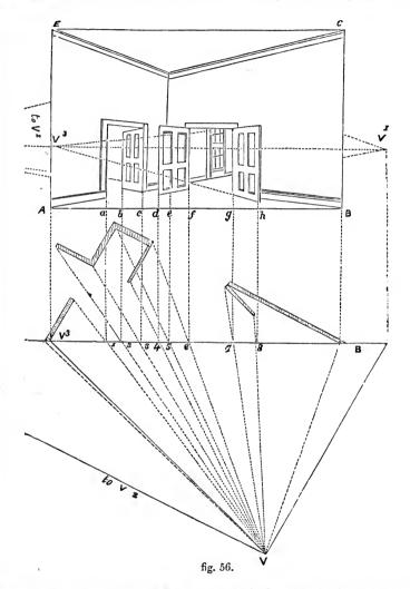
transfer to the picture A B C E; across which draw the horizontal line at the proper height, and by perpendiculars transfer to it the vanishing-points  $V^1$ ,  $V^3$ ,  $V^3$ . Transfer the points *a*, *b*, *c*, &c. in a similar manner to the
