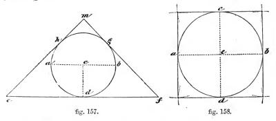
To describe a square about a given circle (fig. 159). Draw two diameters intersecting at i, with the radius of the circle, from the points of the diameters a b, d c, describe arcs cutting in f, g, h, e; join these points,
