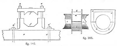
by the bolts dd; and the "cover," a, which is secured to the sole by bolts passing through it, as in the sketch. The journal of the shaft revolves in a space, ff, left in the centre of the block. In order to prevent as much
