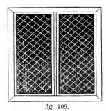
EXAMPLE 107, fig. 109, is the elevation of a rustic window, with lozenge-shaped panes of glass. For the method of laying this out, see Example 5, fig. 5.
