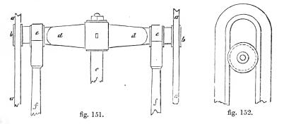
sliding within a slot in the side framing a a, a side view of which is shown in fig. 152. The connecting-rods ef, ef, are attached by straps and brasses to journals made in the cross-head d d, the other ends to two cranks placed beneath the cylinder, which stands on a frame.
