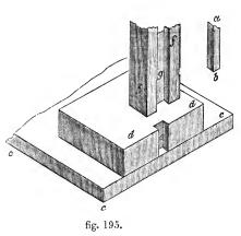
that another portion is subjected to the cutting-edge. Thus by alternately raising and depressing the tool, and moving the article to be cut regularly forward to meet the cutting-edge, a groove of any depth can be cut in the metal, the breadth of which is obviously equal to the width of the cuttingtool, and the length to the thickness of the metal in which the groove is to be cut.
