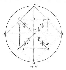
h g, fig. 80), with the radius p 3, an are to 4; from the point o (line gf, fig. 80), with radius o 4, an are 5, and so on from the centres corresponding to the points s, t, v, x, y, &c., describing curves to the points 5, 6, 7, 8, 9, &c. fig. 79.
