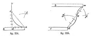
the third from d) by arcs cutting in f; and the part de by arcs in g. From f, with fa, describe the arc ae; and from g, with gd, an arc ed; the moulding is complete.
