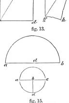
by which the circle is described, as ab, is called the radius, and the diameter, as cab, is double the radius; the boundary-line is called the
