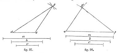
To construct a scalene triangle, having the three sides a, b, c given. Draw ef, fig. 98 = a; from e, with side c, describe an arc; and from f with b cut this in g; join eg, fg.
