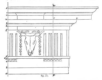
equal 5, the fillet 1; projection of h equal 32; of  $k 35\frac{1}{2}$ ; height of k m equal 6; projection of m equal  $64\frac{1}{2}$ ; of v t equal  $39\frac{1}{2}$ . Height of m n equal 8;
