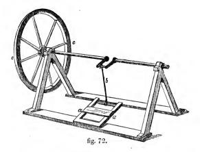
reciprocating motion to the rod b, which turns the axle and fly-wheel *cc*. In the "potter's wheel" the crank is also used to drive his machine; by turning the crank-handle a a, fig. 73, motion is imparted to the fly-wheel b b, from which motion is communicated to the machine by the strap or
