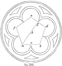
corners of a pentagon, a, b, d, e, f, by dividing e d equally on the point g, and drawing a line from a to it, cutting the perpendicular e c in h; the centre h of the surrounding circles is obtained.
