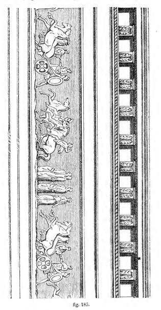
EXAMPLE 184, fig. 186, is the elevation of a sculptured pilaster forming part of a chimney-jamb.
