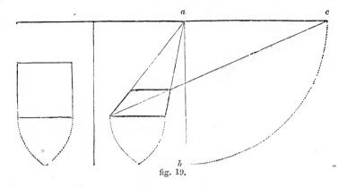
drawn between them; and if a space be set off upon the horizontal line to the right or left of the point of sight (a) equal to the distance so denoted, a b, the point c at the end of that space will be the true distance-point.
