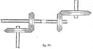
motion in various directions. The " trundle," in conjunction with the "face wheel," as it is termed, has been frequentlv used in corn-mills for changing the direction of motion by
