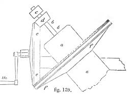
end of the shaft bb; the other end of e works into the face-wheel f; the two motions are thus effected : as thus arranged, the mechanism is that used in a patent "rice-cleaning machine."
