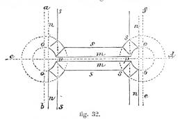
lines m, m; and parallel to same lines, lines s, s touching the eircles. From f e, a b, lay off to nn lines equal to m; and from m, to ss equal to the distance of the line ms from cd; join ps and the points corresponding.
