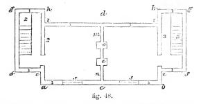
to ab draw ef, and parallel to cd, fg. Parallel to ef draw gh; parallel to cd, hi. Join ii; the outline of the plan is thus obtained. Put in the thickness of the walls, the horizontal lines 1 1 first, the vertical 2 2 thereafter; and the central partition mn, with fire-jambs oo. Put in also the windows ss, and stairs, as in the drawing.
