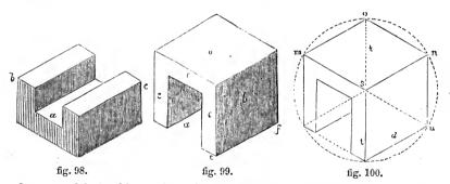
faces o and b, fig. 99, are formed by the upper and right-hand sides of the cube mons and stvn, fig. 100, the parts ccc being drawn by lines parallel to ms and st, the line d being the line corresponding to  $ef_{s}$ . The
