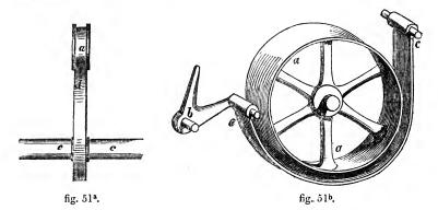
carpet with considerable ease. In the power-loom, the pulley, a a, fig. 51<sup>b</sup>, is stopped when required by the friction-belt, c c c, being tightened on the periphery of the drum by the lever b.
