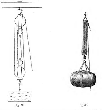
The ropes used about a pulley are called tackle, and the pulleys blocks; therefore, when a sailor or workman collects together all necessary for the application of this machine, he speaks of the *block and tackle*.
