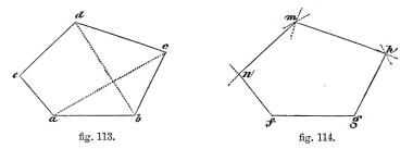
in h, join gh; from g with bd, describe an arc, and from h with ad, cut this in m; from m with de, describe an arc, and from f with ae, cut this in n; join hm, mn, nf.
