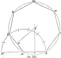
side; with this radius from adescribe a semicircle b q d on a b, produced to d; divide it into seven equal parts; through the fifth of these draw a g; bisect ab, a g in c, e; erect perpendiculars from these points cutting in f; from f, with f a, describe a circle; lay a b from gto h m and n o; join the points. -Meth. 2d. Let a b, fig. 122, be the side; from b, with a b, describe an arc a e; bisect a bin c; draw a perpendicular as ed; divide a e into seven parts, lay one of these from e to d;
