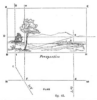
line, B H the base-line, S the point of sight, V the station, and D the point of distance; S D on the picture being equal to K V on the plan. Let M N be the position of the plane of delineation on the plan, and C that of any object (say a tree) beyond that plane. Required the perspective position of such object.
