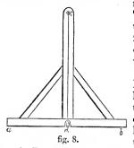
nexed figure (8) represents the mason's level. The under side a b is placed on the wall; if the cord by which the weight d is suspended from c hang so as to correspond with a line on the centre of the upright, the wall on which a b rests is level.
