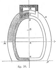
EXAMPLE 25, fig. 26, represents the front elevation of the cover for a gas retort. The centre of the parts b, c, and d is at a on the line de; the centre of the curve joining o p at m, on the line n m.
