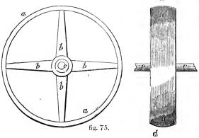
so as to be convex, as d d, fig. 75. In cases where the strain is severe, the belts are apt to slip on the surface of the wheels. Where this embarrassment is merely temporary, from increase in the work to be performed, or from other causes, engineers generally obviate it by strewing the inside of the belt with pounded resin; this is taken
