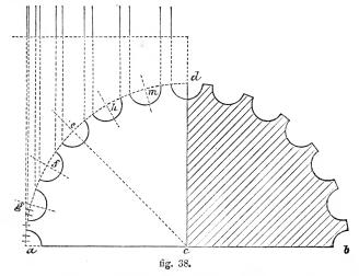
e, and divide the arcs a e, e d, by points g, f, h, m. Mark the position of these by radial lines from c, as in the copy. Divide the part a g into eight equal parts; and with three of these as radius, from the points in the quadrant, as g, f, &c., describe semicircles. Six parts will thus be given to each flute, and two to each fillet: and the column will have twenty-four flutes.
