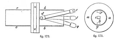
be observed that the steam does not press on the whole surface of the piston, but only in the annular ring a a, between the outside of the trunk b, fig. 173, and the interior of the cylinder in which the piston moves.
