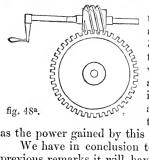
If the winch, fig. 48<sup>a</sup>, be 20 inches long and the screw 2 inches in diameter, here is evidently a power of 20 gained; then if the wheel have 30 teeth and the screw at each revolution throws off one tooth, this is a power of 30 gained, which multiplied by 20, the other power, gives a power of 600. Again, say that the cylinder is only half the diameter of the wheel, that is an additional power of 2 to 1, by which multiply the former power, and the result is 1200
