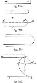
from d draw to e perpendicular to b d, produce a a to e; from e draw through b a line meeting the semicircle b d produced in m; from e as a centre, with e m as radius, describe part of a circle to n.
