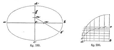
number of equal parts; and from these draw lines parallel to a b, b c; through the points where the corresponding lines intersect as the first from b, with the first from c, draw a curve by hand—this is one quarter of the ellipse, the others may be produced in like manner.
