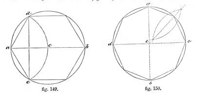
a with ac (the centre of the circle); describe an arc cutting the circle in de; join ad, it is the side required.
