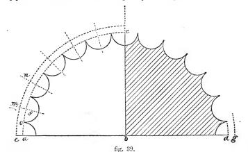
six equal parts, as e, m, n, &c., giving to the entire column twenty-four flutes as before. Draw radial lines from b. Divide af into four equal parts, and lay one of these on ab produced to e; from b, with be, describe a semicircle as emn, cutting the radial lines. Bisect af in o, and with fo as radius, from the points—where the dotted semicircle intersects the radial lines—as centres, describe the arcs as in the copy. Another method is shown in
