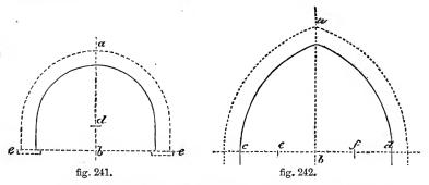
To describe the pointed horse-shoe arch (fig. 242). Draw the lines c b, b a perpendicular to one another; divide c b, b d each into two equal parts at e, f; from e, with e d, describe an arc, and from f, with f c, another, both meeting in a.
