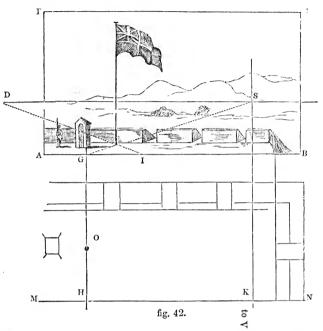
the point of distance is now made use of, as in the perspective drawing of squares; its distance D S from the point of sight being made equal to KN. From the position or place of the object O (in this case a flag-staff) draw O G perpendicular to M N, intersecting it at H. From G, with the radius O H, describe an arc intersecting A B at I, and making G I equal to O H. The diagonal D I will intersect a visual line G S at the required perspective position of the object.
