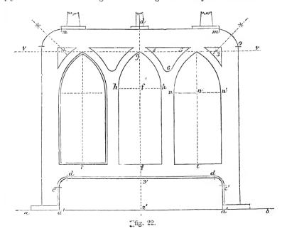
EXAMPLE 21, fig. 22, represents the outline of side elevation of framing. Draw the line a b, and at right angles to it 2' d; measure from 2' to a' a', and to 3'. Through these points draw lines d d, a' c', a' c'; join the points c', d by the part of the circle, as in the diagram. From 2' measure to f, and draw the line tf t; from f measure to t, t; from these points draw
