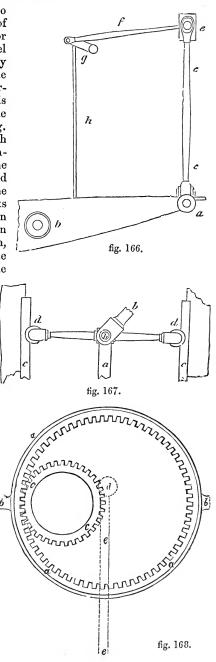
of the wheel cc is one-half of that of the wheel aa, or equal to its radius, then the point d will describe a straight line in the direction de; if the proportions are different from the above, the point d will generally describe a curve known as the hypocycloid.
