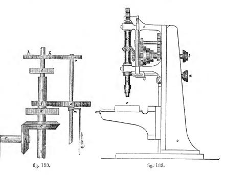
In fig. 189 we give the elevation of a self-acting drilling-machine by Whitworth of Manchester : a b the speed pulleys,
