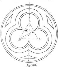
drawn, and the angle bac bisected; a line drawn from a to e, cutting the line cf, gives the centre of the surrounding circles; ab and c are the centres of the trefoil curves.
