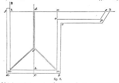
a b into two parts at c; next, on the paper on the board draw any two lines at right angles corresponding to those in the copy, as c d, f d n s. To avoid unnecessary repetition, we wish the reader to understand that, when we give directions to measure any part or distance, as "measure from c to b and a," we mean that the distance c b is first to be taken from the copy in the figure, and transferred to the corresponding point on the
