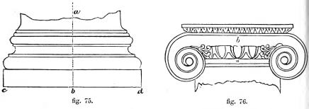
EXAMPLE 76, fig. 76, shows the elevation of Ionic capital drawn to same scale as the others. The plan of the capital is shown in EXAMPLE 77, fig. 77, and the side view in
