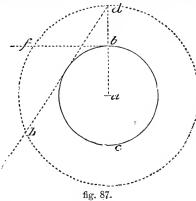
a c at right angles to a b; bisect c d in f; and draw f e at right angles to c d; the point f where they intersect is the centre of the circle.
