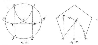
To construct an equilateral and equiangular pentagon on a given line, a b, fig. 106. From a with a b describe the arc b c; draw the perpen-
