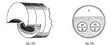
and double-furnaced boiler, a sectional diagram of which is given in fig. 63; aa the flues, bb the furnaces, cc the boiler. This is now in general use, and is fast superseding all other constructions. "It consists," says Mr. Fairbairn of Manchester, "of the cylindrical form, varying from five to seven feet in diameter, with two flues, which extend the whole length of the boiler; they are perfectly cylindrical, and of sufficient magnitude to
