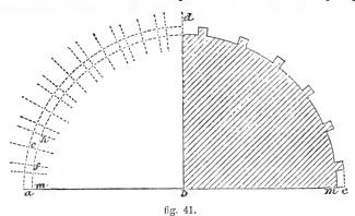
divide a e into five equal parts. With two of these from the radial line, lay
