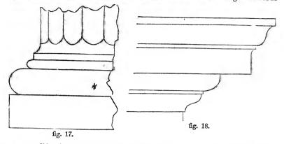
an exemplification of the outline of part of a "cornice" belonging to the Tuscan order. Let us slightly analyse the supposed proceedings of the pupil in delineating this. Suppose fig. 19 to be the rough sketch as first attempted. On examining the copy as given in fig. 18, the pupil will at
