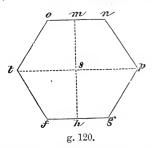
bisect this in s, draw  $t \le p$  parallel to fhg; from m make o = fg; from o, n with fg, cut  $t \circ p$  in t and p; join the points. An irregular hexagon as that in fig. 33 may be drawn in the same way as figs. 113 and 114. Let a b, fig. 121, be the
