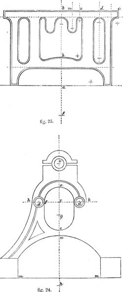
EXAMPLE 24, fig. 25, represents the front elevation of a 'cross head' and 'side levers.' The centre-lines are a d, e h, vv. The plan is shown
