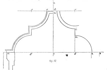
measure to d, and draw f df parallel to a b. From d measure to ee and ff; from c measure to g, and from g, with g h, describe the quadrant h m. From m draw m i parallel to c d; from f, with radius f n, describe the arc meeting the line i. Finish as in the part to the left of the sketch.
