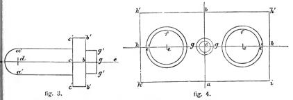
g' g', and from b to b' b'; join g' g' to b' b' by lines at right angles to g' g'. From c measure to c' c'; join b' c', b' c'. From d, with d a' as radius, describe a semicircle d a' a'; by lines parallel to c b join a' a' with the line c' c'.
