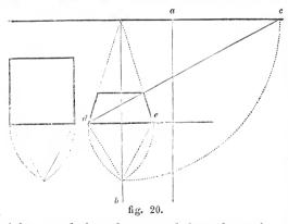
This will determine the perspective lengths of receding objects, by rules to be hereafter laid down. This is further explained in fig. 20, which contains a ground-plan of a square on the left, while the right shows the same square in perspective, and the mode by which the point of distance is obtained. One leg of the compasses is to be placed at the point of
