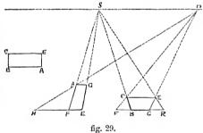
object may be attained by using the visual line S R instead of S B, marking off R G equal to B C on the plan; and drawing the diagonal D G, intersecting S R at E, when R E will be the perspective view of that side on the plan.
