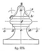
are found by producing perpendiculars from  $o \ o \ to \ d$  and e, cut by lines drawn through the points of intersection of the bisecting circles of the lines  $b \ o, c \ o$ ; the centre of the top circle at  $h \ a$  is found by bisecting lines  $c \ a$ ,  $b \ a$ , and producing the lines of bisection, meeting the perpendicular from a.
