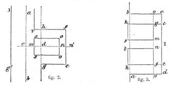
EXAMPLE 3. To draw one jamb with two internal flues. Let a b, fig. 3, be the internal line of wall, a b c d the outline of jamb. Produce the sides h g, h f, to meet the line c d, in the points e e, and m g, n f, to meet b c, a d at the points o, o. Having fastened the paper properly on the board, and
