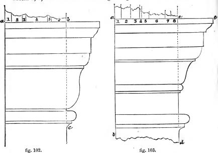
EXAMPLE 100, fig. 102, is the Ionic impost, the projections, heights, and widths 1, 2, &c. of archivolt mouldings being set out as in last figure.
