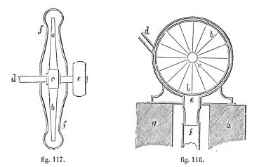
as simple and economical, yet their number is by no means increasing. One great objection to it is the high pressure of the steam employed, and the limit to the power of the engine set by the difficulty of increasing the length of the arms ab, so as to obtain increase of power; the amazing velocity at which the arms revolve, 3000 and 4000 times per minute, makes it liable to speedy disarrangement of parts.
