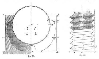
draw b n. From f on the line b f measure to g, and from b to n; through d draw n d g, and parallel to this, through e, 1, 2, 3, &e., draw lines. Next, from d measure on each side of d g, equal to half the breadth of each thread, to n'. These lines terminate at the perpendicular b n: join the angles as in the drawing.
