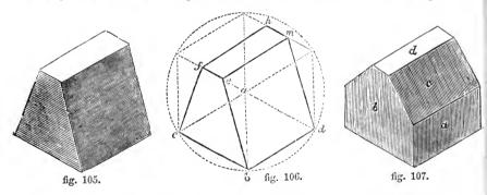
block; from a, the centre of the circle, measure to e and f; from e and f measure to h and m; join
