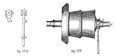
and conical piece are fixed, capable of longitudinal motion on the shaft a, but made to revolve with it; this is effected by having a key e fixed on the shaft, along which the clutch moves in a slot made in its interior surface. Suppose m to be the wheel fixed on the end of the main shaft d, provided with a conical piece c, the interior of which receives
