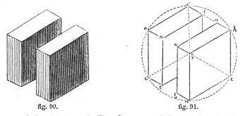
From c and d and b draw the lines bn, cm, and d o, meeting the diagonal oe; from h draw t, v, s, parallel to og; and from g, n, m, o, draw to h, v, t, and s: the representation is complete.
