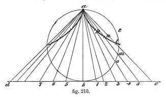
line de, as to 1, 2, 3, 4, 5, 6, 7, and so on; with the distance am cut the line 8 a from 8 in n, and from 4, with ao, cut a 4 in p, and so on. Through the points thus found, on each side of ab, draw a curve as in the diagram.
