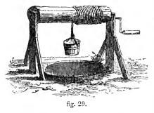
power has to be applied: the cause of this is, that the rope winding upon itself increases the circle on the axle, while the handle describes the same motion through space; and as a larger axle requires more power, the weight feels augmenting.
