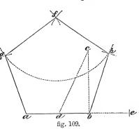
from these draw perpendiculars cutting in g—it is the centre of a circle which will contain db five times; the radius being=gd.—Meth. 4th. Let ab, fig. 110, be the line; from ab describe with ab the circles cbd,
