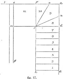
EXAMPLE 17. To delineate the plan of a staircase having 'returns,' by which the direction of the steps is changed. Assume any point in fig.
