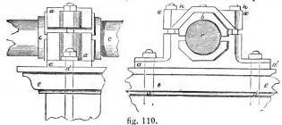
transmitted to the gib, c, tightens up the strap in the brasses embracing
