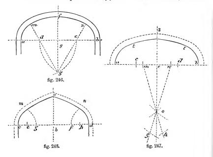
in the point e, and draw a line perpendicular to ab through this; divide ea, eb into two equal parts at c, d; from a, b, with radius ad or bc, describe arcs cutting the line e produced; from d, c, with radius db, describe parts of circles to t, t; divide ae, eb into three equal parts, and lay one of these from e to m, n; from m, n, through o, draw lines to g, h; from a, b, with ab, cut these in g, h; from the points g, h, with radius gt, describe arcs joining t, t.
