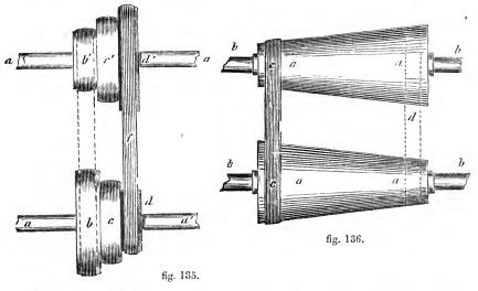
lathes. Another form is used, represented in fig. 136, being two conical drums placed conversely; a a being the drum on the driving shaft b b, a' a' being that on the driven b' b'; by moving the belt c the relative velocities of the two shafts may be changed : this modification is used in the cotton-machine known as the "throstle."
