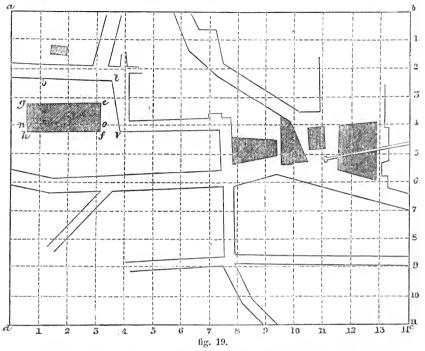
EXAMPLE 19, fig. 19. This example is also designed to show the use of squares in reducing or enlarging maps. The principle of this method has been fully described in *Practical Geometry*.
