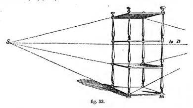
The figures for which rules have been given thus far have been all supposed to be horizontally on the ground-plane, or parallel with it; but such figures frequently stand on their edges, that is, in a vertical plane. Of this kind are the sides of a room, of a house, and of many solid figures. Their perspective form is determined on the same principles, by finding the point in the visual line at which they terminate. Thus, let such a
