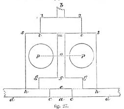
through this parallel to dd; from o measure to pp; these points are the centres of the circles. From a measure to m; draw a line as before, and measure to s, s. From m measure to t, t, and draw lines to 1, 2; put in the thickness of the wall mf.
