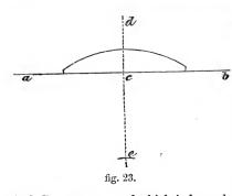
Draw lines on the board corresponding to a b, c d; the centre of the curve will be found somewhere on the line de. By trial  $\overline{b}$  on the copy, it will be found to be at e; measure from c to e, and from e as centre, with e d as radius, draw the curve, joining the short perpendicular lines from a b. The centre from which the part of the circle in the copy is described can easily be found by adopting any of the methods described in *Prac*-
