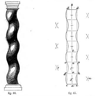
off to *i*. From *i*, with ip as radius, describe the arc ph; from the points g, o, with same radius, describe arcs cutting in s; from s, with same radius, describe the arc og. Next make nt equal to op, and proceed as already described. The various centres are shown by the intersection of the arcs.
