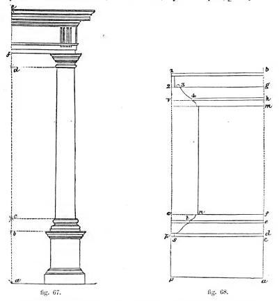
'entablature.' The height of the column, including base and capital, is equal to seven diameters.
