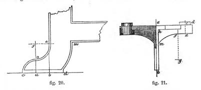
draw lines perpendicular to cd; with ac from a describe the curve co. From b measure to e. Find the centre of the curve joining oe, at f. Find by any of the methods already described the point m; join md by the curve.
