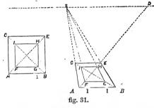
in perspective, its perspective em from corner to corner. If a smaller square be inscribed in a larger, its centre and diagonals will be identical with those of the larger; and one visual line will suffice for determining the perspective of the smaller square. Thus, in fig. 31, the square A B E C being obtained in perspective by preceding rules, draw its perspective diagonals; produce one side G H of the in-
