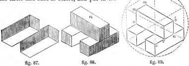
two blocks as in fig. 87; then from e measure to c fig. 89, and from c to d; measure and put in the height of the block from c d to a and b; parallel to the side a', draw from a and b to n and m, and from c to o; join ab, nm, and no: the figure is complete. The two blocks on edge, repre-
