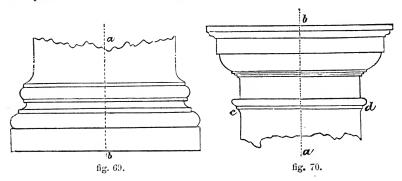
fillet above it;  $5\frac{1}{2}$  to the second torus, and 1 to the fillet above. The projections are set off from the centre-line *a b*, and are as follows, commencing with the 'plinth' equal 40; 'torus' equal 40; 'fillet' equal  $36\frac{2}{3}$ ; fillet beneath the second torus 35; second torus  $36\frac{2}{3}$ ; last fillet 34.
