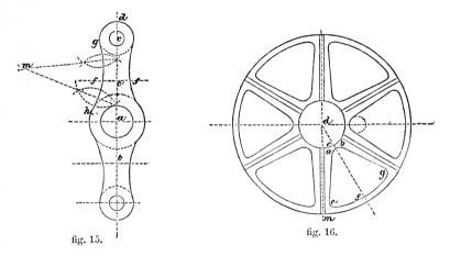
described from the centre d; the circle m is divided into as many equal parts as there are arms in the wheel, any central point of these, as m, being adopted as the datum-point from which to take the measurements. The space between any two of these arms, as  $a \ b$ , is bisected, and a line,
