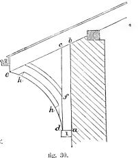
to m, and draw through this a line parallel to ab; measure also to n, and draw nn. From m measure on both sides the distance mo; mn also from n to n, n; these points are the centres of the circles shown in the sketch, the method of putting in of which is still further elucidated by
