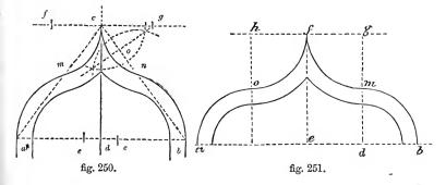
To describe the form in fig. 251. Let  $a \ b$  be the breadth, and  $e \ f$  the height of the canopy arch, equal to half  $a \ b$ ; draw lines  $a \ b$ ,  $e \ f$  at right angles; divide  $a \ e$ ,  $e \ b$  into two equal parts at c, d; from these points draw lines parallel to  $e \ f$ , meeting a line drawn through f parallel to  $a \ b$ ; from c, d, with  $d \ b$ , describe quadrants to m, o; from g, h, with same radius, describe other quadrants joining  $o \ f$ ,  $m \ f$ .
