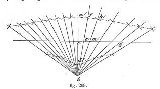
lines, as d ef, b m h, b g; make on the line a b, c d = c a; and on each of the lines drawn from b, take e d = ef, m h = a c, and so on; through the points
