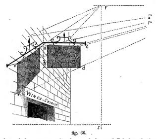
the shadow of the tower on the slopes of the roof, L being the luminary's place, F its foot, and the shadow being thrown rather towards the spectator,
