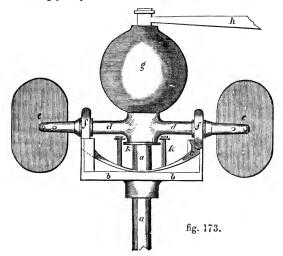
g, and two pins k k screwed into the disc b b; the pins are furnished with adjustible buttons, the lip j will come in contact with these, and prevent the wheels from rising too high.
