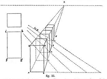
in perspective a row of three square pillars of equal size, a plan of their bases being given in fig. 35, also an elevation of their sides; and let the
