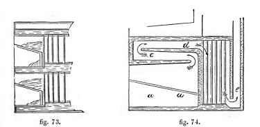
of the Earl of Dundonald, is given in fig. 74: aa the fire-bars (there are four furnaces abreast), the heated air passes over the inverted bridge named the "economical heat trap;" along c and d, and down among the tubes, and finally up the chimney-flue e; by this arrangement, "the heated products of combustion are retained in contact with the most efficient part of the heating surface of the boiler, until the complete ab-
