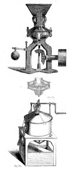
EXAMPLE 52, fig. 55, is a transverse vertical section of the 'patent conical flour-mill,' of which the perspective view is given in
