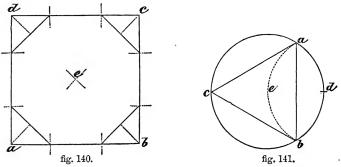
To inscribe an equilateral triangle in a circle (fig. 141). From any point d in the circumference, with d, e (the centre), describe an arc cutting the circle in a, b; from a, b, with a b, describe an arc cutting in c; join c a, c b, a b.
