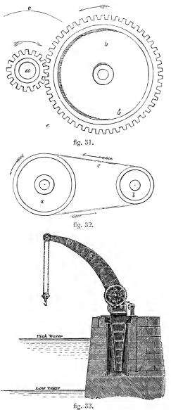
regulation of a quick or slow motion. Thus in fig. 32 the wheel a drives b by the belt c.
