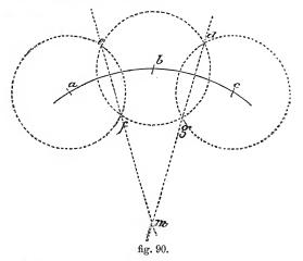
so on; from these points draw to a; from point c, with distance b c, cut g a in g; from g, a h in h, from h the other line from a; these are all points in the circumference of a circle which will pass through a, b, c.
