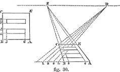
rallel with A B; these will give the longer sides of the rectangles. Draw the visual lines S 5, S 6 to the point of sight, which will give the shorter sides of the rectangles, and complete the figure.
