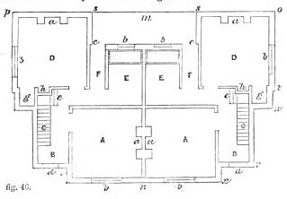
EXAMPLE 46, fig. 46, which is the 'ground-plan' of a pair of cottages, the division or party-wall being at m n, AA the living-rooms, D the kitchen, E the scullery, F the back lobby, B the front lobby: aa are fire-places, b windows, d doors. The method of copying this is given in
