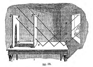
supposed to pass through an opening in a wall, falling upon a table, and thence reflected to the plane d e f g, set up on it at the position 1, in which position all the three rays are reflected upon it. But if we suppose it moved backwards to the position 2, it can only receive one (a) of the reflected rays, the others passing away over it.
