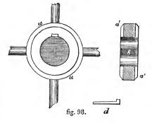
tions, commonly called "ruffs" or "collars." As the "eye" or centre of a wheel to be fixed on a circular shaft is generally bored out, it is necessary that there should be some means adopted to prevent the wheel from turning round or shifting on the shaft. This is effected by cutting, in the first place, a longitudinal "slot," or groove, along the inside of the eye of the wheel or pulley, as in fig. 98 at b; this may be done at only one side, or
