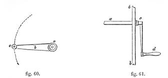
fig. 61 illustrates the method adopted in starting and stopping the engines of a locomotive : bb is part of the boiler through which the rod aa passes to the value to which it is connected; a lever, c, is moved by the handle d
