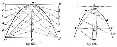
any line f h g; bisect it in h; draw h m o; join m f; from f, at right angles to m f, draw a perpendicular cutting m n in n, divide h n into four equal parts: lay one of these from m to p and o: p is the focus; through this draw a line parallel to f g—it is the parameter—a line through o parallel to this is the directrix.
