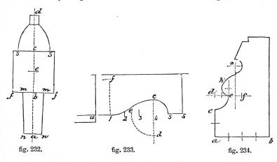
To describe the moulding in fig. 234. Draw a b, divide it into four equal parts; make ac equal to two of these, and cdequal to one; through d draw df parallel to ab; from d, with dc, describe the arc ce; make ef equal to ed; from the centre, above e, describe the part of the circle to h; from f, with fh, describe the curve meeting the semicircle described from o.
