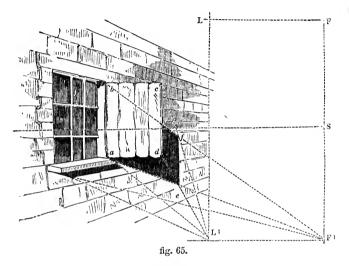
shutter, as thrown on the wall from the sun's place L, in front of the picture, draw L F perpendicular to the shadow-plane, cutting it at F, which is the foot of the luminary. The shadow being in this case thrown from the spectator, invert the luminary, as in fig. 63. Draw  $F^{1}a$ ,  $F^{1}b$ , and  $L^{1}c$ ,  $L^{1}d$ , crossing each other respectively at e and f; join e and f, and efa b is the outline of the shadow, part of which is hid by the shutter.
