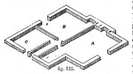
clear and distinct style; the height at which the walls stand being 12 or 14 inches. But the whole height of a wall may be shown by this mode of drawing as well as its thickness; thus, in a future example the reader will find the isometrical drawing of a house with the height of the walls
