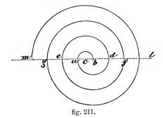
semicircle b a; from b, with a b, the semicircle a d; from c, with c d, the semicircle d e; from b, with b e, to f; from c, with c f; to g; from b, with b g, to l; from c, with c l, to m; the spiral is complete.
