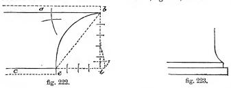
and c that of the shaft; produce c to d; divide a d into four equal parts; lay five of these from d to e; join e d, bisect it by arcs cutting in f; from f, with f a, describe the arc a e.
