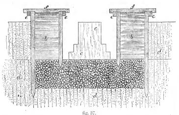
EXAMPLE 33, fig. 37, where cc is the mass of masonry, resting on the mass of beton; dd represents mud; ec the main piles and 'wales,' and j'j' the cross-pieces; b represents the elay-puddling between' the piles, which serves to keep out the water from the interior. For explanation
