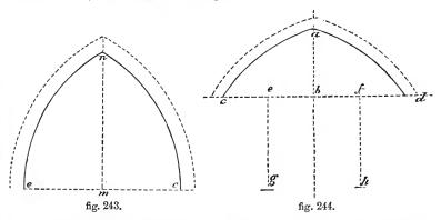
To describe the early English arch, given in fig. 244. Draw the lines  $a \ b, c \ d$  at right angles; divide  $c \ b, b \ d$  into two equal parts at e and f; from these points draw lines to g, h perpendicular to  $c \ d$ , and make  $e \ g, f \ h$
