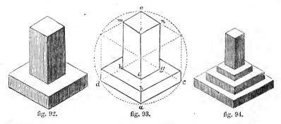
and giving the breadth of the faces of the oblong block; from e measure to f, and put in the square om, fn; join all the points, and the figure is complete, the distance ef being the height of the block.
