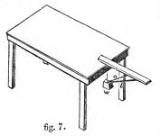
be perceived, fig. 7, that the weight wwould fall to the ground if the cord a, to which it is attached, were allowed to hang straight; but by placing a piece of wood b reaching to the end of the stick, the weight is pushed to one side, and its centre of gravity is underneath the table: thus both the stick and weight are supported by it. The reason of this is, if the stick to which the weight is suspended had to fall, the weight must rise upward towards the table; and being
