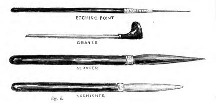
the "burnisher," and the "hand-vice." These are all delineated in the annexed diagrams (fig. b). An etching-table must also be provided, with the following accessories :---
