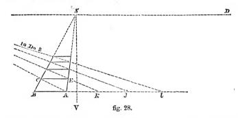
The same rule is applicable to finding the perspective sides of parallelograms. Thus, for a perspective view of the parallelogram A B C E, the dis-
