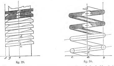
distance between them; the line from g is the line of the inside of the screw, the line f the outside line of the threads. The last example shows the method of copying this.
