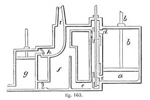
water in the cone, frees the air-pump bucket from an unnecessary weight of water. The air-cone is now frequently dispensed with. Two orifices
