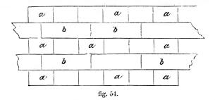
sists of alternate layers of brick 'headers' and 'stretchers,' a a being the 'headers,' and b b the 'stretchers.'
