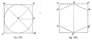
To inscribe a hexagon in a given square (fig. 139). Bisect the side a c into two parts in the point b; divide a b into seven equal parts; lay three of these from a to d; join b d; and with this distance lay off to e in the side a d e; from e to f, g and h, join the points.
