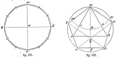
To inscribe an equilateral triangle in a given pentagon (fig. 152). Jointhe opposite angles by lines db, ec, cutting in g; join af through g; lay off fg from g to h; from h, with ha, describe a circle about the pentagon; from a, with ah, describe the arc mhn; bisect mh, hn, in o, o; through these from a draw lines cutting eb, dc in s and t; join st.
