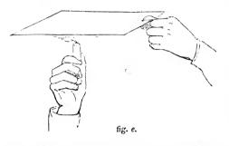
portion of the plate required. On an even and complete layer having been obtained, take a wax-taper (fig. e), and next proceed immediately to smoke the ground; the taper must be kept in motion, in or der that the whole of the ground may be evenly blacked: if the flame of the taper is allowed to remain too long in the
