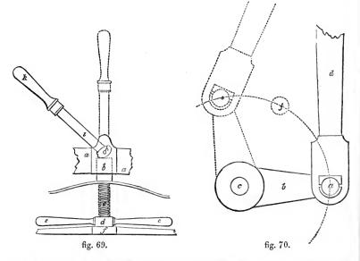
brought into action, which acting on the screw by means of the cam h, depresses the plate f with great pressure.
