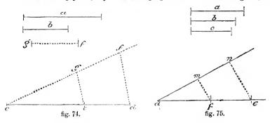
the two lines. Draw any line c d, equal in length to a b, joined; from c draw a line cf at any angle to c d, make cg=ce or a, join ge; parallel to this, from d, draw df; fg is the third proportional.
