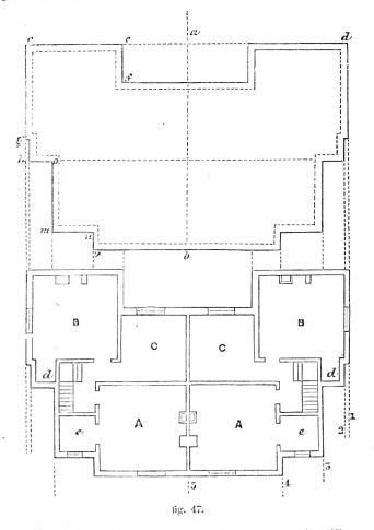
fig. 46. Measure os, fig. 46, and lay it off from c to e, fig. 47; at right angles to this draw ef, and make it equal to sc in fig. 46. Draw eg at right angles to ce, and make it equal to ot in fig. 46; make the short 'return' at g equal to that at t in fig. 46. Parallel to gc draw gh, and make it equal to tu in fig. 46; make the return ho at right angles to gh, and equal to that at u in fig. 46. At right angles to this draw om, equal to uv:
