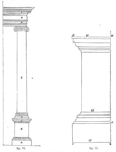
EXAMPLE 74, fig. 74, shows the elevation of half of Ionie pedestal; the line ab being that from which the projections are taken; the plinth bc is  $28\frac{1}{2}$  parts in height, and 57 in projection. The upper fillet ad is 2 parts high, and 57 in projection. The width of die is 42 parts. The whole height of pedestal from a to b is two diameters 34 parts, or 4 modules 4 parts. The heights of the other mouldings and projections are as follows,
