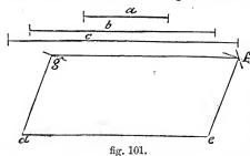
d, e with a describe arcs to g, f;from d with c, cut that in f, at f; from f with distance b, cut that in g; join d g, g f, f e.
