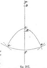
To describe a hyperbola by means of points. Draw any indefinite line a f(fig. 207); set off on it the transverse, bc. Let d be the focus; equal to d c from b set off to a; from a, with any radius greater than b a, describe an arc : fr
