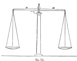
on each side are made of equal length, and suspended over the centre of gravity. The axis or pivot b, which is the point of suspension, is sharpened to a very thin edge, sometimes equal to that of a razor, that the beam may easily turn with as little friction as possible when weights are applied in the scales. Should the arms not be of equal length, then the scales
