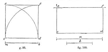
Let a be the breadth and b, fig. 100, the length; make cd=a; from c, with radius b, describe an arc to e; raise the perpendicular ce, cutting the arc; from d, with radius b, describe an arc at f; from e, with a, cut this in f; join ef, fd.
