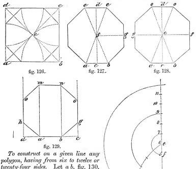
twenty-four sides. Let a b, fig. 130, be the line; from b, with a b, describe an arc a e; bisect a b in c, and erect an indefinite perpendicular, as c e; divide the arc a e into six equal parts; from e transfer these to the line ec.
