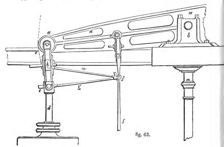
part. The great beam, a a, is a lever, the centre of vibration of which is at b; the links, cc, are also levers, the centres of which are at the ends of the lever g, and at the points where they are attached to the beam; the centres of the lever mg are at h and f. The result of this combination may be here generally stated; although the end, ac, of the beam describes a
