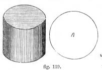
method. In fig. 119 is given the representation of a cylinder, the method of drawing which will be learned from the construction of the preceding figure. In fig. 120, a hollow cylinder B is represented, of which A is the geometrical plan. And in fig. 121, a cylinder B, represented with a square hole D, running in the direction of its length, and supported on a square plinth cc; this figure is an exemplification of the mode in which pillars can be drawn isometrically.
