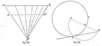
db is the tangent — Meth. 2d. Let b cf, fig. 85, be the circle, and c the point through which the tangent is to be drawn; from a draw ac; through c draw ecd, at right angles to ac; ecd is the tangent.
