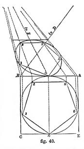
The same rule will apply, whatever be the form of the base and number of sides. In architectural drawings the spires of churches are easily drawn by this rule. If the base be a circle, find its perspective centre by drawing the eircumscribing square with its diagonals, whose intersection will be the foot of the central perpendicular line. In this case a single line from the apex to each side of the base will complete the figure.
