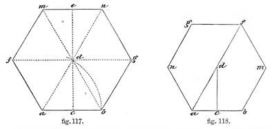
A hexagon, as fig. 119, being given, to draw another equal and similar to it. Bisect a b, fig. 119, in c; draw c d, and join the opposite angles by a Draw fg (fig. 120)=a b; bisect it in h, draw h m = c d; line through e.
