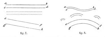
Curved lines, as a b, c d, fig. 8, may also be parallel, and circular lines, ef, gh; these are termed also concentric, as in fig. 86 are two concentric circles. The sides of a figure, or the boundary-lines, are those within which the figure is contained, as a b, c d, fig. 13, are the sides of the figure abcd; the line cd is called the *base*, on which the figure rests
