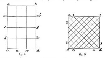
EXAMPLE 5. To draw the diagonal lines representing the panes in a rustic window, fig. 5. Draw cd, making it equal to cd in the copy; cd is the side of the square abdc, which describe. Divide the sides cd, ac, each into six equal parts; join the corresponding points, as 1, 2, 4, 5, 3, 6.
