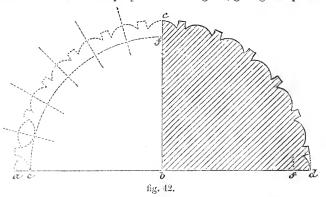
as in that example. From b, with b e, describe the semicircle eff. From the points where the radial lines intersect this, as centres, with radius a e, describe the curves as in the copy.
