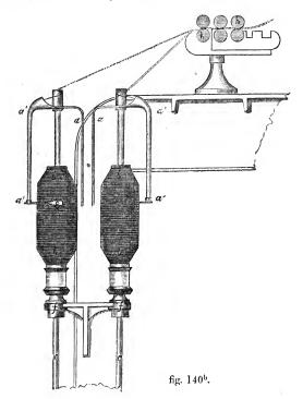
spindles cc; the yarn is delivered to the bobbins at x, passing from the rollers through the hollow leg of the flyer a'a'; the bobbins rest loosely on the copping-rail ff; this rail is made to rise and fall by means of racks and a pinion, thus making the bobbins pass up and down on the spindles cc, and opposite the "finger" x; thus each part of the bobbin is presented to the delivery-finger at x.
