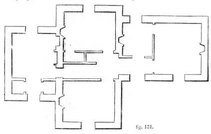
the same scale used for the plan in fig. 131. The pupil should try to draw the geometrical plan from the isometrical sketch, and *vice versâ*; if he can do this with facility and correctness, he will be able to proceed to the isometrical delineation of any geometrical plans which may be presented to him. In concluding this part of our present volume, we would earnestly advise the reader wishful of having an acquaintance with this attractive
