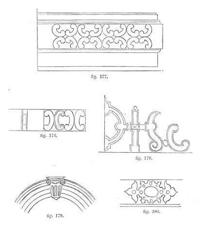
EXAMPLE 174, fig. 176, is the elevation and end view of a pierced parapet in the Elizabethan style.
