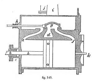
The cylinders of locomotive engines are always of the three-ported species, as in the diagram, fig. 149. aa the piston; b the piston-rod; c the stuffing-box; d the exhaust-port, leading to the exhaust-pipe i; g the valve; h valve-rod; e port to upper side of piston; f port to under side; k cleansing and greasing-cock. Cocks are supplied to cylinders in some instances at top and bottom of cylinder : these are opened when required
