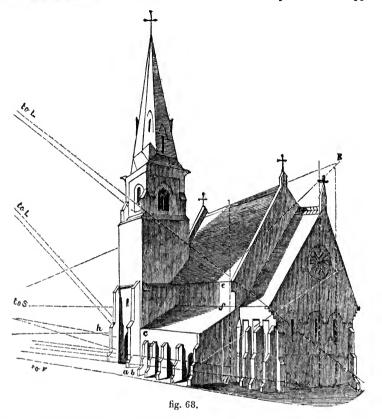
roof; find the perspective position of the furthest angle of the tower, and by the same process of finding its shadow-line on the ground-plane, and erecting a perpendicular where it crosses the centre-line under the ridge, the intersection of the shadow with the ridge and the boundary-line of its other side are found. The shadows of the buttresses are found by the simple process shown on a larger scale at fig. 69, and those of the church itself are obtained by preceding rules.
