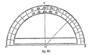
down by means of an instrument called the 'protractor:' it may be
