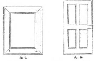
"mitre" joints, as they are termed. By first drawing the simple outlines, as in fig. 10, the foundation of a door is obtained, which is finished by filling in the extra lines, as in the figure.
