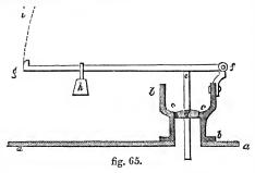
part of a circle at each vibration, yet the piston-rod, d, traverses up and down in a straight line. In the proper place we will fully investigate the *rationale* of this elegant adaptation of one of the simple mechanical powers. In the "governor," another important appendage of the steamengine, the lever is the principal feature; in an advanced portion of this treatise we
