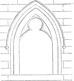
fig. 22. useful practice. Fig. 21 is part of the arch and mullion of a window. Fig. 22 is an outline-sketch of a gothic recess in a wall.
