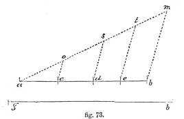
cut, and gh the line to be cut. Join gh to ab, making any angle, as am; join mb; parallel to this, through c, d, e, draw lines to o, s, t—these are the points cutting am equal to gh.
