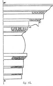
the torus, height 4, projection 56; fillet  $\frac{3}{4}$ , projection 55; cyma 5, projection 47; fillet 1, projection 47; cyma  $3\frac{1}{2}$ , projection 42; die 3 modules  $4\frac{1}{2}$  parts; projection of die, 42 parts; the cavetto in cornice  $3\frac{3}{4}$ , projection 43; fillet  $\frac{3}{4}$ , projection 46; quarter-round  $4\frac{3}{4}$ , projection 50; corona  $4\frac{1}{2}$ , projection 53; cyma  $3\frac{1}{2}$ , projection 57; the top-fillet  $2\frac{1}{2}$ , projection 57.
