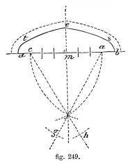
radius eb, describe parts of circles to m, n; join ac, bc; bisect cn, cm (from where the lines ac, bc cut the circles described from e, e) in o; draw lines through the points of intersection of the bisecting circle, meeting cgf in f and g; from f and g, with radius gn, describe parts of circles joining cm, cn.
