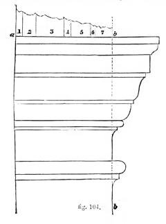
being set out from the line c d towards e, the width of archivolt mouldings 1, 2, 3, &c., as a c, from c towards a.
