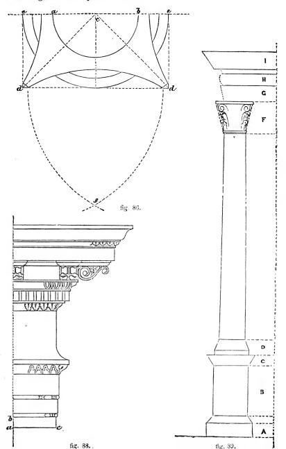
**EXAMPLE** 88, fig. 90. The pedestal. The heights, commencing with b c, are as follows: 33,  $4\frac{1}{2}$ , 1, 3,  $1\frac{1}{2}$ ; 1, height of die d e 4 modules 5 parts. The height of mouldings in cornice, beginning at e, are as follows:  $1\frac{1}{2}$ , 3,  $8\frac{1}{2}$ , 1,  $5\frac{1}{2}$ ,  $3\frac{1}{2}$ ,  $2\frac{1}{2}$ . The projections, beginning with a b, are 57, 57, 55, 46, 45, 42,  $44\frac{1}{2}$ , 47,  $52\frac{1}{2}$ , 53; top-fillet 57.
