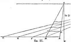
The same object may be accomplished by prolonging the base-line on the side opto D posite the distance point, and setting off on it the width of each of the proposed squares, as B F, F G, G H, fig. 27; a diagonal from each of the points F, G, H, to the distance-point, will, by its intersection with the visual line
