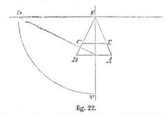
fig. 22, be shown in parallel perspective. Draw the horizontal line, and on it mark the *point of sight* S; which, as we shall first suppose the spectator to stand directly opposite the square at the *station-point* V, must be perpendicularly over that point, as denoted by the line S V. From S, with the radius S V, set off the *distance-point* D on the horizontal line, by
