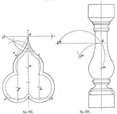
In fig. 268 we give the *drawing of a Baluster*. a is the centre of the lower curves; the centres of the upper curves are found by drawing a line c b; from a and b describe arcs cutting in d; from d, with radius d a, describe an arc cutting the line c d in c; c is the centre of the curve.
