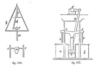
"steeple-engine," much used in the Clyde. a is the piston-rod, carrying a triangular cross-head bb; c the paddle-shaft, d the connecting-rod, attached at one end to the upper extremity of the cross-head bb; and the parallelism of the piston-rod is maintained by the guide e, in which the cross-head mworks.
