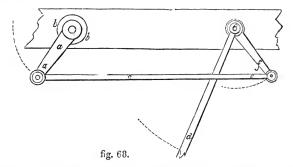
ment of levers in the well-known "copying press" is shown: the plate f is first pressed in close contact with the article subjected to pressure by means of the lever dee acting on the screw c; thereafter the lever ki is
