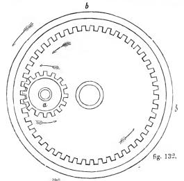
The RELATIVE VELOCITY of wheels, shafts, &c. may be altered and modified by simple means. Thus, suppose in fig. 31 (p. 19), the large wheel is three times the diameter of the small, then it is evident that the former will revolve only once, while the latter will revolve three times. Again, in fig. 32 the small pulley revolves faster than the large one just in proportion as it is
