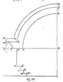
os, os. From s draw st parallel to ab. Finish the circles as in the copy. The method of putting in the part from g to v will be more fully described in
