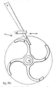
allows each tooth to pass it: but on the wheel beginning to move in a contrary direction, it catches in the bottom and side of the tooth, and prevents it moving. This movement is used in cranes and windlasses, where it is essential to prevent the rope unwinding; it is also used by the mechanic in boring holes in metal, as will be described hereafter.
