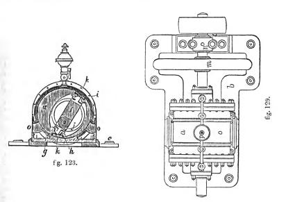
main-engine shaft, d, is passed eccentrically through the cylinder, and in the vertical line of the minor or conjugate axis of the ellipse. The castiron rotatory piston e is suitably fitted with packing-pieces, and slotted trans-
