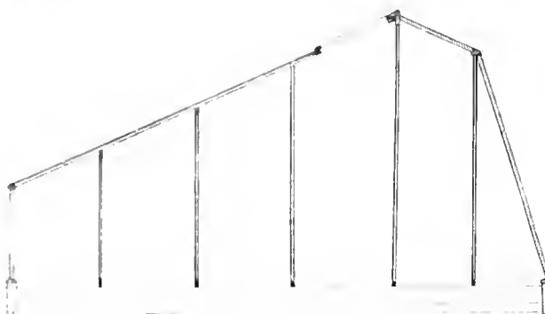
2148. Showing type of greenhouse constructed to obtain the maximum amount of light in short winter days. Modification of type shown in Fig. 2147. Obstructs more light than Fig. 2147, but could be built wider.
