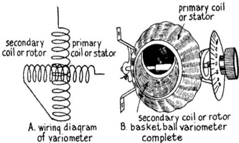
FIG. 54.—How the Variometer is Made and Works.
