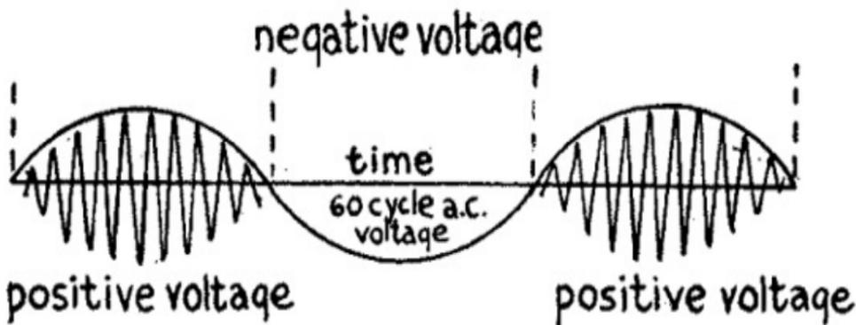
FIG. 95.—Positive Voltage only sets up Oscillations.
