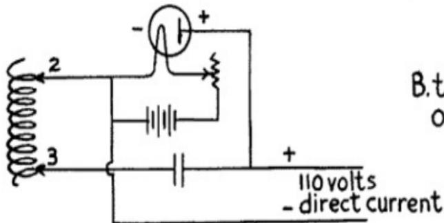
A- the high voltage direct current and plate oscillation circuits
