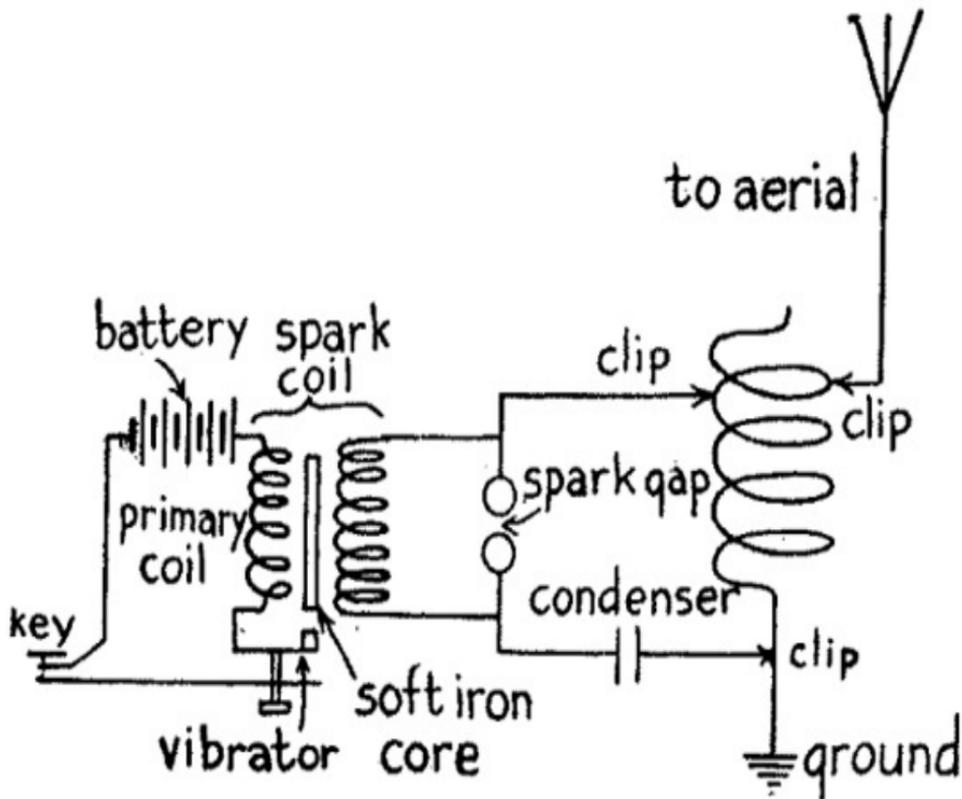
(B) FIG. 20.—Wiring of Diagram for Sending Set No. 1.
