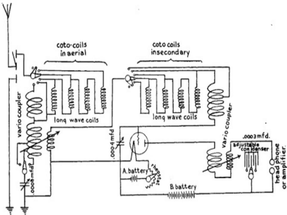
FIG. 59.—Wiring Diagram Showing Long Wave Receiver with Variocouplers and 8 Bank-wound Inductance Coils
