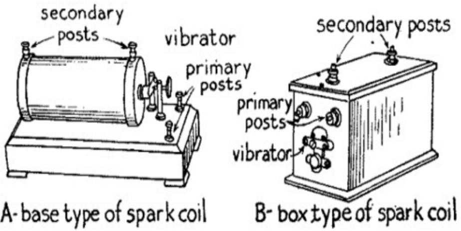
(A) and (B) FIG. 18.—Types of Spark Coils for Set. No. 1.
