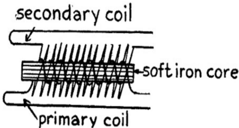
A. wiring diagram of induction coil
