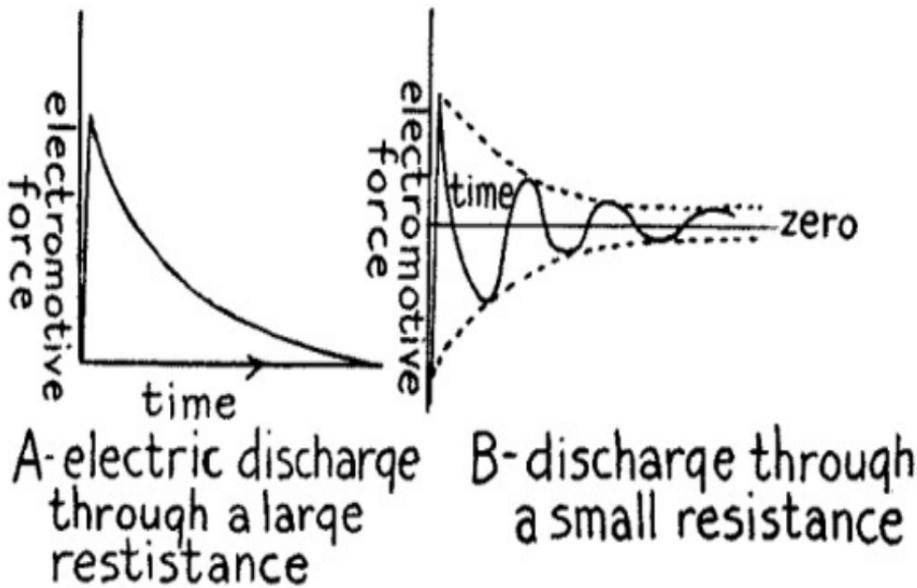
FIG. 83.—The Effect of Resistance on the Discharge of an Electric Current.
