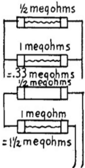
B ways of connecting up grid leak resistances
