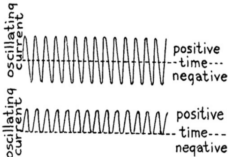
(C) FIG. 71.—Only the Positive Part of Oscillations Goes through the Tube.
