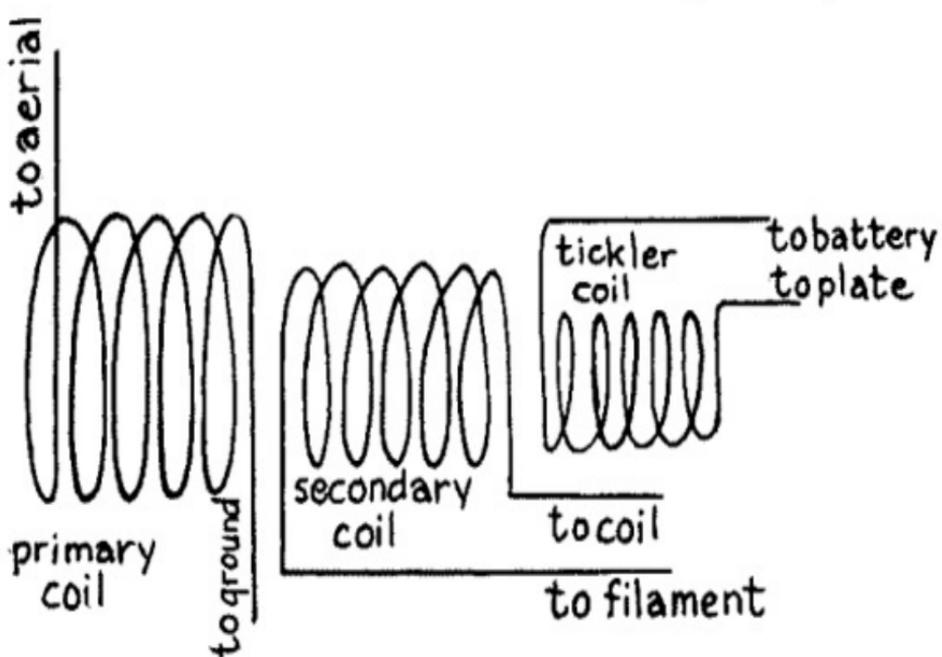
(A) FIG. 49.—Diagram of a Three Coil Coupler.
