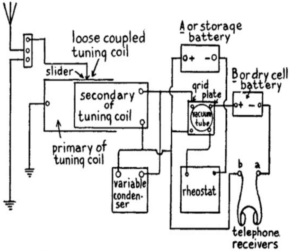
(A) FIG. 41.—Top View of Apparatus Layout for a Vacuum Tube Detector Receiving Set.
