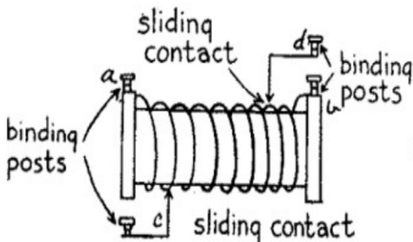
(A) FIG. 11.—Schematic Diagram of Double Slide Tuning Coil.
