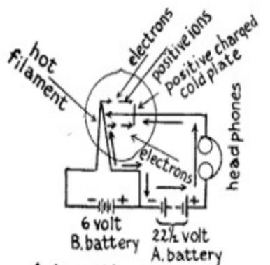
A. how the batteries are connected in
