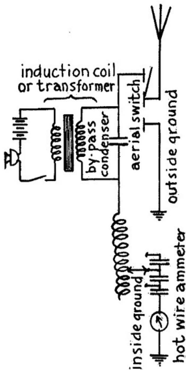
(B) FIG. 89.—Microphone Modulator Connected in Aerial Wire.
