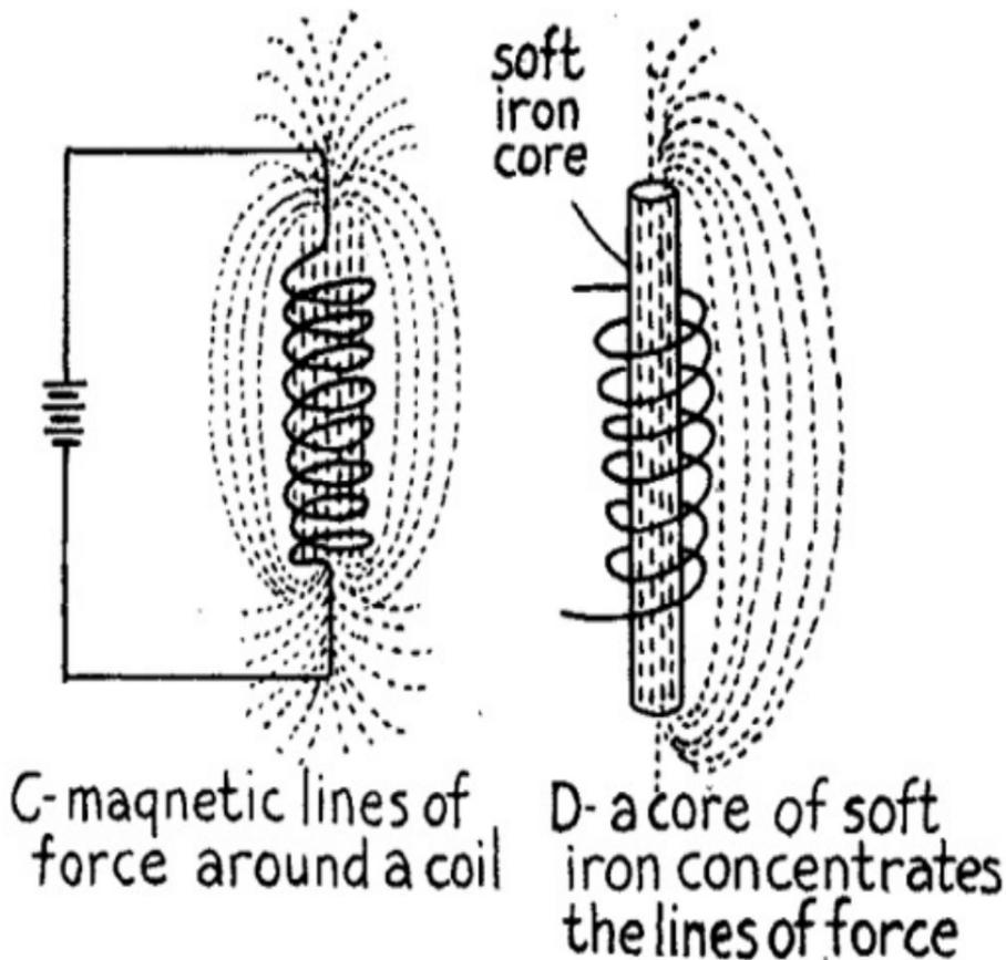
(C) and (D) FIG. 32.—How an Electric Current Sets up a Magnetic Field.
