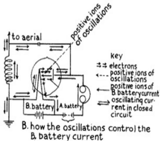
(A) and (B) FIG. 71.—How a Two Electrode Tube Acts as a Relay or a Detector.
