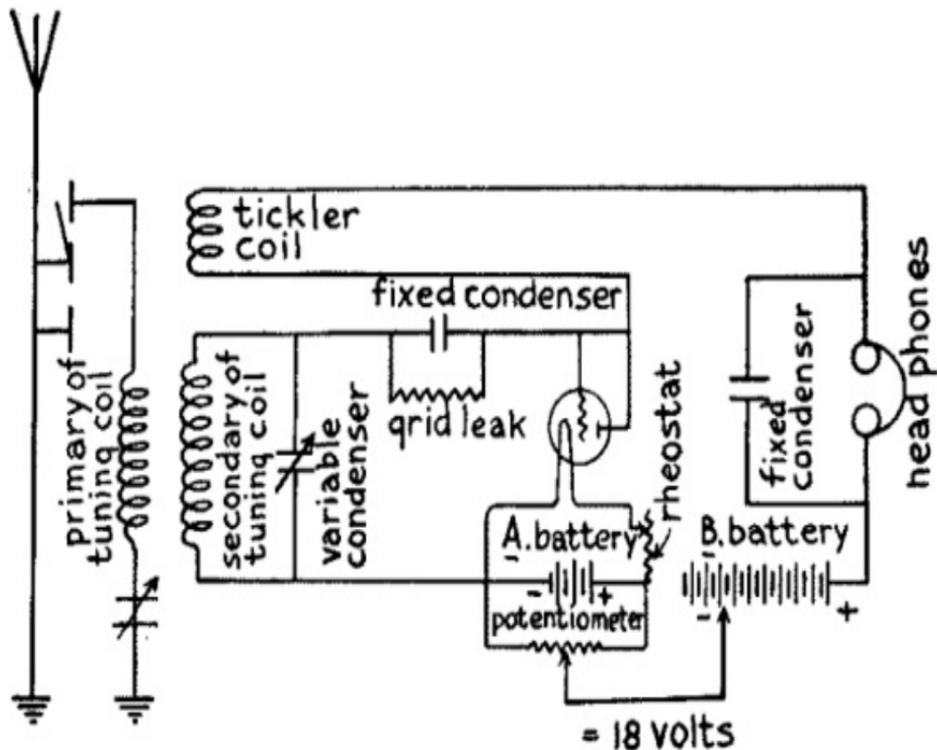
(B) FIG. 47.—Efficient Regenerative Receiving Set. (With Three Coil Loose Coupler Tuner.)
