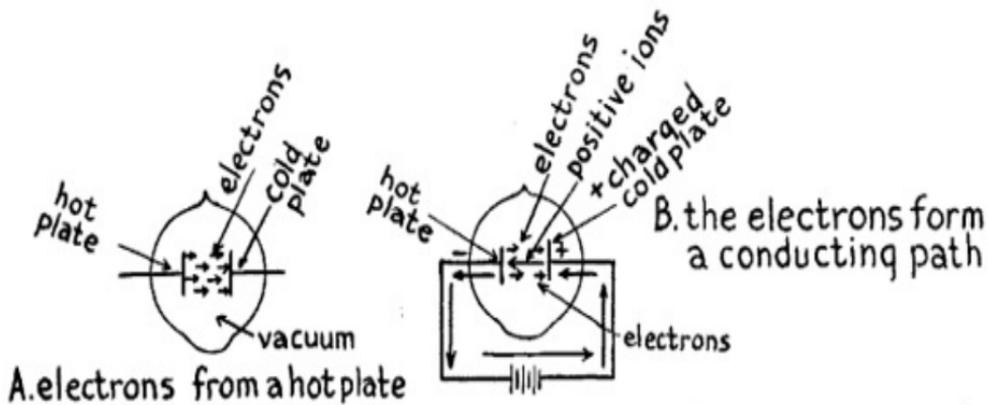
FIG. 70.--Action of Two-electrode Vacuum Tube.
