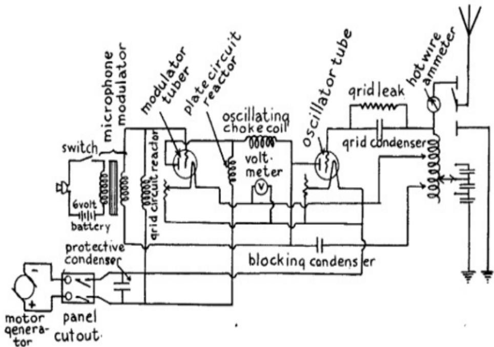
FIG. 90.—Wiring Diagram of 50 to 100 Mile Wireless Telephone Transmitting Set.
