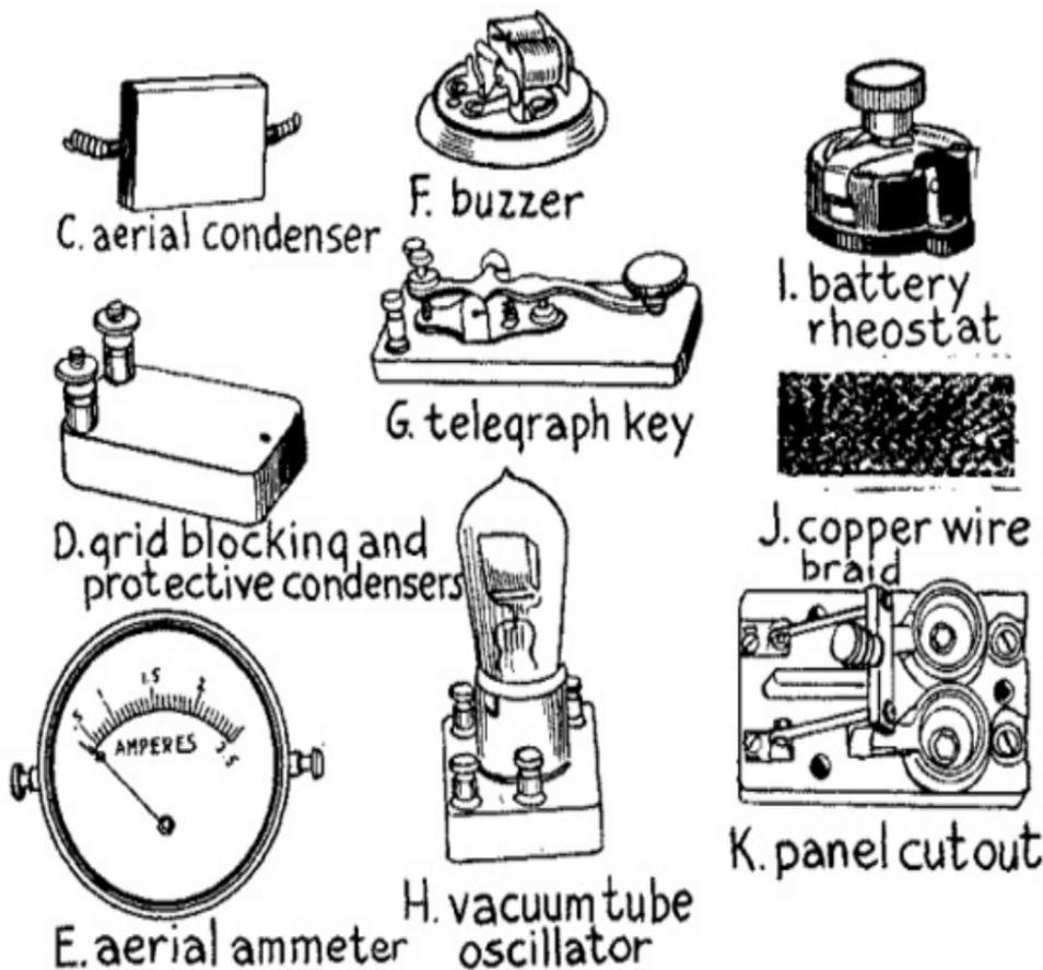
(B) FIG. 75.—Apparatus for Experimental C. W. Telegraph Transmitter.
