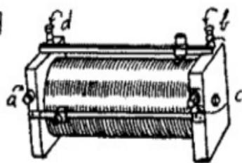
(B) FIG. 11.—Double Slide Tuning Coil Complete.
