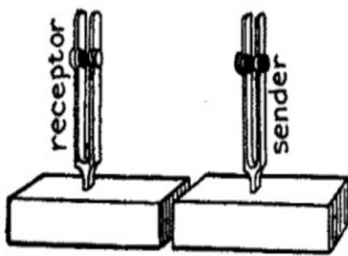
A—variable tuning forks for showing sound wave tuning
