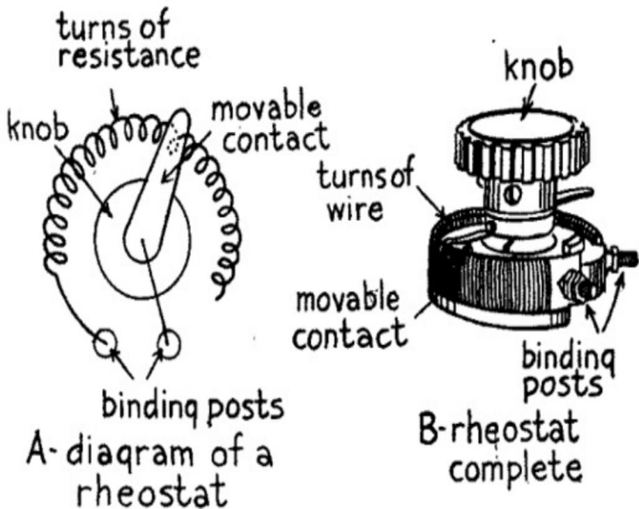
FIG. 40.—Rheostat for the *A* or Storage Battery Current.
