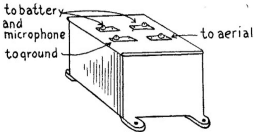
FIG. 88.—Magnetic Modulator. (Used with Microphone Transmitter.)
