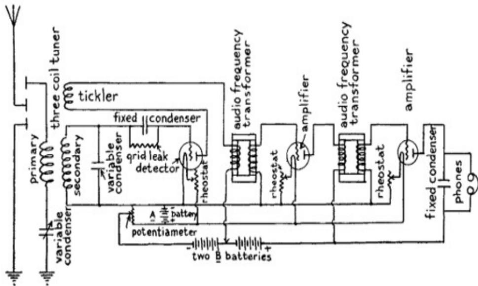
FIG. 52.—Regenerative Audio Frequency Amplifier Receiving Set.
