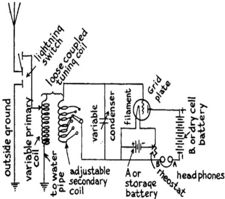
(B) FIG. 41.—Wiring Diagram of a Simple Vacuum Tube Receiving Set.
