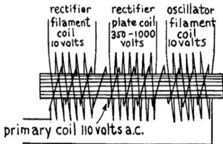
A. wiring diagram of a power transformer
