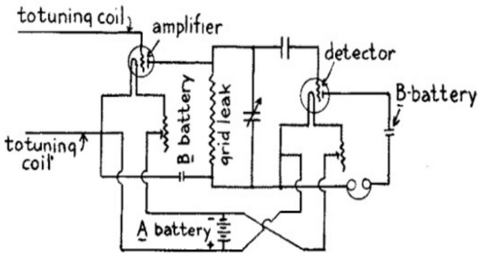
(B) FIG. 44.—Wiring Diagram for Using One A or Storage Battery with an Amplifier and a Detector Tube.
