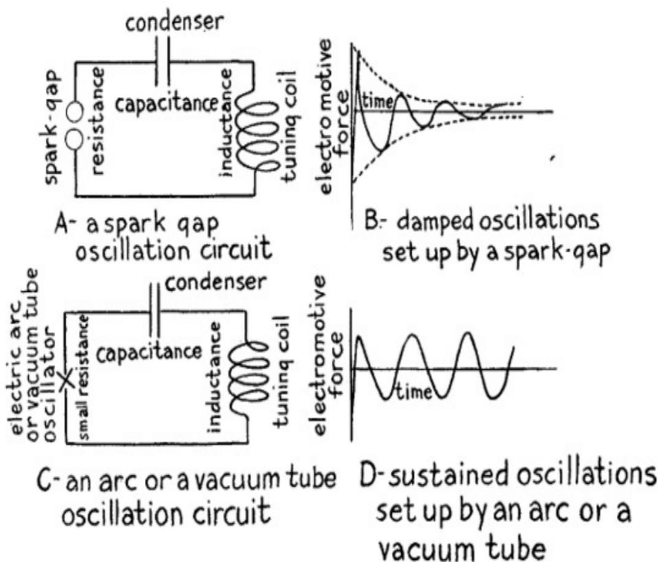
FIG. 35.—Damped and Sustained Electric Oscillations.
