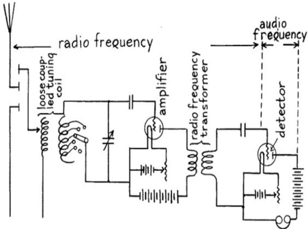
(A) FIG. 45.—Wiring Diagram for a Radio Frequency Transformer Amplifying Receiving Set.
