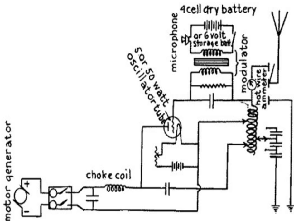
(A) FIG. 89.—Wiring Diagram of 25 to 50 Mile Wireless Telephone.
