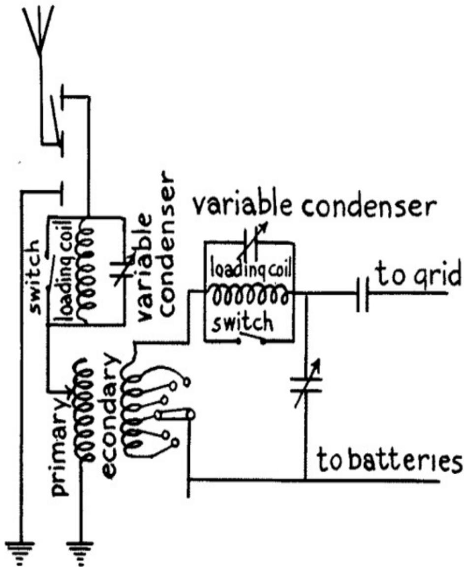
FIG. 57.—Wiring Diagram Showing Fixed Loading Coils for Intermediate Wave Set.
