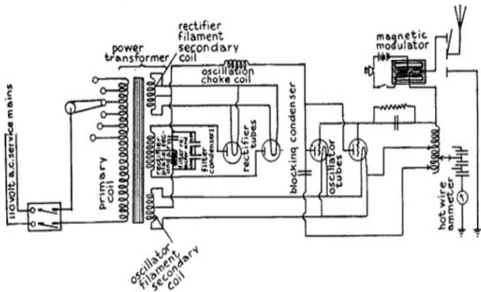
Fig. 93.—100 to 200 Mile Wireless Telephone Transmitter.
