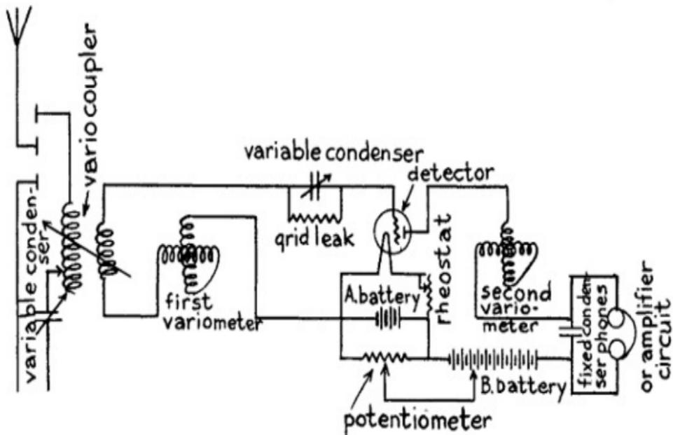
FIG. 56.—Short Wave Regenerative Receiving Set (two Variometer and two Variable Condensers.)
