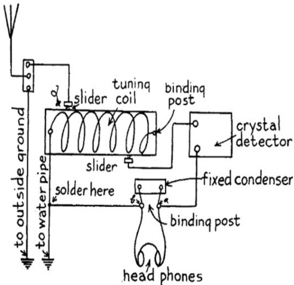
(A) FIG. 15.—Top View of Apparatus Layout for Receiving Set No. 1.
