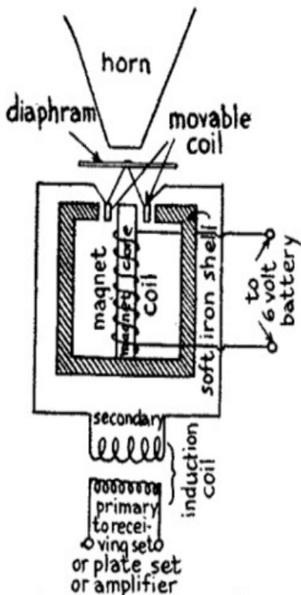
A. wiring diagram of magnavox
