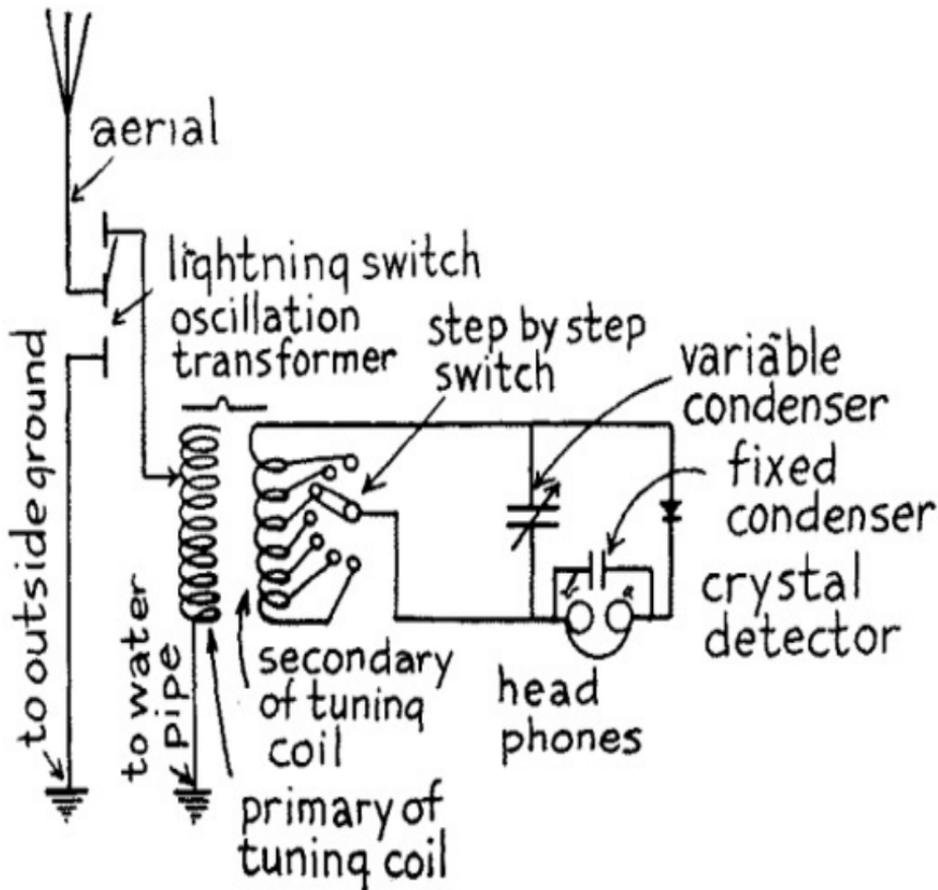
(B) FIG. 16.—Wiring Diagram for Receiving Set No. 2.
