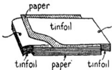
(A) FIG. 13.—How a Fixed Receiving Condenser is Built up.
