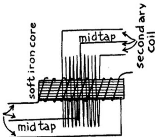
A. wiring diagram of microphone transformer
