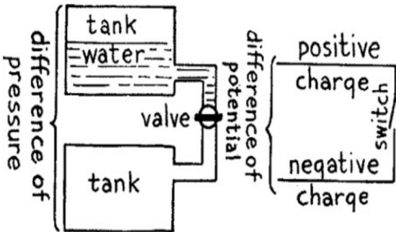
A- water pressure B- electric pressure
