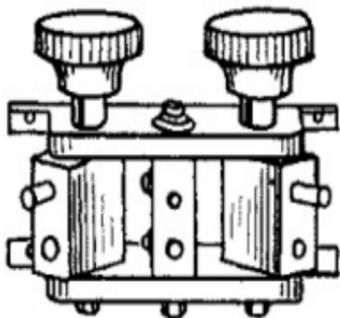
B- mounting for three multilayer inductance coils
