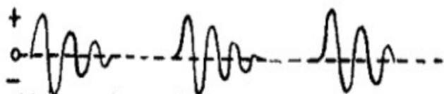
(a) + and - voltage impressed on the grid by oscillations
