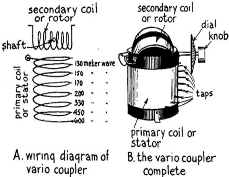
FIG. 53.—How the Variocoupler is Made and Works.
