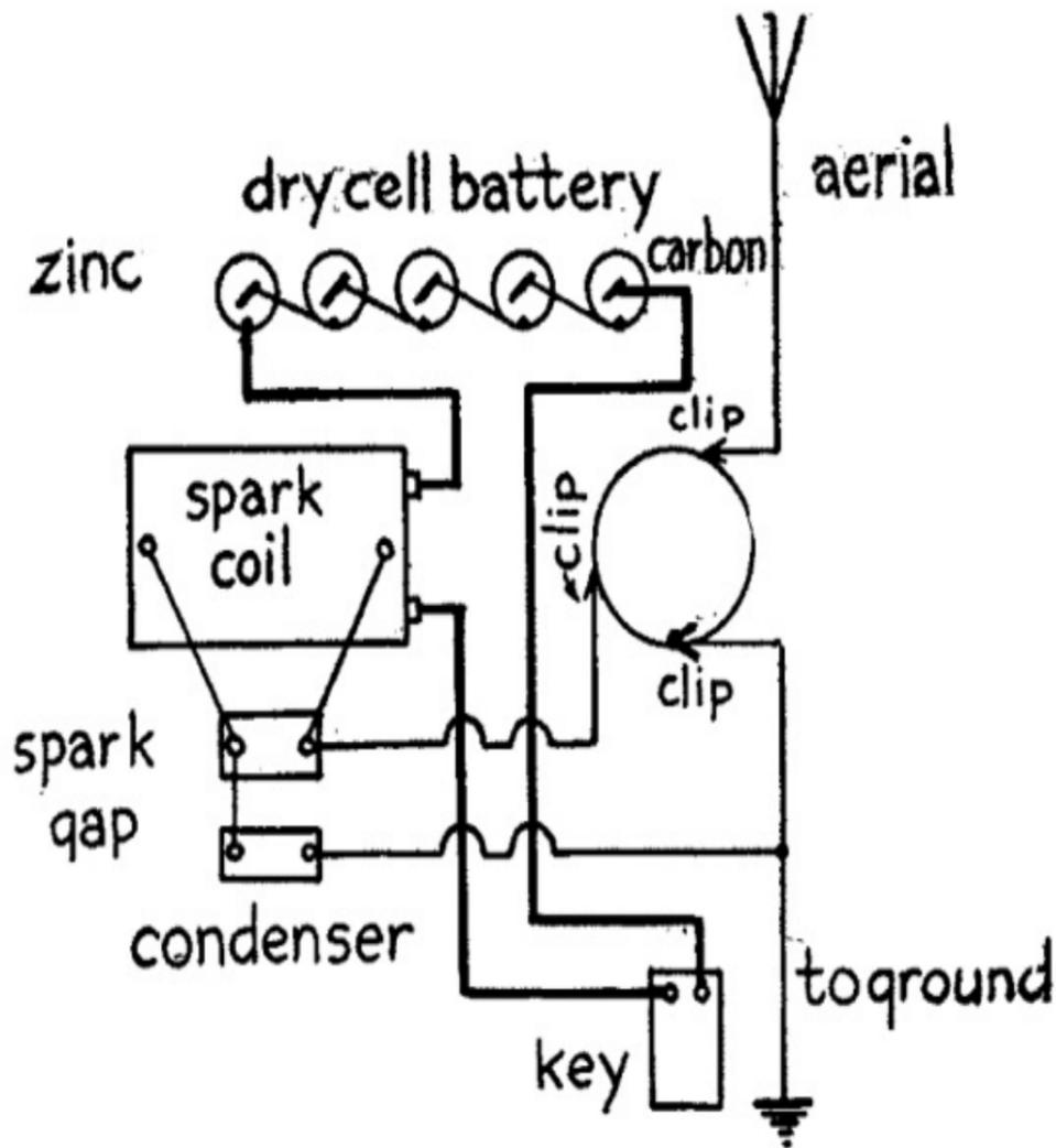
(A) FIG. 20.—Top View of Apparatus Layout for Sending Set No. 1.
