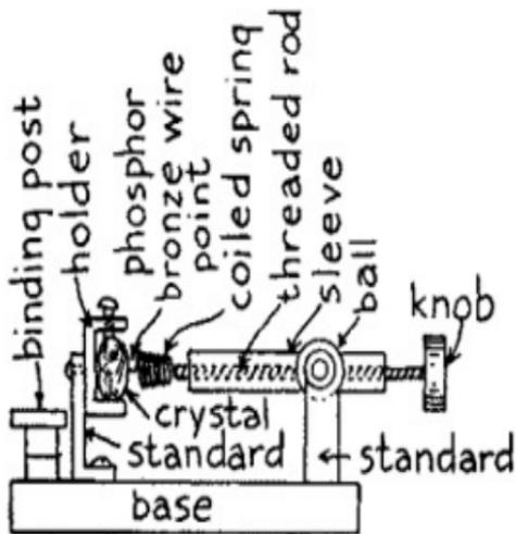
(A) FIG. 10.—Cross Section of Crystal Detector.
