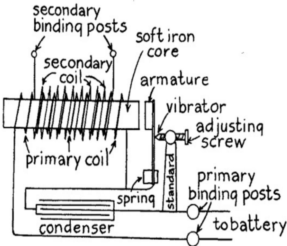
(C) FIG. 18.—Wiring Diagram of Spark Coil.
