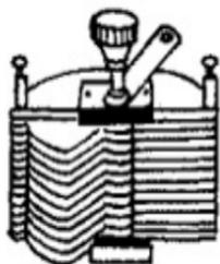
C-fixed and movable plates of a rotary condenser
