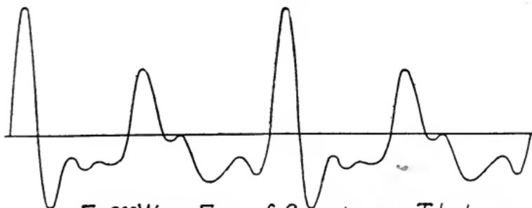
*Fig.285 Wave Form of Current on a Telephone Line Transmitting the Sound of "a" as in "father"*
