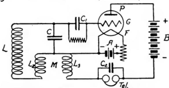
Fig.275. Regenerative Circuit for simultaneous amplifying and rectifying.
