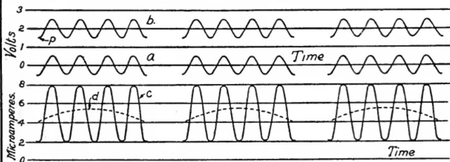
Fig. 248 Action of crystal detector with booster battery.
