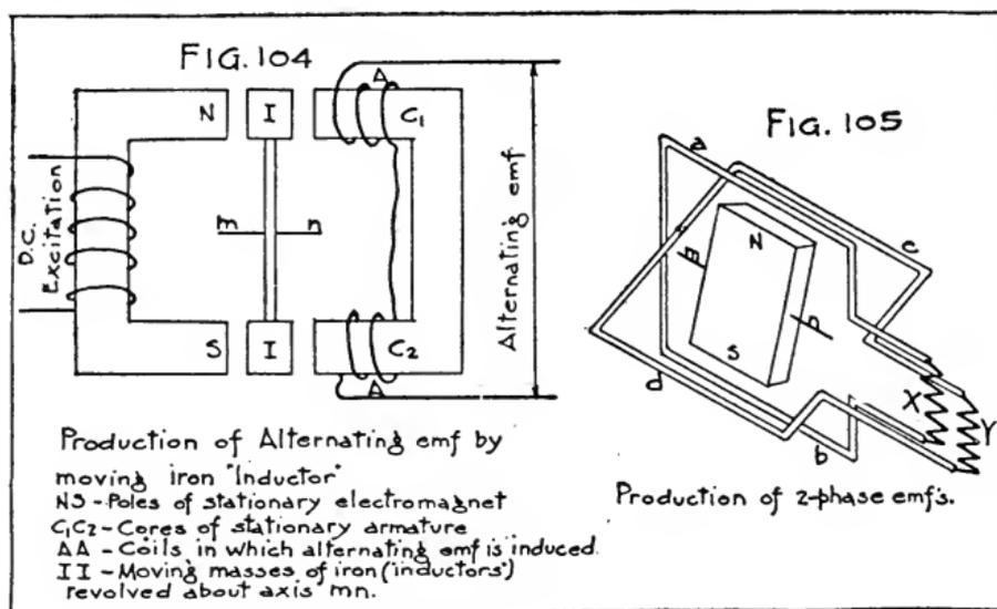
which have a very much smaller permeability than the iron conductors. The flux is consequently less. The increase and decrease of magnetic flux in the coils *AA* sets up an alternating emf., because any change in the flux inclosed by a circuit sets up an emf. in the circuit (Sec. 45) in the one direction while the flux is increasing, and in the opposite direction while it is decreasing.
