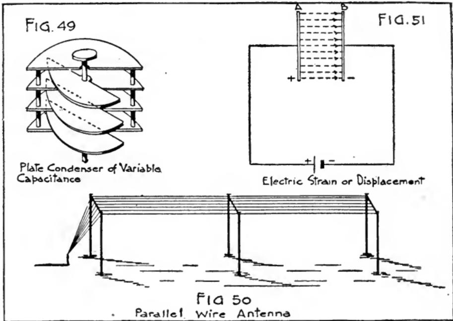
can be calibrated so that the capacity corresponding to any angular setting of the rotating part is known. Condensers used in radio circuits are represented by certain symbols. These symbols may be found in Appendix 3, page 553.
