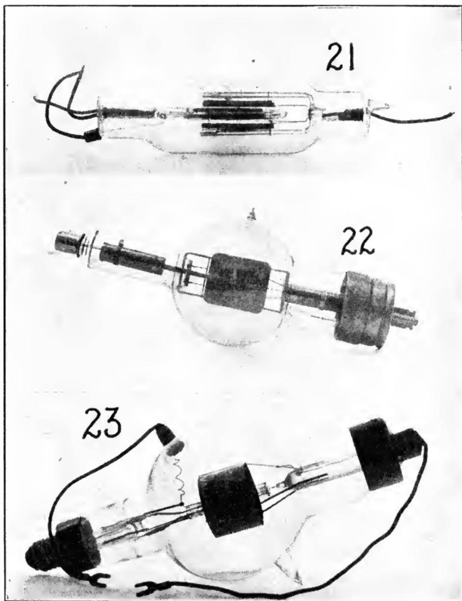
FIG. 266.—Large transmitting tubes.
