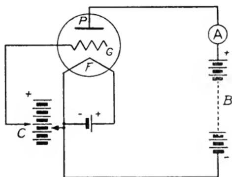
*Fig. 257 Use of Grid in the Electron Tube*
