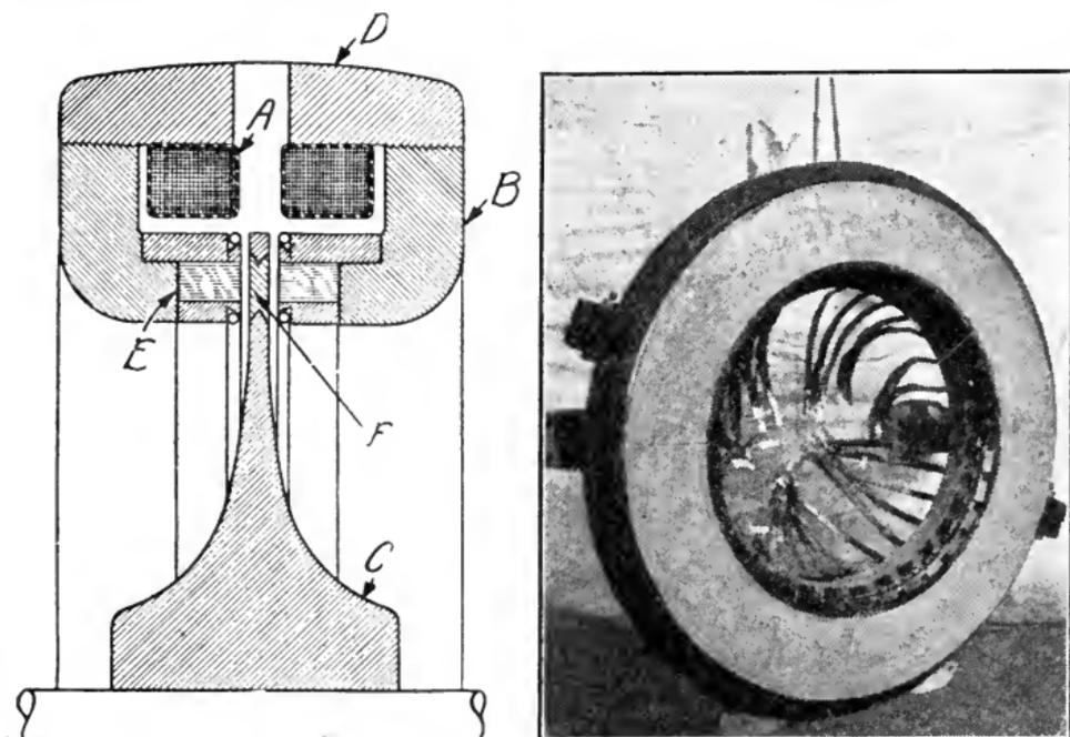
FIG. 126a (left).—Section of Alexanderson alternator, showing rotor.
