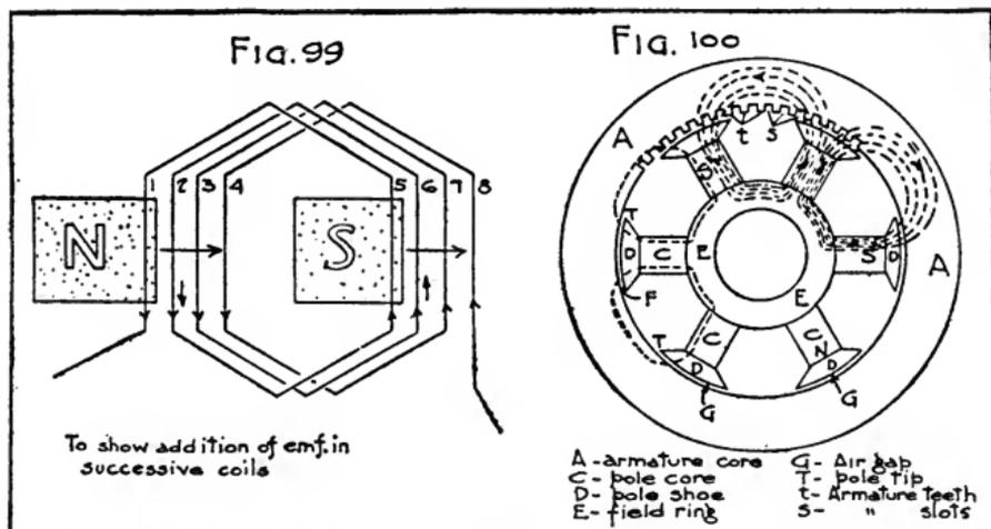
resultant electromotive force begins to decrease, falling to zero and then beginning to increase in the opposite direction. In this manner an alternating emf. is gotten in which the changes occur gradually as conductors get into or out of the magnetic field one by one, or at least coil by coil. In addition the edges of the poles are usually tapered off ("chamfered") to make the changes still smoother.
