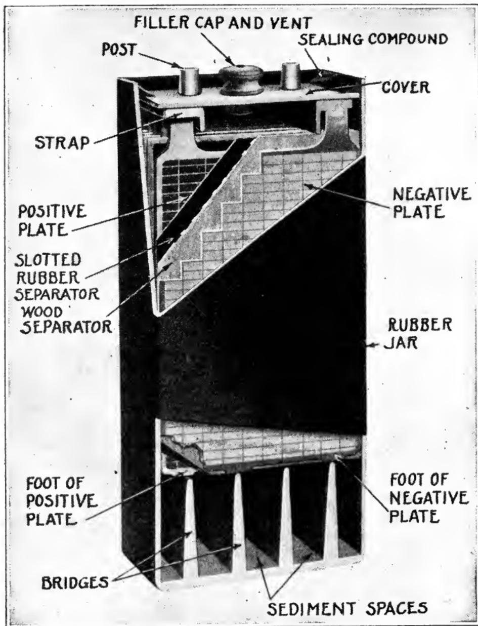
FIG. 29.—Storage cell. Lead plate-acid electrolyte type.
