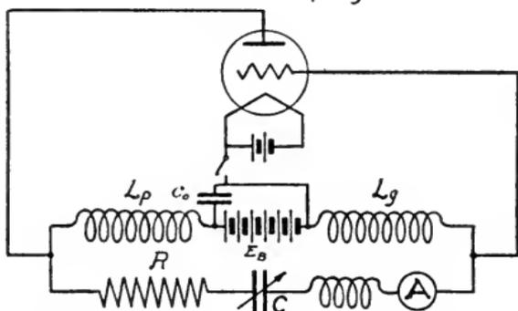
Fig. 280. Electron Tube Generating Circuit Direct Inductive Coupling
