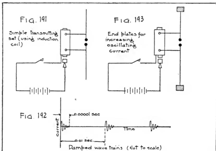
one or more wires, horizontal or nearly so. See Fig. 194. A relatively large capacity can thus be added, and the constructional difficulties and arrangements of support are simplified. This assemblage of wires forms the "antenna." A variable inductance coil inserted in the antenna wire will permit tuning to different frequencies or wave lengths. Thus a simple transmitting outfit is built up.
