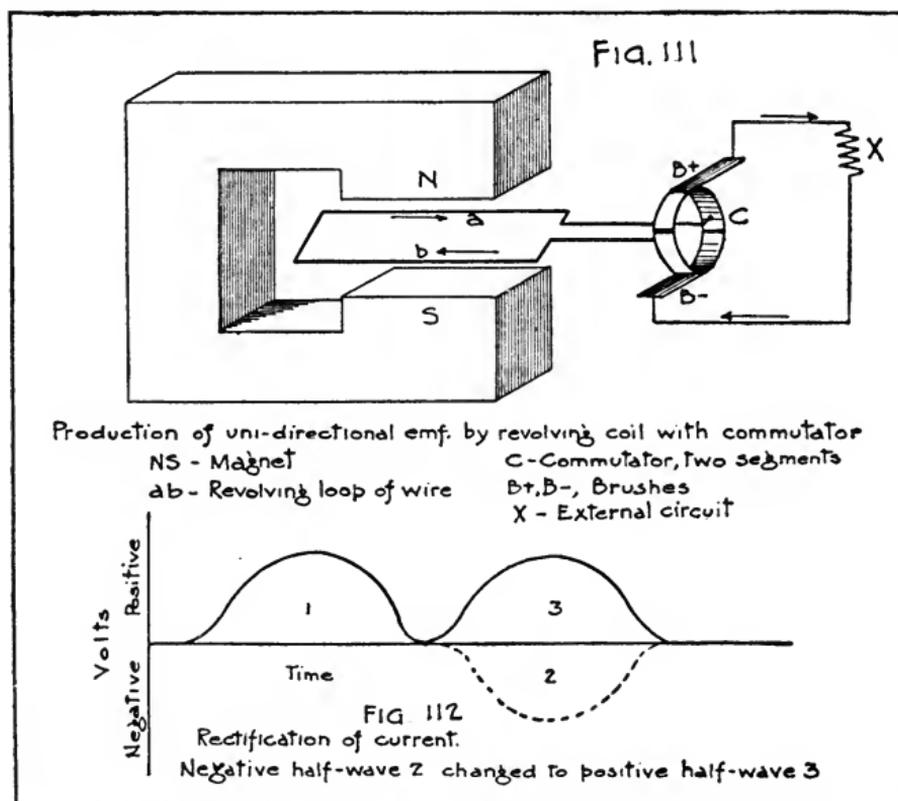
If an emf. curve similar to Fig. 95, p. 154, were plotted for this circuit, with time measured along the horizontal axis, and volts at any instant along the vertical axis, the result would be somewhat like Fig. 112. Instead of a positive and a negative half wave there would be two positive halves, the negative being rectified by means of the commutator.
