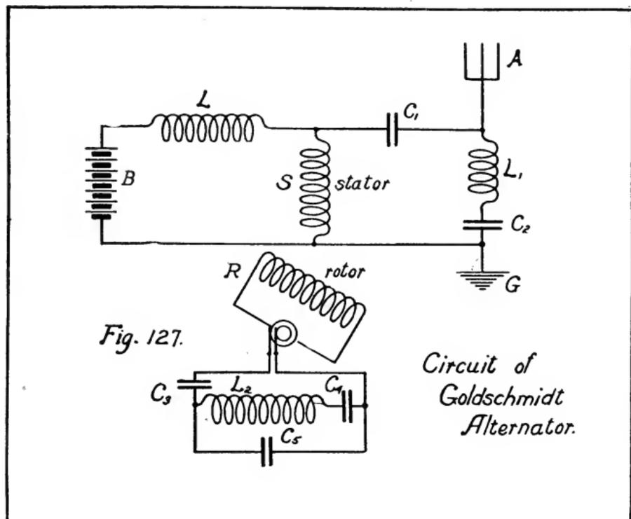
Without undertaking to give the proof here, it may be stated that when a rotor is revolved, and at the same time alternating currents are made to flow in the rotor at a frequency corresponding to the speed of rotation and to the number of poles, then, due to these currents, pulsations take place in the strength of the magnetic flux of the machine at double the frequency of the alternating currents.
