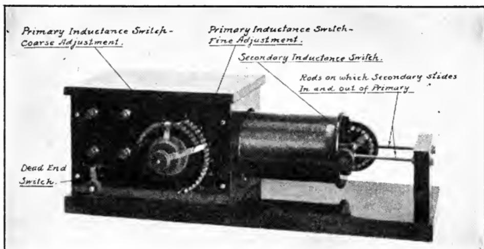
FIG. 249.—Receiving transformer.
