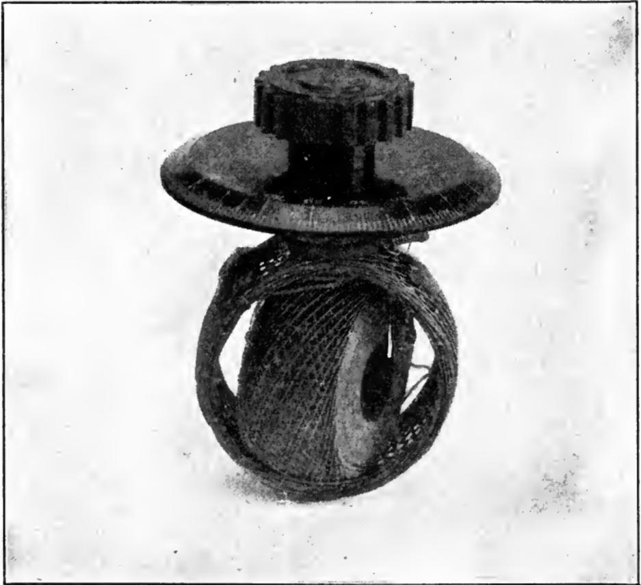
FIG. 250.—Lattice-wound variable coupling coil.
