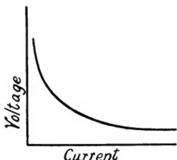
Fig. 223. Current-Voltage Characteristic of the D.C. Arc.
