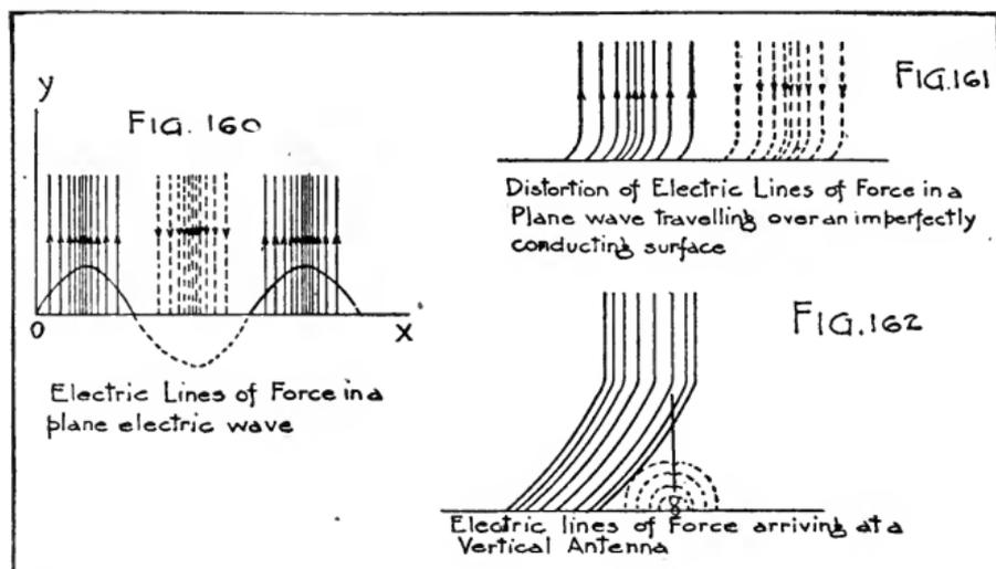
kinds, loops are formed and detached in the same general way. In some of them the distribution of the lines of force is such as to favor the production of more such loops than in others; this means that such an antenna will be a better radiator than the others.
