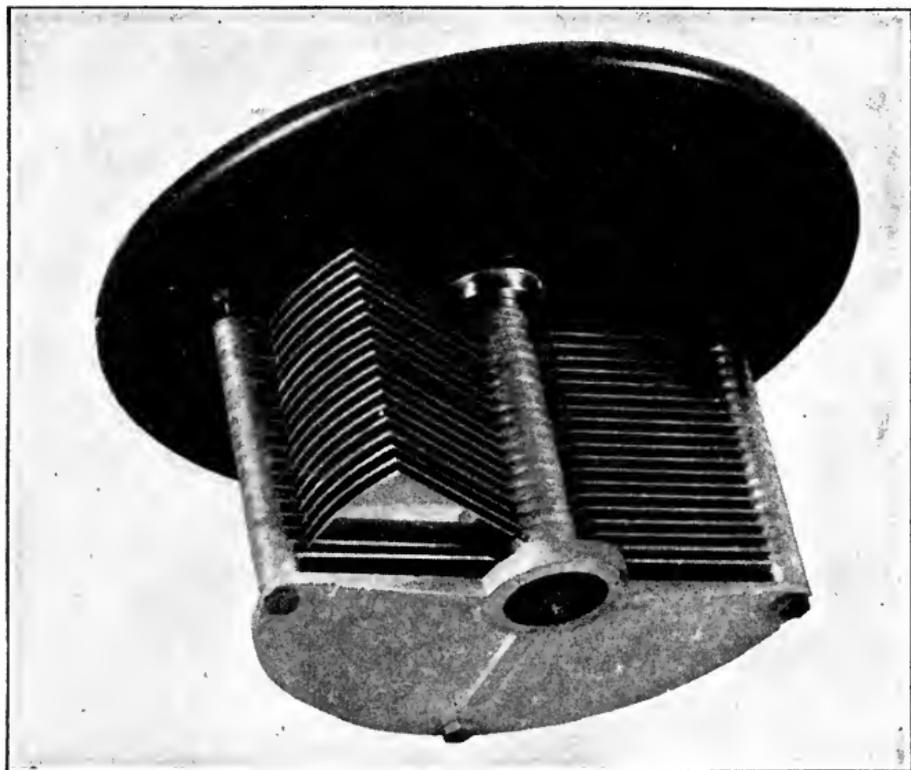
FIG. 251.—Rotary variable air condenser.
