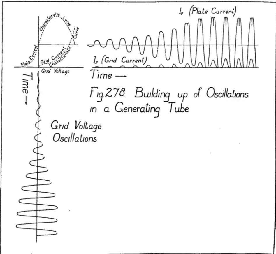
circuits in which the plate circuit is coupled back to the grid circuit in such a manner as to supply this small power to the grid and make the surplus power available for use in an external circuit in the form of continuous or undamped oscillations of any frequency from even less than one per second to 10,000,000 or more per second.
