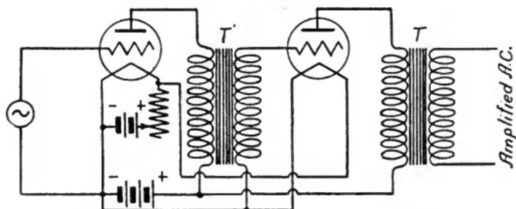
Fig.273. Connections for Cascade Amplification Transformer Coupling.
