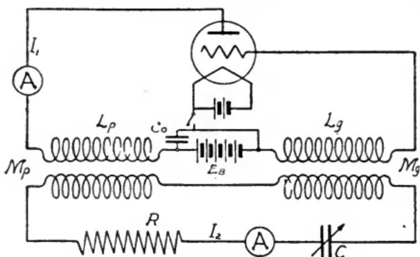
Fig. 279. Electron Tube Generating Circuit Inductive-Coupling.
