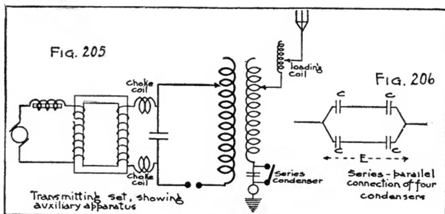
levers, changes simultaneously the adjustments on all three coils. From these coils are taken out taps over which three switch blades pass, adjusting all the inductances to approximately the values needed for the particular wave length desired, keeping the circuits in resonance and at the proper coupling. For fine adjustments an additional variable inductor may be provided in the primary and in the secondary.
