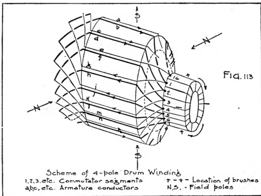
the brushes, which are thus seen to be alternately, one positive and the next negative, as we go around the commutator. If a machine having more than two sets of brushes is examined, it will be found that all the positive brushes are joined by a heavy conductor and all the negative brushes by another. Then one connection is made from the group of positive brushes to the external circuit, and one from all the negative brushes.
