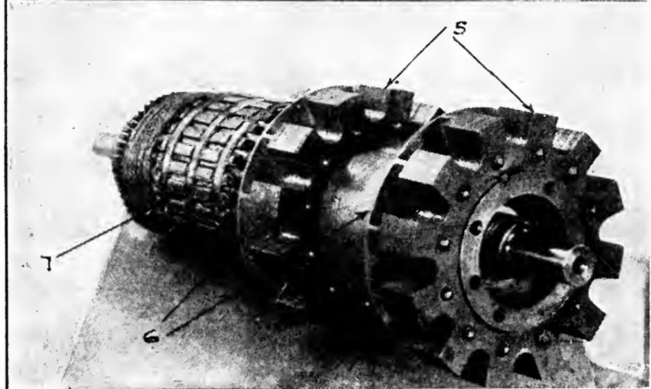
FIG. 124.—Inductor alternator type motor-generator set.
