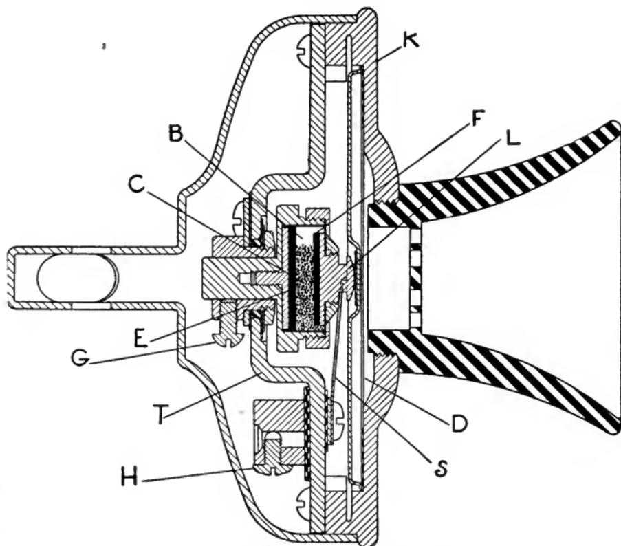
FIG. 93a.—Microphone transmitter.
