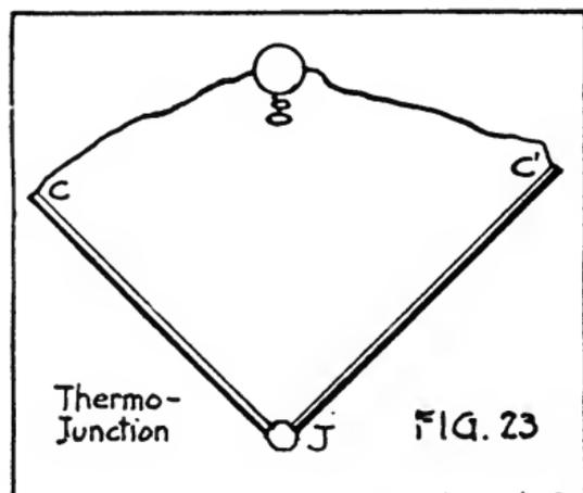
ends are connected by a copper wire through the galvanometer  $g$ . If the point of contact, or junction  $J$ , is heated to a temperature above that of  $C$  and  $C'$ , there will be a flow of current through the galvanometer. This is commonly explained by saying that at the junction  $J$ , heat energy is transformed into electrical energy, and this
