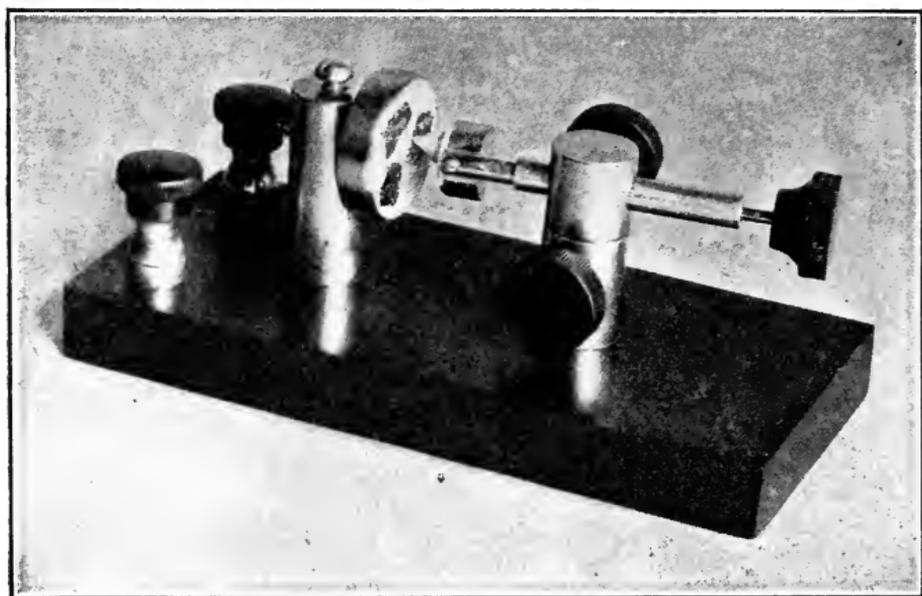
FIG. 245.—One method of mounting crystal detectors.
