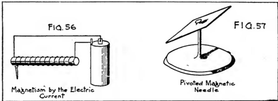
porary magnet or an "electromagnet." Examples of electromagnets are seen in induction coil and buzzer cores, in telegraph sounders and relays, and in telephone receivers. Electromagnets are very useful because the magnetism is so easily controlled by variations in the current strength. If the bars are of hardened steel, the magnetism due to the current remains after the current ceases and a permanent magnet is the result.
