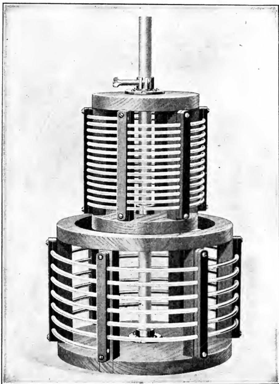
FIG. 197.—Double helix oscillation transformer; coils separated axially. cuitied except when actually needed in order to keep the resistance of the antenna circuit low.
