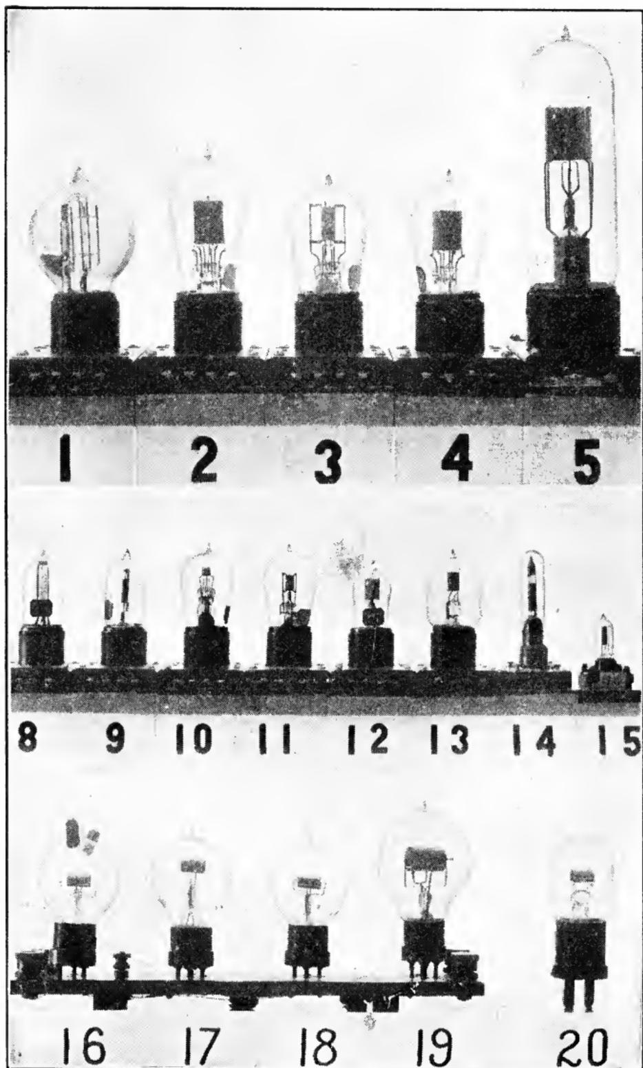
FIG. 265.—Practical forms of three-electrode electron tubes.
