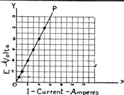
Fig. 20. Current-Voltage Relation in Simple Circuit
