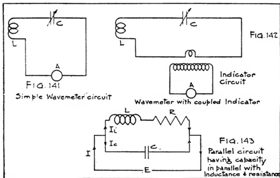
other will be variable. A hot-wire ammeter, thermo-junction, or other suitable device for measuring radio currents is inserted, either directly into the circuit (Fig. 141), or, better, is coupled electromagnetically to it, the coupling being made as loose (Sec. 119) as will permit of a suitable maximum deflection of the ammeter (Fig. 142).
