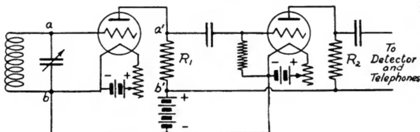
Fig.274. Resistance Coupled Amplifier.
