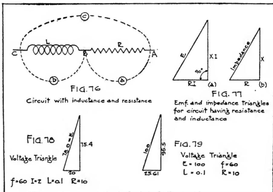
The effective applied emf.  $E$  in such a case is therefore related to the voltages  $RI$  and  $XI$  by the equation (relation between sides and hypotenuse of a right triangle),
