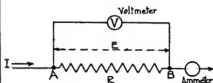
Fig. 19 Simple Circuit for Study of Ohm's Law
