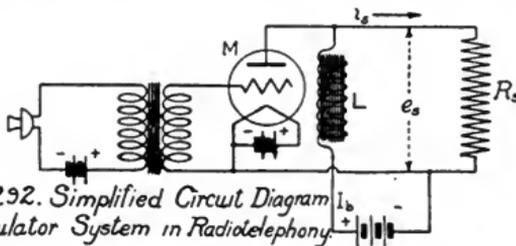
Fig.292. Simplified Circuit Diagram of Modulator System in Radiotelephony.
