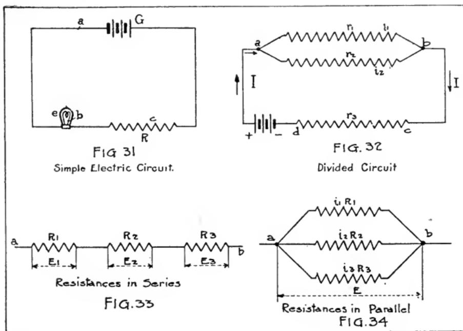
nected as shown in Fig. 34, so that only a part of the current passes through each resistance, they are said to be connected in "parallel" or "multiple." The voltage  $E$  between points  $a$  and  $b$  is the same over any branch. We may then write, from equation (11),
