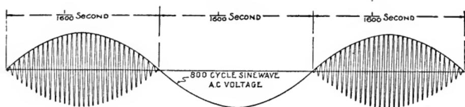
WAVE FORM OF OUTPUT CURRENT FROM TUBE TRANSMITTER HAVING
