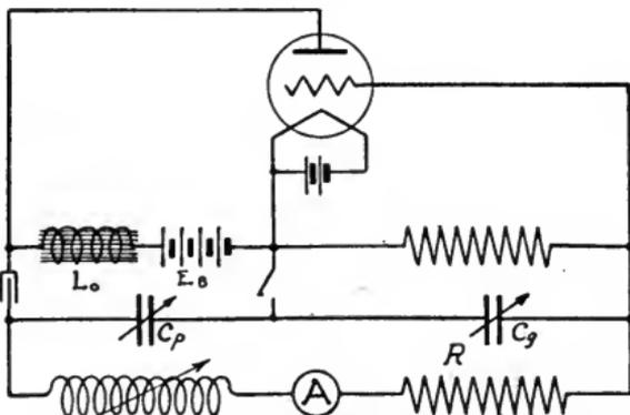
Fig. 281. Electron Tube Generating Circuit Direct Capacitive Coupling
