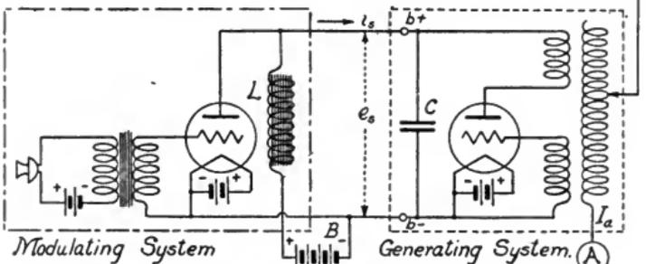
Fig.291 Circuit for Radiotelephone Transmitter, Modulation by Variation of Power Input of Generator Tube.
