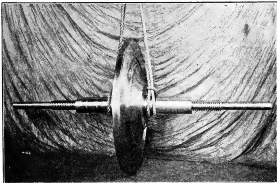
FIG. 126c.—Rotor of 200 kw. Alexanderson alternator.
