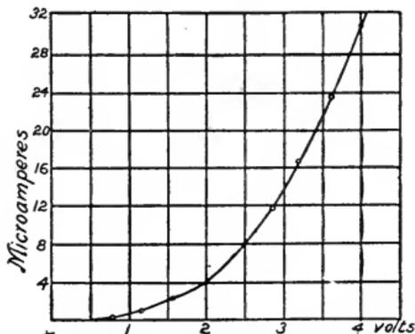
Fig. 247. Curve showing Current-Voltage Characteristic of Carborundum Detector.
