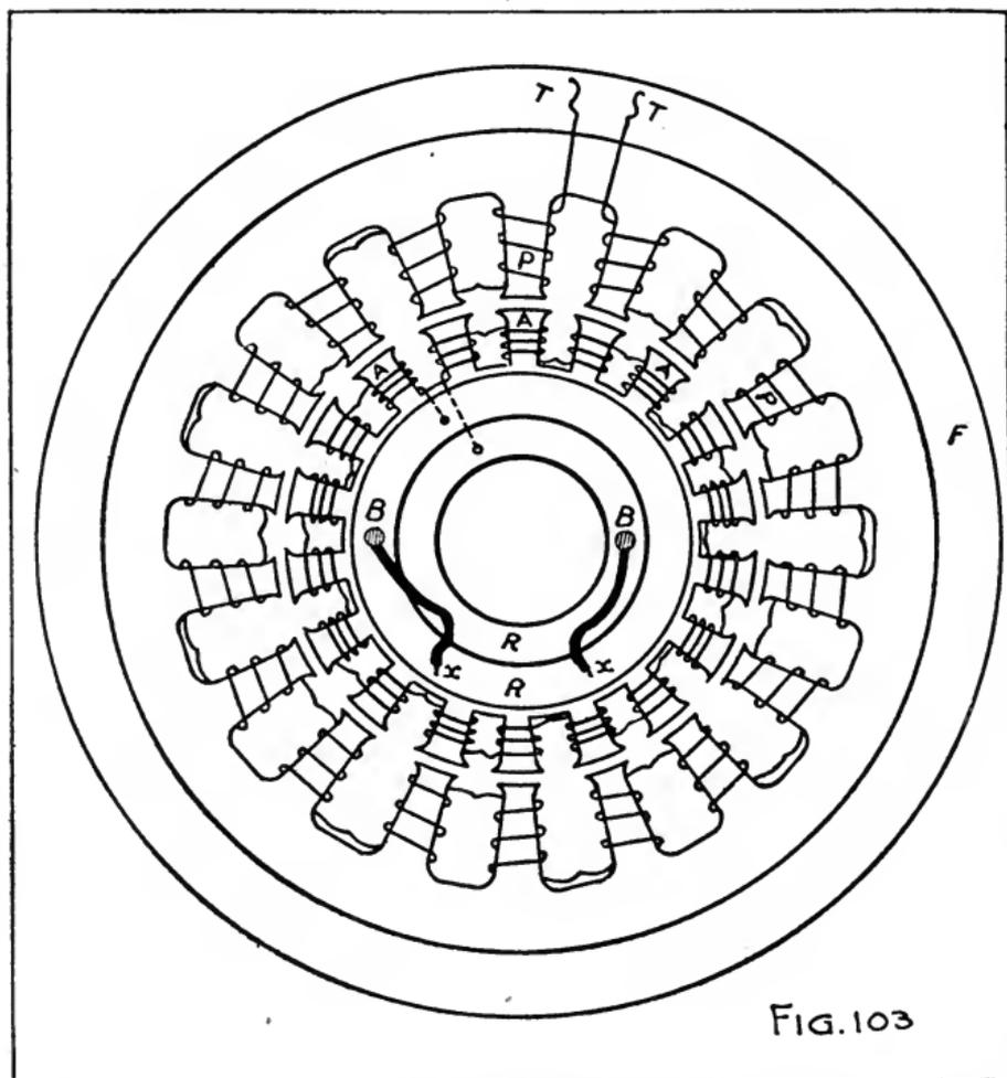
FIG 103.—Circuit diagram of revolving-armature alternator. A, armature; F, frame; P, poles; R, collector rings; B, brushes; TT, terminals of field circuit; XX, leads to external circuit.
