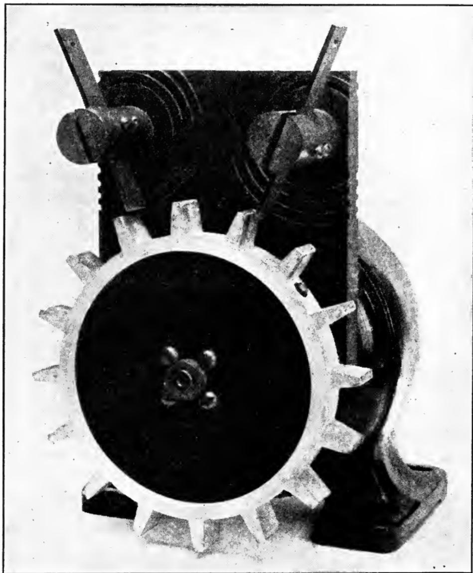
FIG. 186.—Nonsynchronous rotary gap.
