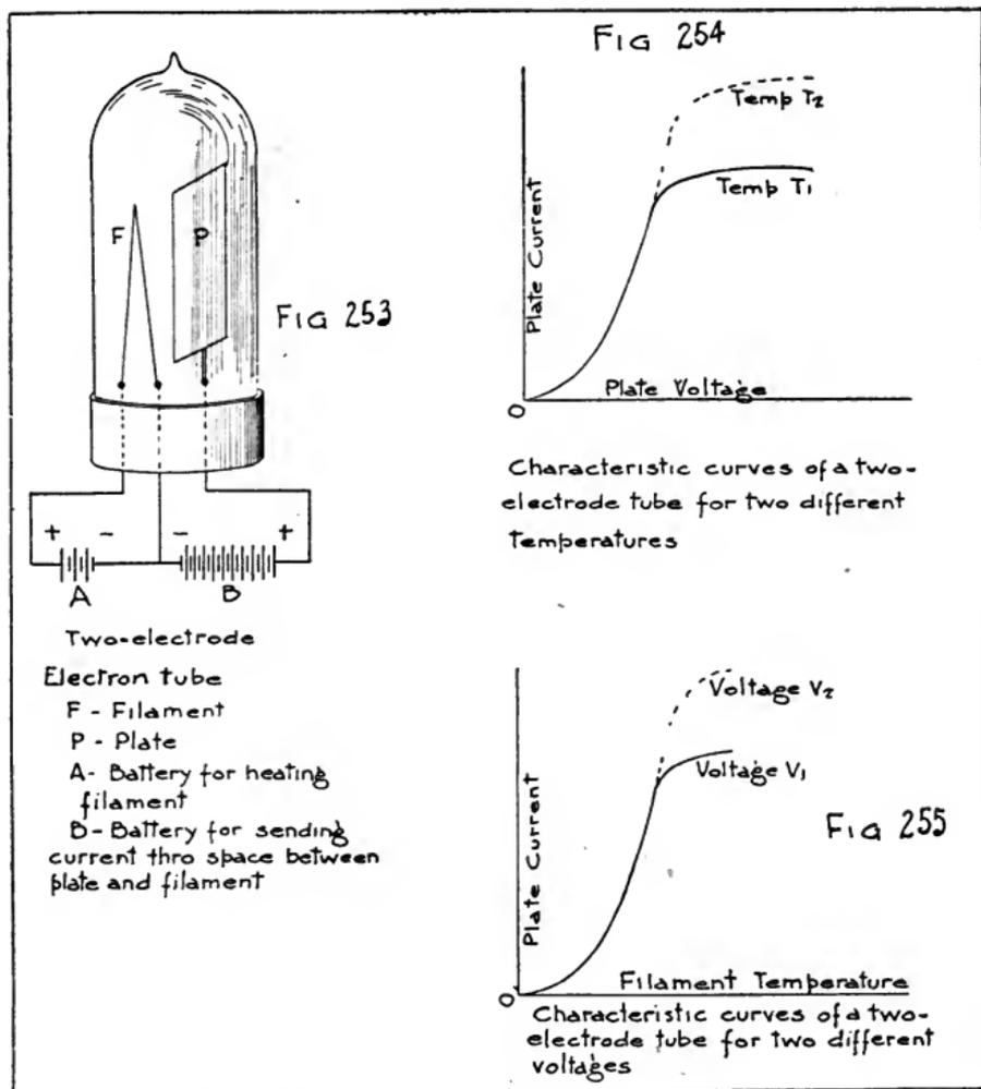
the opposite direction. Thus both of the parts of the disrupted atom become carriers of electricity and contribute to the flow of current through the gas. This action of a colliding electron upon an atom is called “ionization by collision,” and, on account of it, relatively large plate currents are obtained in electron tubes having a poor vacuum. The earlier tubes were of this
