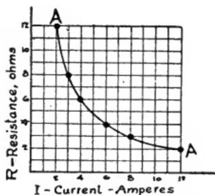
Fig. 21. Current-Resistance Relations in Simple Circuit
