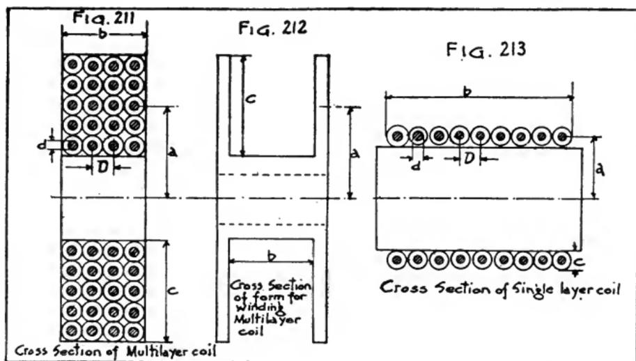
210. For wavemeters a multilayer coil is used, having wires insulated and close together, Figs. 211 and 212. For receiving coils the common form is a single layer of insulated wires, Fig. 213. The coils are supported or held together by some insulating material, and no iron is used in them.
