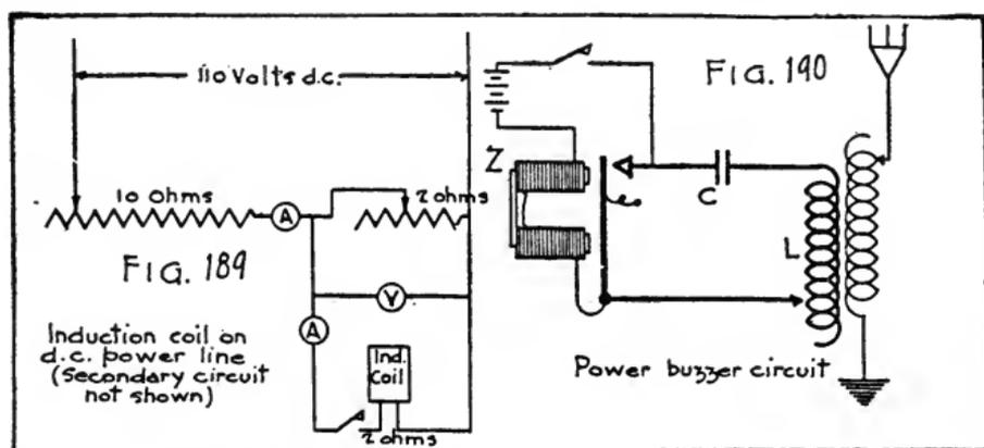
first attempt to signal, and the current will not be broken when the key is released. Of course, the method of inserting a rheostat is very wasteful, since the  $RI^2$  loss in the rheostat is large, much greater in fact, than the power actually used in the radio apparatus.
