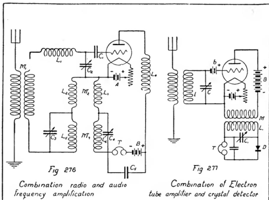
the audio frequency and of by-passing the radio frequencies. The radio-frequency variations in the plate current flow through the circuit  $PFL_3C_4C_5L_4$  and at the same time the audio-frequency variations flow through the circuit  $PFL_3L_6TBL_4$ . The audibility of weak signals received by this method is about 100 times the audibility obtained with a single tube connected in a simple detector circuit. On stronger signals the amplification is smaller.
