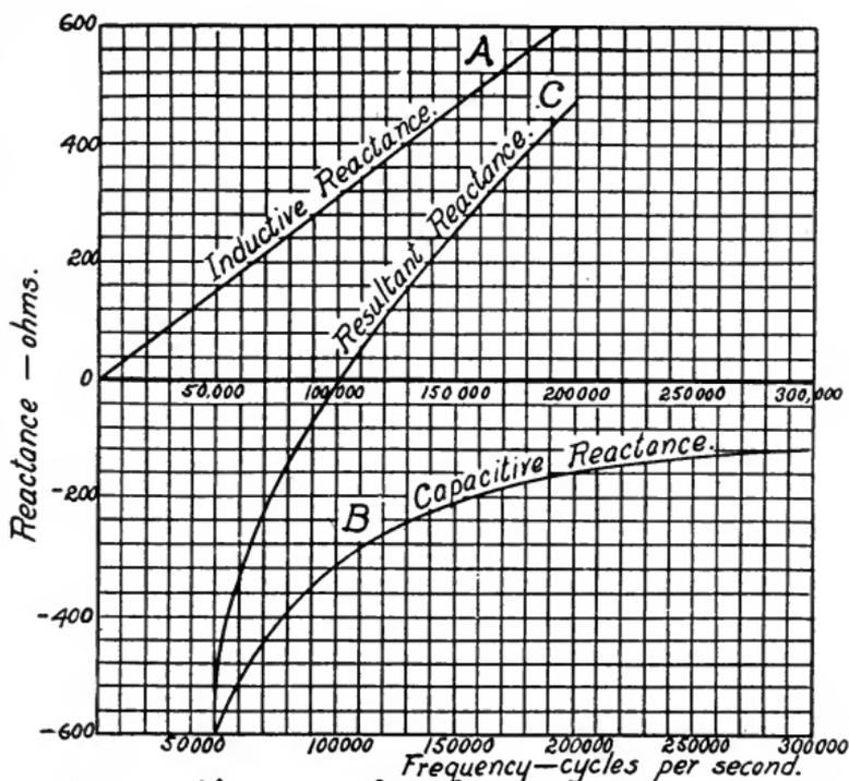
Fig. 138. Variation of reactance with Frequency.
