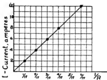
Fig. 22 Current-resistance Relations in Simple Circuit
