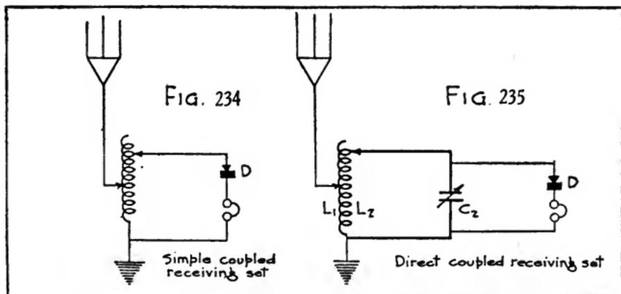
are detected by the crystal and telephone, and which are not in either oscillating circuit. The oscillations are not damped thereby, and sharp tuning is obtained.
