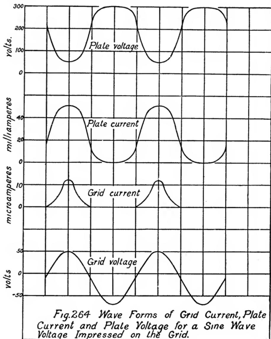
In power applications of tubes the oscillation characteristic is restricted to certain regions. The plate current drawn from the plate battery by a tube is given by the average tube current, and the plate battery voltage is approximately the average
