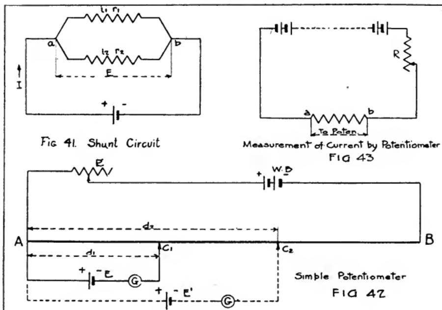
The currents in the two branches are inversely proportional to the resistances of their respective paths. This relation is called the "shunt law." In other words, it means that the branch of lower resistance carries the larger current, and the branch of higher resistance carries the smaller current.
