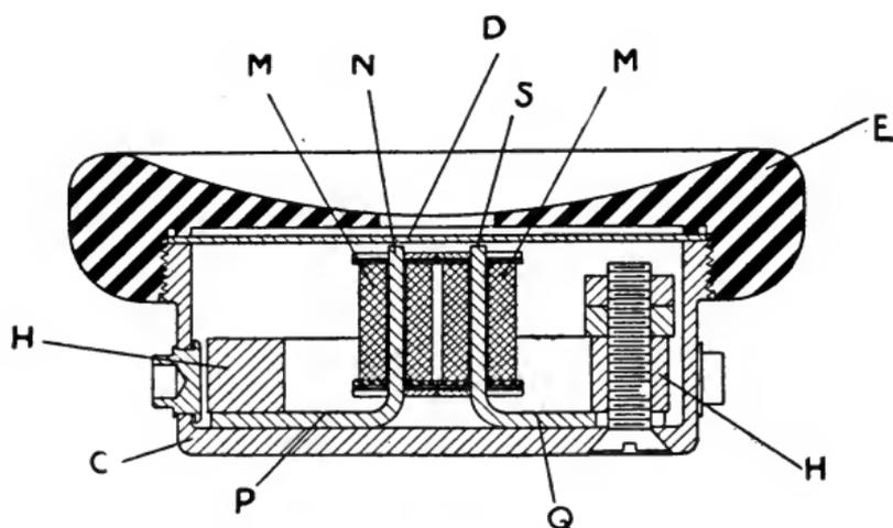
FIG. 93b.—Watch case telephone receiver.
