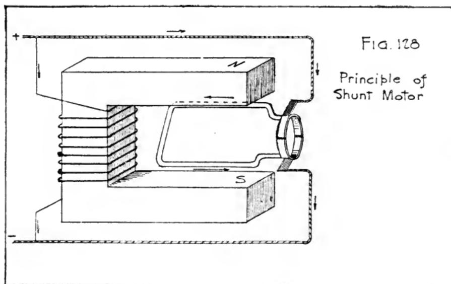
to make the rotation continuous by making the proper connection to the conductors as they come into place.
