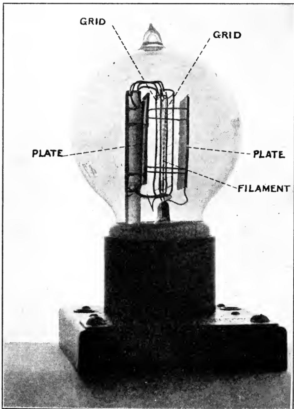
FIG. 256.—Construction of the three-electrode electron tube.
