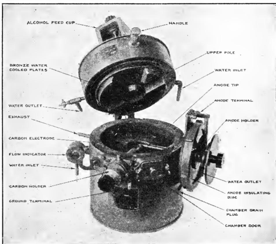
FIG. 227.—Interior of 2-kw. Federal arc converter.
