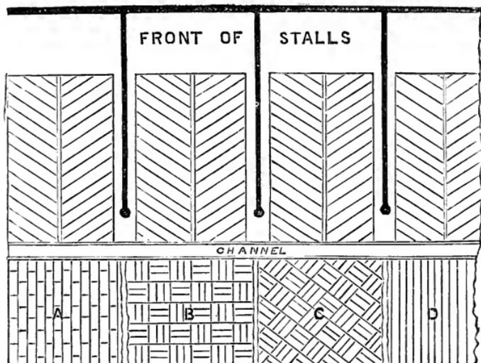
Stalls with concrete floors, the grooves of which incline backwards and inwards to the middle groove. A B C D, different ways of furrowing the pavement behind the stalls.
