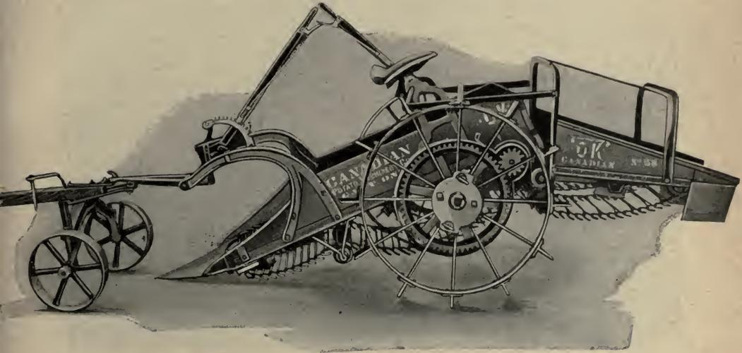
Fig. 26. Side view of a steel-nose potato-digger.
