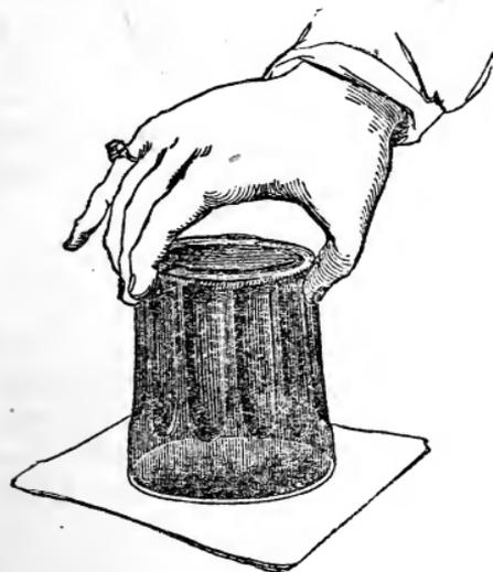
That the air *does* exert a definite pressure, in consequence of its weight, may be easily proved by any one with the above simple apparatus—only a tumbler and a sheet of paper. Fill a tumbler quite full of water, and carefully draw over its top a sheet of clean letter paper, and be careful to see that there are no
