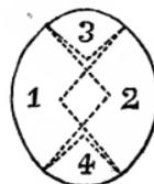
The cabinet-maker must first find the centre of the circle, and strike another circle, half the diameter of the first, and having the same centre. Then cut the whole into four parts, by means of two lines drawn at right angles to each other; then cut along the inner circle, and put the pieces together as in the above diagram.
