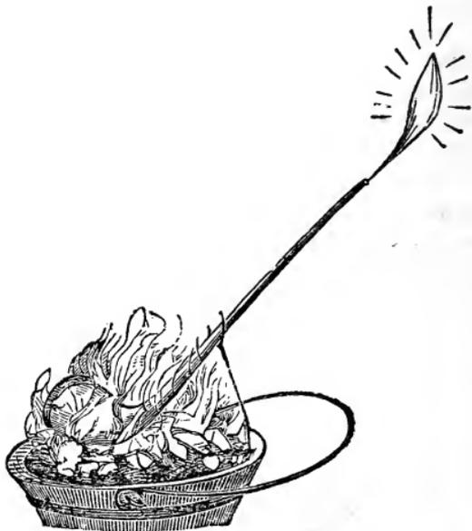
a piece of coke will be found inside; this is the excess of carbon over the hydrogen contained in the coal, for all the hydrogen will combine with carbon at a high temperature, and make what are called hydro-carbons—a series of substances containing both these elemental forms of matter.
