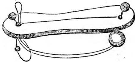
The knots beneath the wood prevent the loops being pulled through by the pellets.
