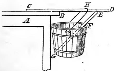
Place the handle of the bucket on the stick in such a manner that it may rest on it in an inclined position, as  $H I$ , and let the middle of the bucket be a little within the edge of the table; to keep this apparatus properly in its situation, place another stick,  $E F G$ , with the end resting against the bucket at the bottom, its middle,  $F$ , resting on the
