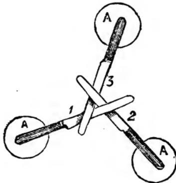
No. 2, and that over No. 3, which rests on No. 1. The bridge so made will be self-supported.
