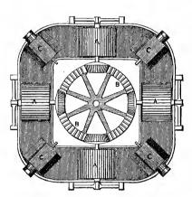
Fig. 49.—Beating Engine with Four Beater Rolls.
