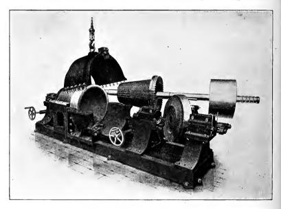
Fig. 54.—Working Parts of a Modern Refining Engine.
