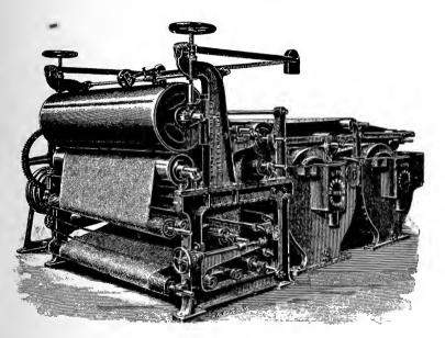
Fig. 42.—Double Cylinder Board Machine.
