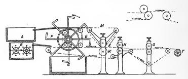
Fig. 5.—The Improved Paper Machine of A.D. 1810.
