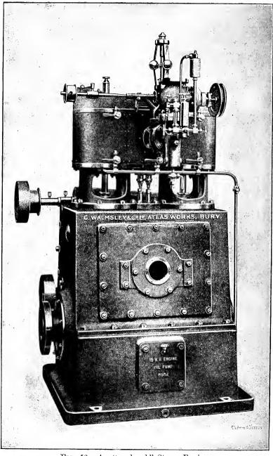
Fig. 56.—An "enclosed" Steam Engine.
