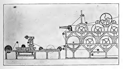
Fig. 15.—Apparatus for Sizing Paper in continuous Rolls.
