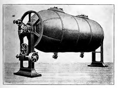
Fig. 26.—A Cylindrical Digester for Boiling Fibre.
