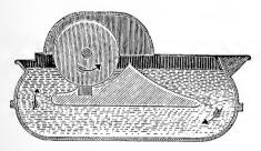
Fig. 51.—Section of Umpherston Beating Engine.
