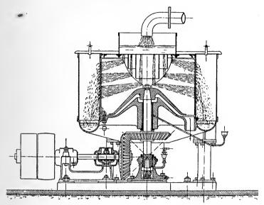
Fig. 32.—Section of Centrifugal Screen for Wood Pulp.
