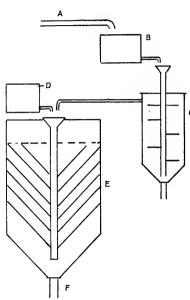
Fig. 55.—Conventional Diagram of a Water Softening Plant.
