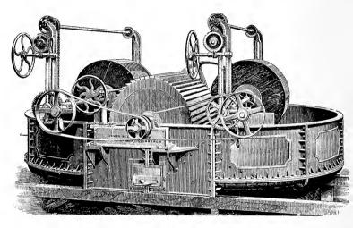
Fig. 11.—A Breaking and Washing Engine.
