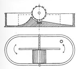
Fig. 48.—Plan and Sectional Elevation of a "Hollander."
