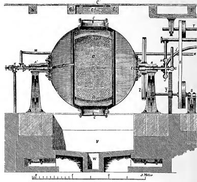
Fig. 10.—View of a Rag Boiler, showing connections.
