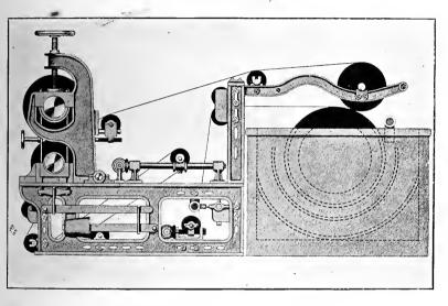
Fig. 41.—Section of Wet Press, or Board Machine.
