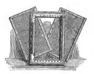
Fig. 14.—The Hand Mould showing Frame and Deckle.
