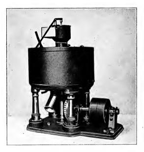
Fig. 31.—Centrifugal Screen for Wood Pulp.
