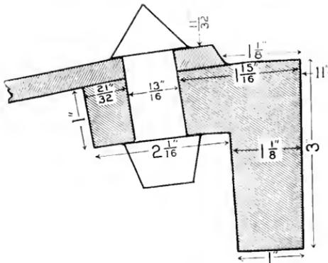
FIG. 5.—SECTION OF MANHOLE FRAME.
