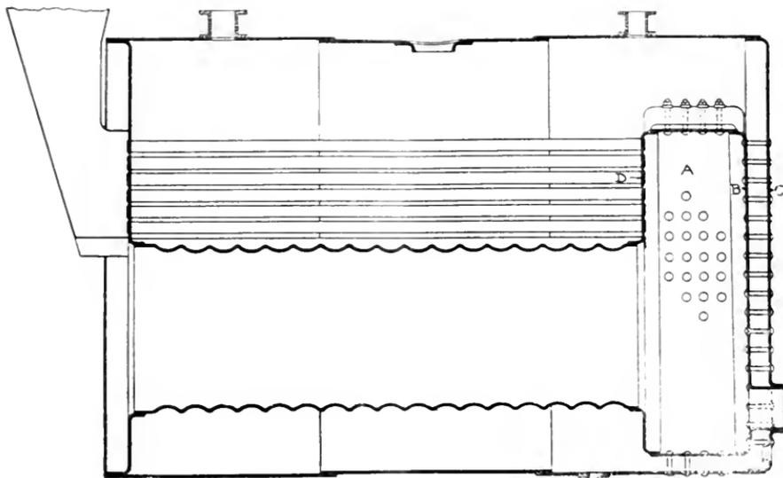
FIG. 2. SECTION OF BOILER.
