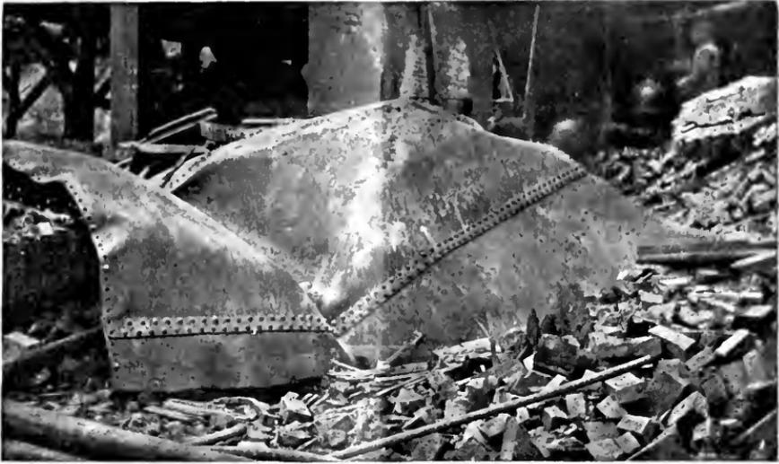
FIG. 3.—SHELL OF EXPLODED BOILER.
