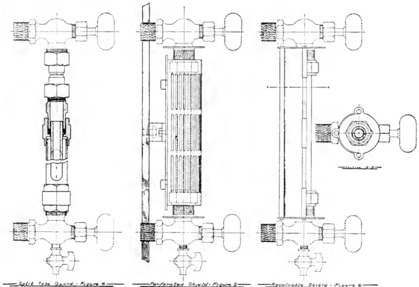
FIGS. 4, 5, AND 6.—SPLIT TUBE, PERFORATED AND REVOLVABLE GUARDS.
