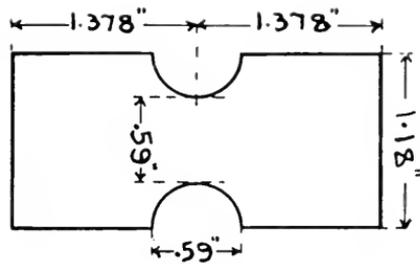
FIG. 7. IMPACT TEST SPECIMEN.
