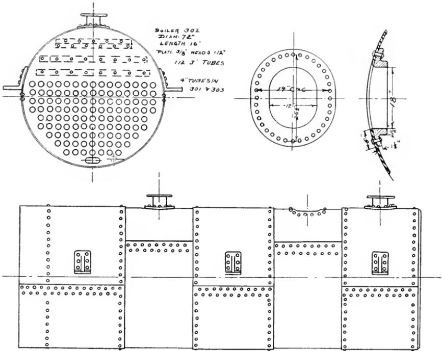
FIG. 1. DETAILS OF BOILERS 301, 302, AND 303.
