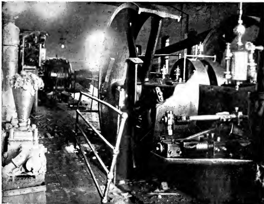
FIG. 1.—SHOWING THE BROKEN WHEEL AND GOVERNOR.
