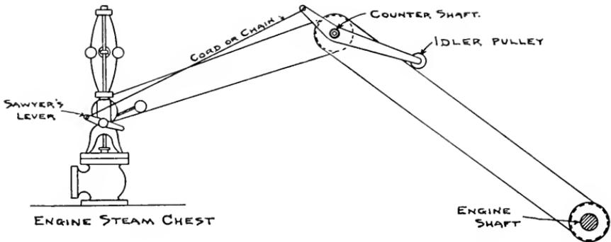
FIG. 1.—SAFETY DEVICE FOR A COUNTERSHAFT DRIVEN GOVERNOR.
