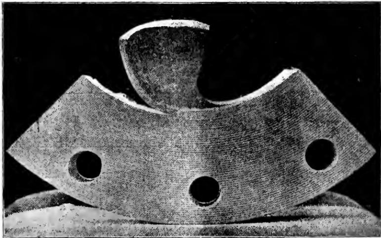
FIG. 1.—WELDED STEAM PIPE, SHOWING DEFECTIVE WELD.
