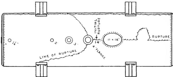
FIG. 6.—TOP VIEW OF BOILER, SHOWING INITIAL RUPTURE.
