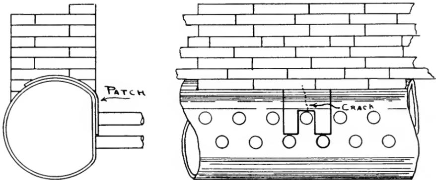
FIG. 2. PATCH BRICKED AND CEMENTED IN PLACE.
