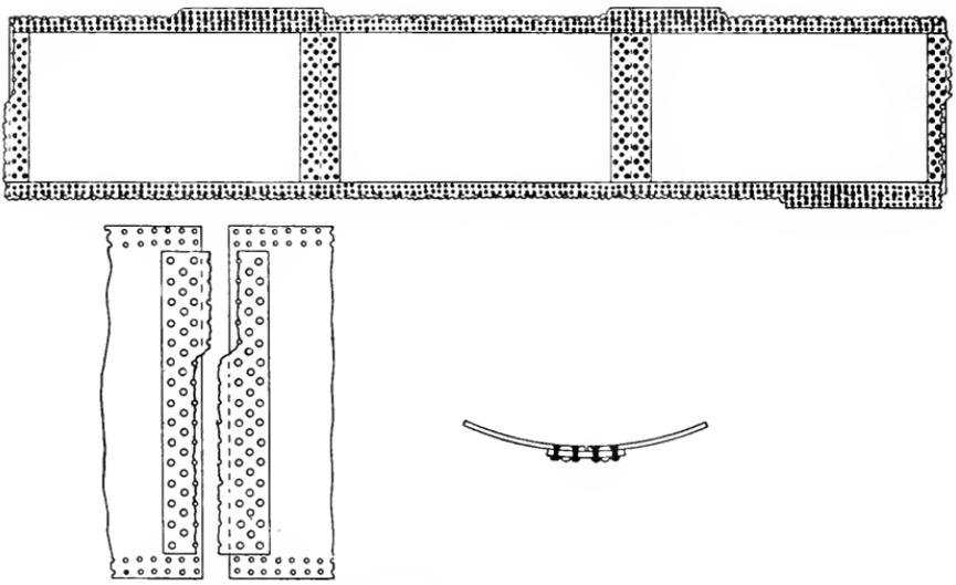
FIG. 4. DETAILS OF COURSE WHICH FAILED.
