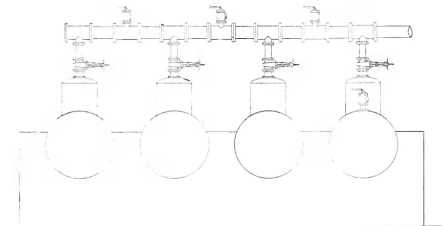
UNSAFE ARRANGEMENT OF STEAM PIPES.
