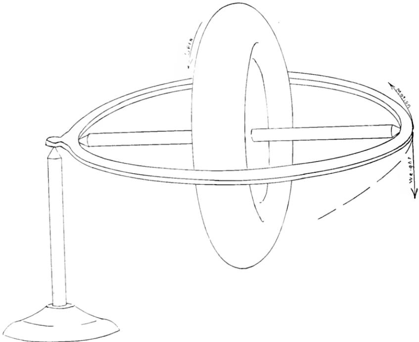
FIG. 2. SIMPLE GYROSCOPE.
