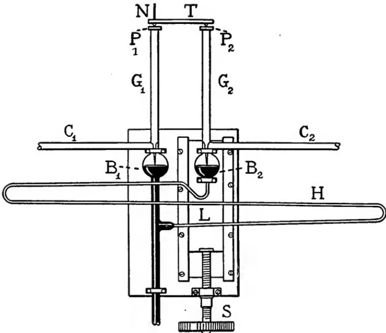
FIG. 2. — MANOMETER No. 3. (FOR THE LOWEST PRESSURES.)
