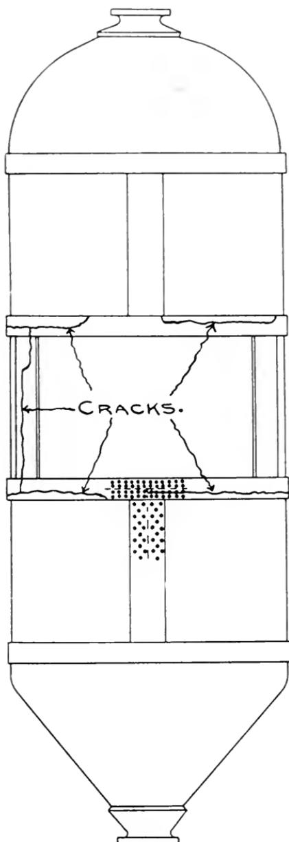
FIG. 3. ELEVATION OF DIGESTER SHOWING LOCATION OF THE LINES OF FAILURE.
