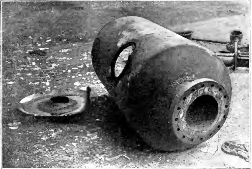
FIG. 4. THE WRECKED SEPARATOR.
