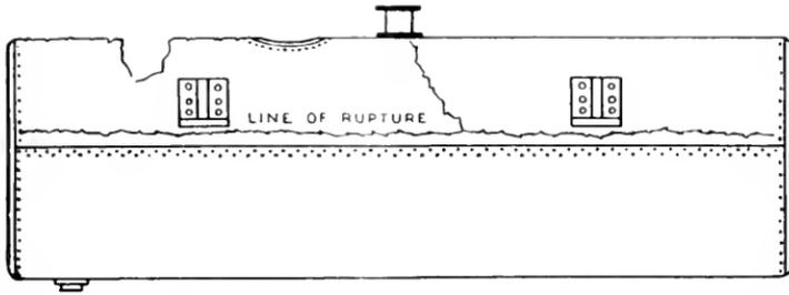
FIG. 8.—LEFT-HAND SIDE OF BOILER, SHOWING LINES OF RUPTURE.
