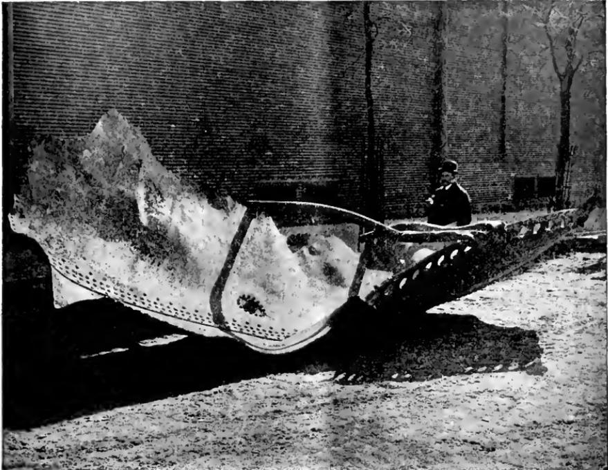
FIG. 5.—ONE OF THE RUPTURED DRUMS.
