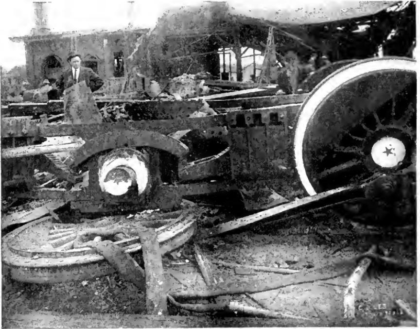
FIG. 3. DRIVER BLOWN FROM AXLE.
