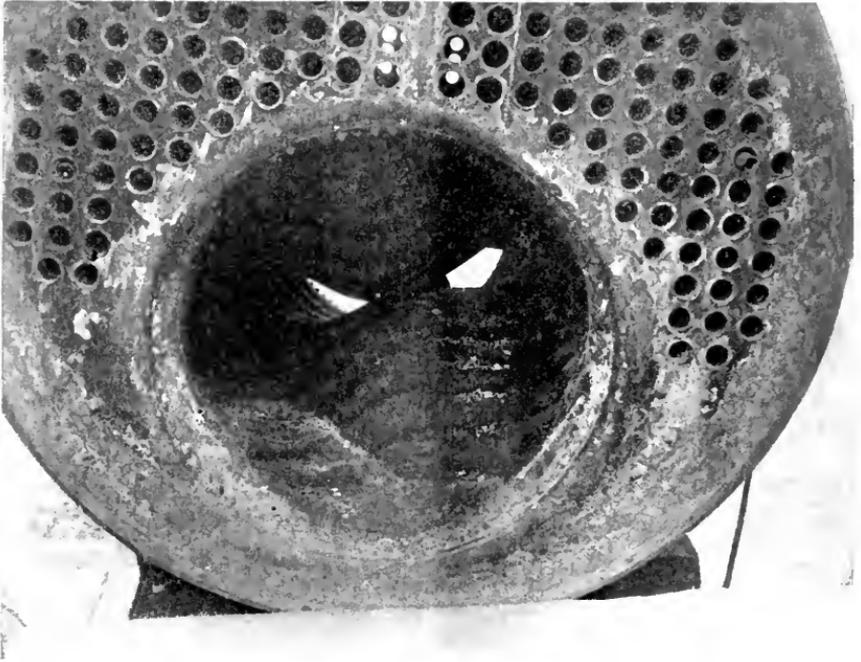
FIG. 2. THE COLLAPSED FURNACE.
