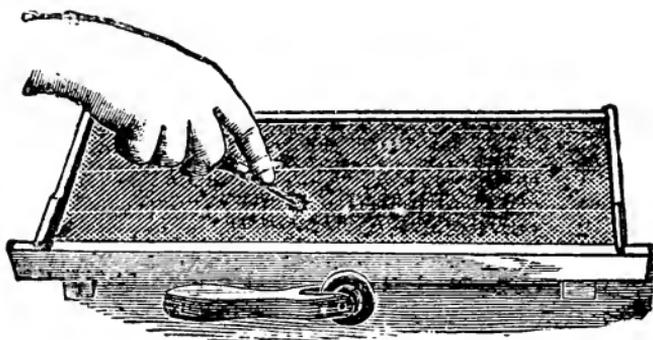
Fig. 40.—SPUR WIRE EMBEDDER IN USE.
