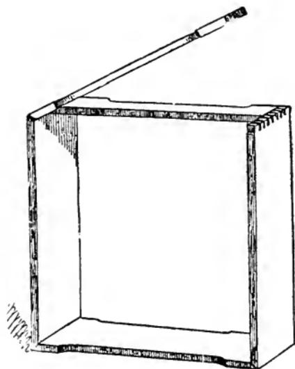
Fig. 36.—ONE PIECE SECTION BOX, PARTLY FOLDED.
