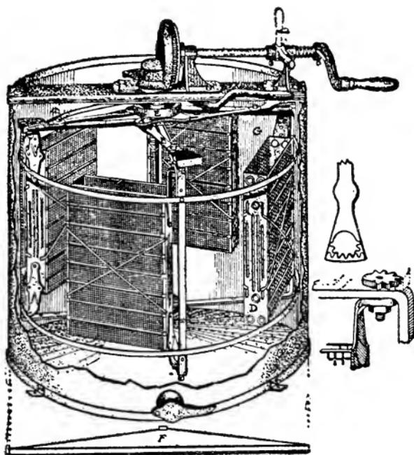
Fig. 43.—“ AUTOMATIC ” FOUR-COMB REVERSIBLE EXTRACTOR.
