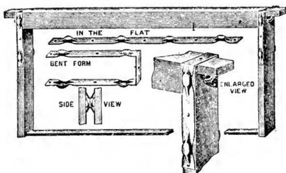
Fig. 33.—METAL-SPACED FRAME.
