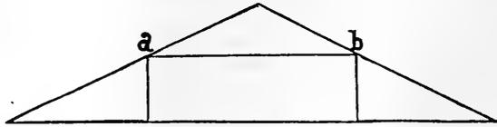
Fig. 93.—Trussing with Straining Beam between the Posts.
