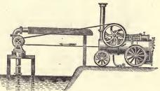
FIXED CENTRIFUGAL PUMPING MACHINERY. This class of Pump is readily fixed on a wood staging in a river or canal, or over a well.
