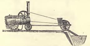
PORTABLE CENTRIFUGAL PUMPING MACHINERY. This class of Pump is especially useful in all cases where it is necessary to frequently remove the machinery.
