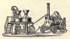
CORN GRINDING MILLS, With one, two, or more pairs of Stones, and driven by Portable or Stationary Steam Engines. Also complete Wheat-cleaning and Flour-dressing Machinery.
