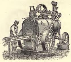
PATENT PORTABLE STEAM ENGINE, For burning straw, reeds, cotton and maize stalks, jungle grass, brushwood, and other vegetable refuse, as well as coal and wood.
