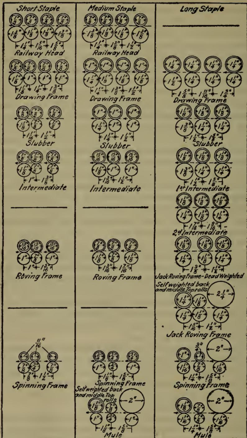
intended to work long-staple cotton, in order that the centers of the rolls may be brought near enough together. The diagram given in the accompanying illustration shows the settings and diameters of rolls for different kinds of cotton. These settings will vary, however, according to conditions.
