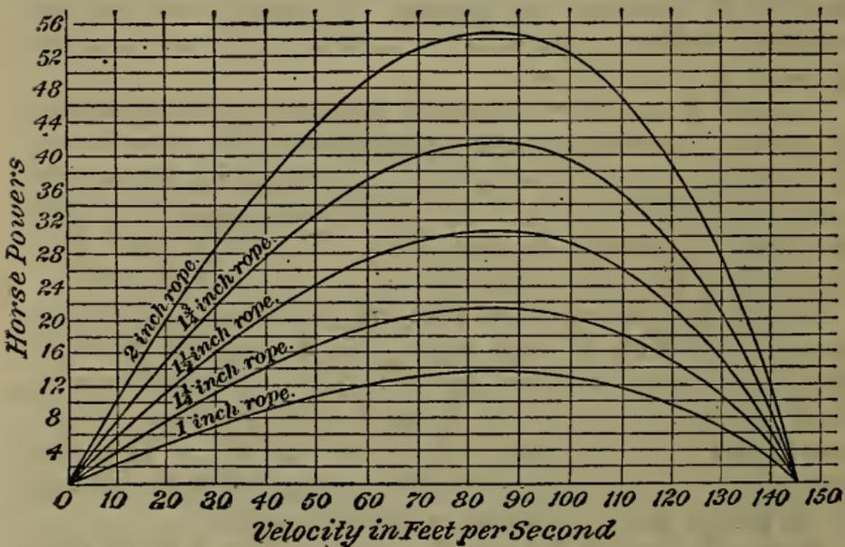
The accompanying figure shows the horsepower transmitted by 1-in.,  $1\frac{1}{4}$ -in.,  $1\frac{1}{2}$ -in.,  $1\frac{3}{4}$ -in., and 2-in. ropes for various velocities.
