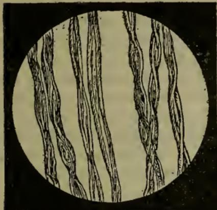
Ignoring the removable foreign matter contained in raw cotton, such as sand and other mineral substances, leaf, and pieces of boll, or stalk, it is found to be composed of from 87 to 90% of cellulose, permeated by about 1% or less of
