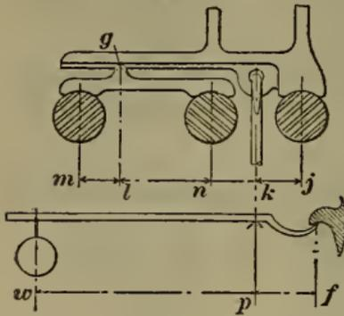
*Lever weighting*, which is a form of dead weighting, consists of exerting pressure by means of a weight acting through a lever. By this means a smaller weight may be used and the same pressure obtained as when a larger weight is employed in the system of dead weighting.
