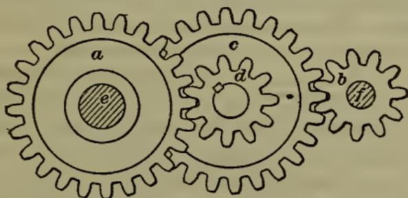
on the driving gear or gears multiplied together and by the speed of the first driver equals the number of teeth on the driven gear or gears times the speed of the last driven gear. Speeds and sizes of gears, like pulleys, should be treated by proportion. Intermediate gears should not be used when finding speeds or sizes of gears.
