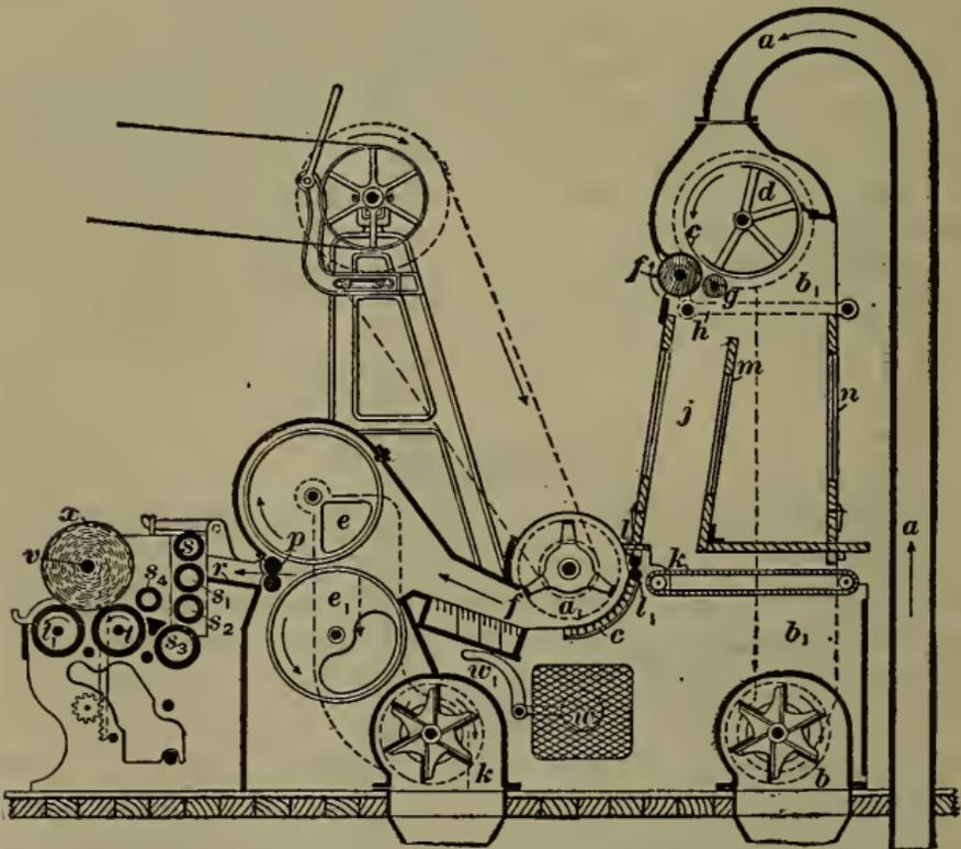
separate the tufts of cotton so that they may be more easily manipulated at the next process; (3) to form the cotton into a layer and wind it on a roll in a cylindrical form known as a *lap*.
