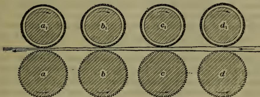
The circumferential speed of the upper and lower roll in each pair, is the same; that is, a point on the surface of  $d$  moves at the same speed as a point on the surface of  $d_1$ , because  $d_1$  is driven by frictional contact with  $d$ . The same remarks apply to any other pair in the series.
