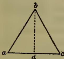
A *triangle* is a plane figure bounded by three straight lines and having three angles. The altitude of a triangle is the distance from its apex to base measured perpendicularly to the base. In the triangle *abc*, the dotted line *bd* represents the altitude, and the line *ac* the base, of the triangle.<sup>#</sup>
