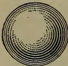
**Rule.**—To find the surface area of a sphere, square the diameter and multiply the result by 3.1416.
