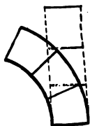
FIG. 15. — Illustrating resistance to bending when the supporting tissue is on the outside of the stem, as in corn. One side must be shortened and the other stretched.
