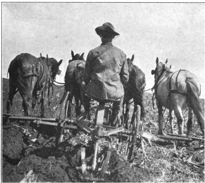
FIG. 45. — A combined lister and drill. The land is not plowed in preparation for listing.
