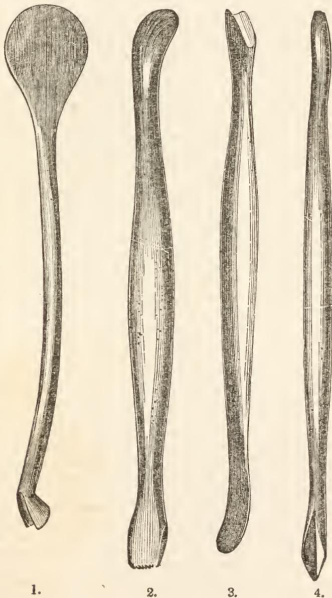
*Modelling Tools.*—No. 1 is termed the rose-stick, the thin flat end being used for forming the leaves of roses out of modelling wax by flattening a piece of it on a table until it is of the required form and size; the other end is used for fluting and making borders.
