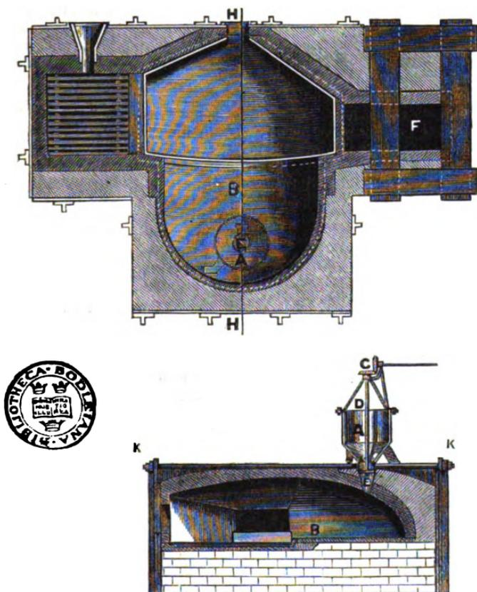
Fig. 204. Mr. Clay's Oven and Puddling Furnace. A. The hopper to contain the charge of ore and coal. B. Preparatory oven or bed. C. Wheels to regulate the supply of the mixture. D. Shaft to which the perforated bottom  $\times$  is attached. F. Chimney, nearly double in area to that which is required on the old system of puddling. The sectional drawing,  $\times \times$ , is taken through  $\times \times$ .
