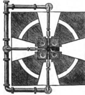
Fig. 202. Ground-plan, showing the disposition of the tuyere pipes.
