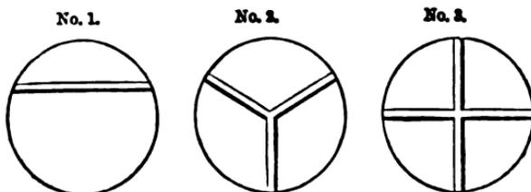
Fig. 34. Various Methods of dividing a Coal Pit Shaft for Ventilation and drawing Coals, &c.
