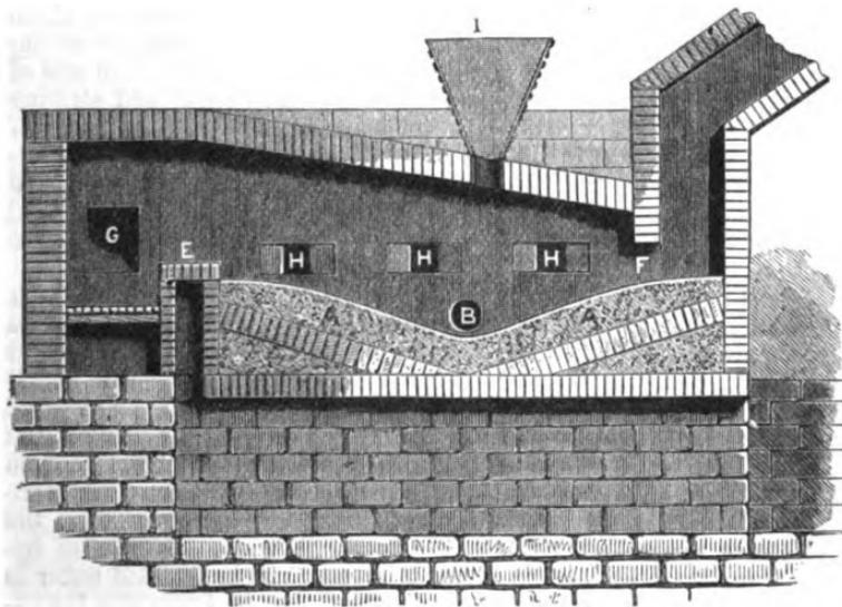
Fig. 155. Section of the Reverberatory Furnace used for roasting and smelting Galena. A. The hearth or sole of the furnace. B. Tap hole. X. The bridge which separates the fire from the hearth upon which the ore is placed. F. The flue. c. Hole through which the fuel is placed in the fire below. h, h, h. Openings, closed by sliding iron plates, for the admission of air. 1. The hopper by which the ore is passed into the furnace.
