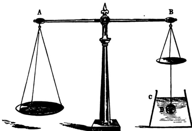
Fig. 123. Mode of taking the Specific Gravity of a Sovereign. A B. The delicate balance. a. Vessel containing distilled water. D. The sovereign suspended by a horse-hair.
