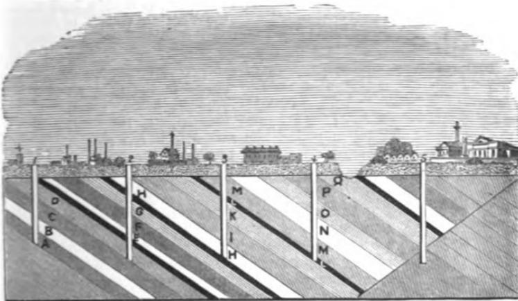
Fig. 27. Mode of "Boring" for Coal.
