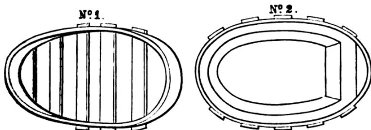
Fig. 135. No. 1. The iron rams of the test. No. 2. The iron frame rammed hard with damp bone-earth and dried, called the test or cupel.
