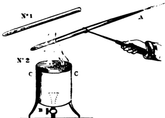
Fig. 157. No. 1. Tube closed at one end, containing tartarate of lead. No. 2. Drawn, closed and drawn out to a capillary tube at A, and held over the mixed gas and air flame obtained by allowing coal gas to escape gently from the cock *x* into the iron cylinder *c*, open at the bottom, and covered with wire gauze at the top, where the mixture of gas and air burns.
