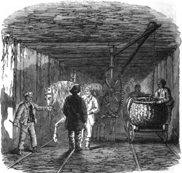
Fig. 48. The Crane Hoister.
