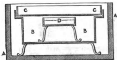
Fig. 186. Apparatus for freezing Mercury.
