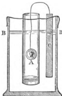
Fig. 135. De la Rive's Process of Gilding. A. Lamp chimney closed at the lower end with bladder containing the solution of chloride of gold; it is supported so that the bladder end does not touch the bottom of the vessel, the outer vessel, containing the acidulated water. C. The plate of zinc attached by a wire to the article which is to be gilt.
