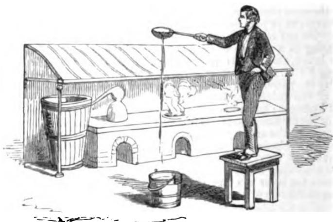
Fig. 266. Process of granulating Zinc by pouring it from a height into a pail of cold water.
