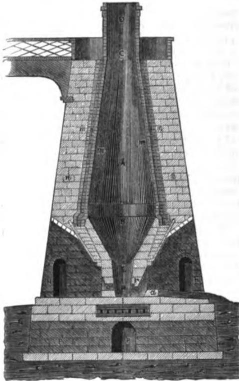
Fig. 301. Section of a Blast Furnace (Muespratt).
