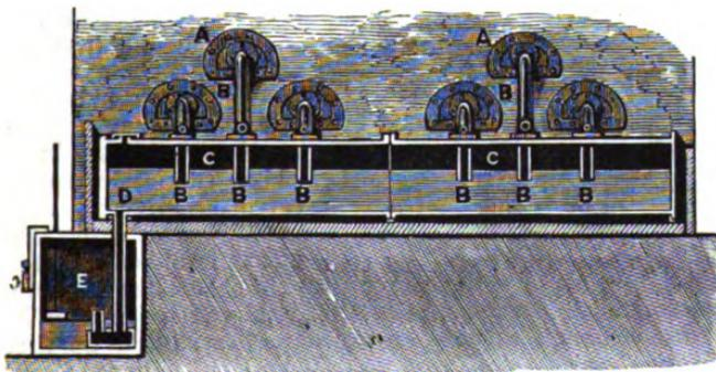
Fig. 135. A, A. The retorts. The pipes leading from the retorts marked B. C. C. The condenser of cast iron nearly filled with water into which the pipes B dip. D. Pipe through which the condensed mercury falls into the iron chest E, which is provided with a float and rod to indicate the quantity of condensed mercury.
