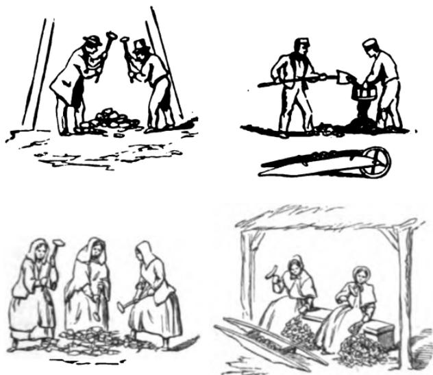
Fig. 166. Ragging, Spalling, Liddling, and Cobbing the Copper Ore.
