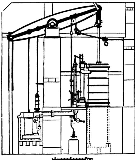
Fig. 199. A Cornish Pumping Steam-engine. (Bourne.)
