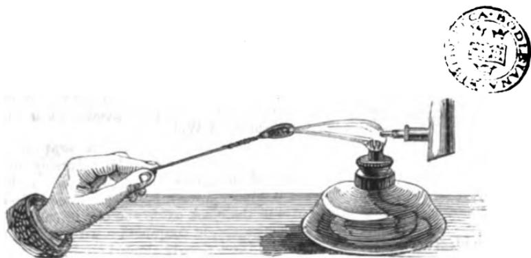
Fig. 245. Manganese Compound, fused on a loop of platinum wire with phosphate of soda and ammonia, which is sometimes called microcosmic salt.
