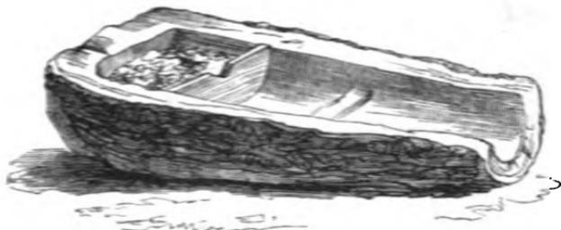
Fig. 113. Bade Washing Cradle, consisting of the Half of the Trunk of a Hollow Tree.
