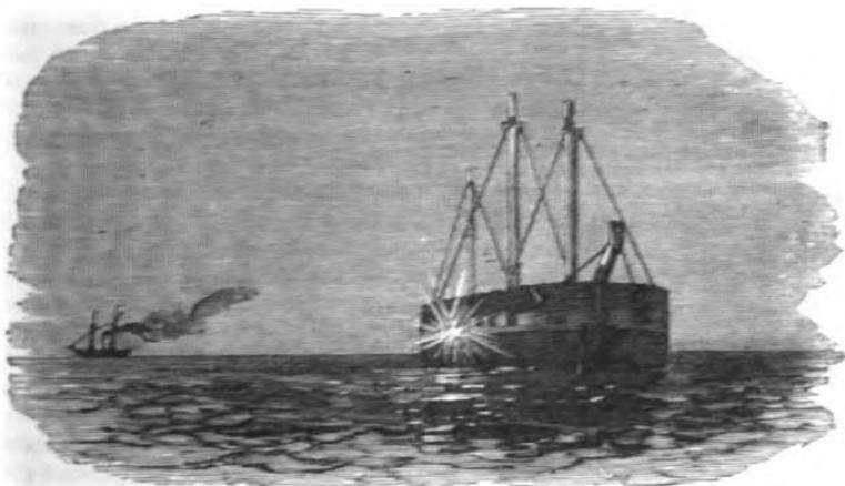
Fig. 36. Whitworth Gun and the Iron-plated Floating Battery, the *Trusty*, showing the flash of light when the shot struck the side.
