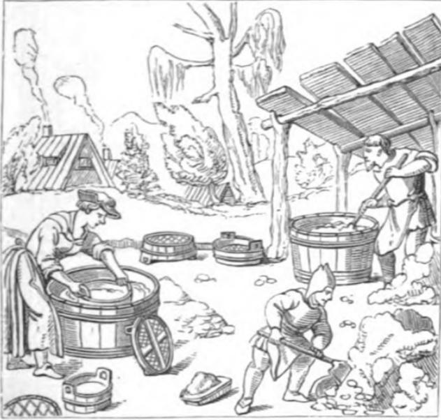
Fig. 151. Old Method of sorting and cleansing Mineral Ores. (Agricola.)
