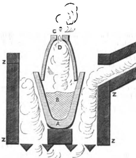
Fig. 226. Preparation of the Anhydrous Teroxide of Antimony. A. Lower crucible standing on a brick in the furnace x x x, and containing the melted antimony B, which, being gradually oxidized, forms the teroxide; and this latter sublimes into the upper inverted crucible, with hole in bottom, C, and condenses at D in needle-shaped crystals.
