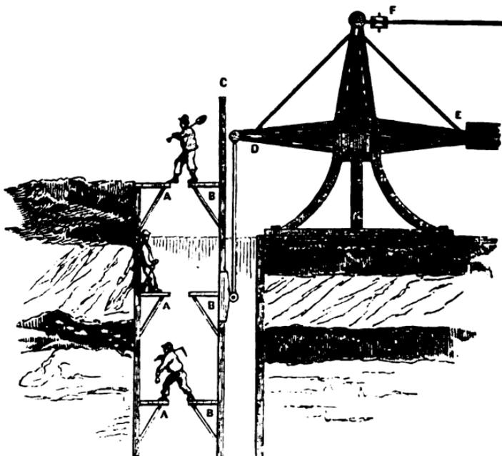
Fig. 165. "The Man Lifter," showing the fixed stages, or shelves, A, A, A, and the moving ones, B, B, B, attached to the rod, C, which is worked by the arm counterpoised by X. The pull is given at F. The man lifter is adopted at the Tressavan mine, which is 350 fathoms deep, and formerly occupied the miners one hour and a quarter to ascend by ladders placed nearly perpendicular.
