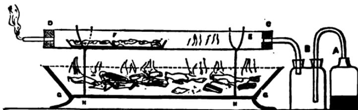
Fig. 221. A. Hydrogen generator. B. Chloride of calcium bottle, for drying the gas. C, D. The Bohemian-glass tube, containing the chloride of aluminium at G, and the tray of sodium at F. H. H. The chafing-dish, containing burning charcoal. E, F. Wire supports for the tube.
