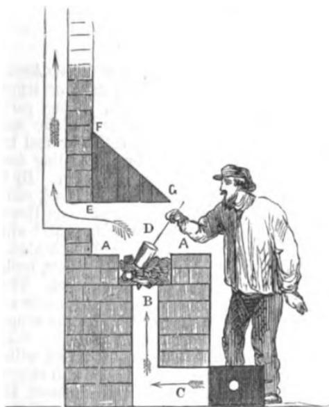
Fig. 160. Roasting Furnace. A A. A square cavity in brickwork, with small grate at *x*, to which air passes from the opening C, closed at pleasure by a door and register. D. The crucible containing the powdered "matt," which is kept at a very low heat, and occasionally stirred with a steel rod; the sulphur is oxidized and carried up the chimney at *x*, and the whole is covered with a hood of sheet iron, *y* e.
