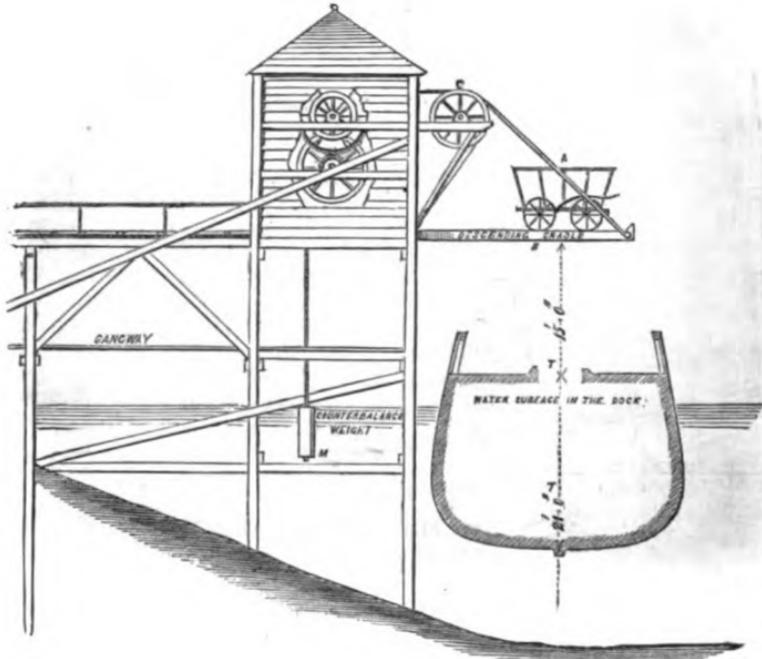
Fig. 67. One of the Forms of Staith Machinery.
