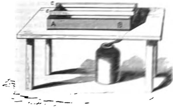
Fig. 100. A. B. The developing stand. C. C. Two glass plates placed on the tray for developing.
