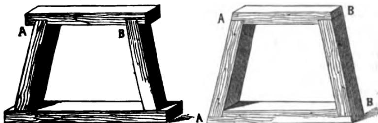
Fig. 196. Timber Supports used in Mines.
