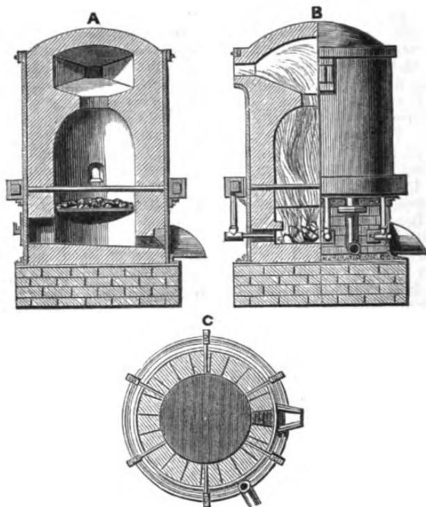
Fig. 206. A, B, C. Sections of Bessemer's apparatus, showing the construction of the iron vessel lined with fire-clay, and the arrangement of the tuyères.
