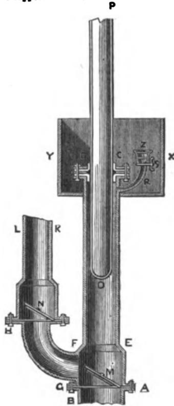
Fig. 198. The Plunger Force-pump.
