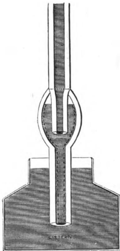
Fig. 169. Negretti and Zambra's ingenious arrangement to prevent the air creeping up the inside of the barometer tube.
