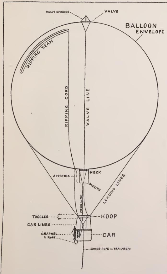
DIAGRAM SHOWING ESSENTIAL PARTS OF A BALLOON.
