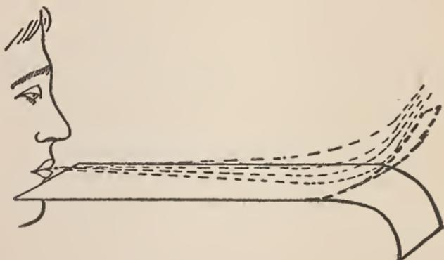
I am not aware if it has been accurately determined what exact proportion of lift is attributable to the partial vacuum above the plane and what to the concave lower surface, but it is obvious from the foregoing that both contribute in greater or lesser degree in attaining the desired result.
