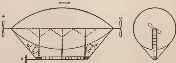
The "Pax," as his balloon was called, was built by Lachambre, and the envelope was made virtually rigid by an inner frame-work. Its cubical capacity was nearly 85,000 feet, and a propeller was placed at each end of the pole which formed the longitudinal axis. The front
