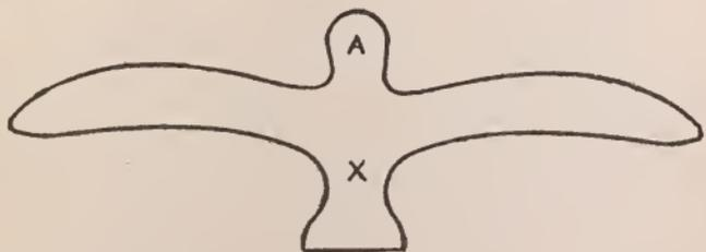
Holding this little flat bird between the thumb and first finger at X, throw it gently away from you and observe the result. You will find that it may skim through the air for a yard or two, then lose its balance, and, according to its height, turn a succession of somersaults until it falls to the ground. There is evidently something wrong in principle with this attempt at a
