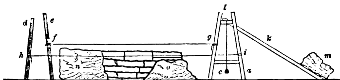
THE FRAME AND COMMENCEMENT OF BUILDING A STONE-DYKE.
