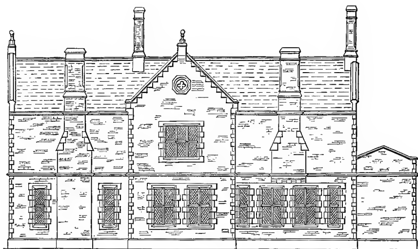
Fig. 711.—Side elevation of farmhouse, finished to show stone-rubble walling—scale in Plate VIII.
