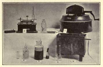
FIG. 70. — Apparatus necessary to test cheese for fat.
