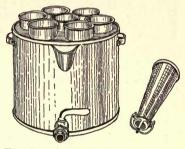
FIG. 4. — A gang sediment tester, one tester removed.
