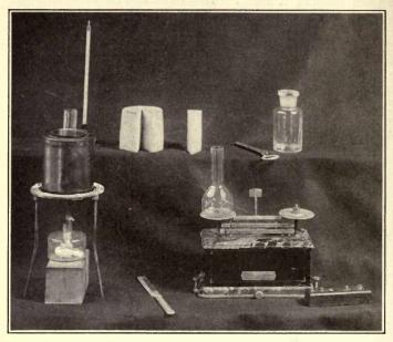
FIG. 73. — Apparatus necessary to test cheese for moisture.
