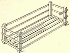
FIG. 14.— Detail of a Neufchâtel draining rack.
