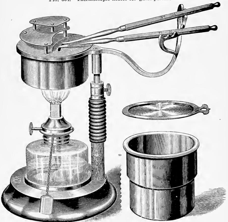
FIG. 355.—Flagg's gutta-percha softener and tool heater.
