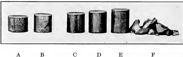
FIG. 339.—Test cylinders of amalgam prepared by amalgamating 6 gm. alloy. Cylinders A and B from low-silver alloy compress and crack. Cylinders C, D, E, and F from high-silver alloy burst explosively. Cylinders B and D, both packed under 400 kg. show difference in size of amalgam from same weight of alloy. D is 25 per cent. larger and 75 per cent. stronger than B. C, D, and E are packed under 141, 400, and 1131 kg. per cir. cm. respectively. Natural size 10 mm. in diameter.
