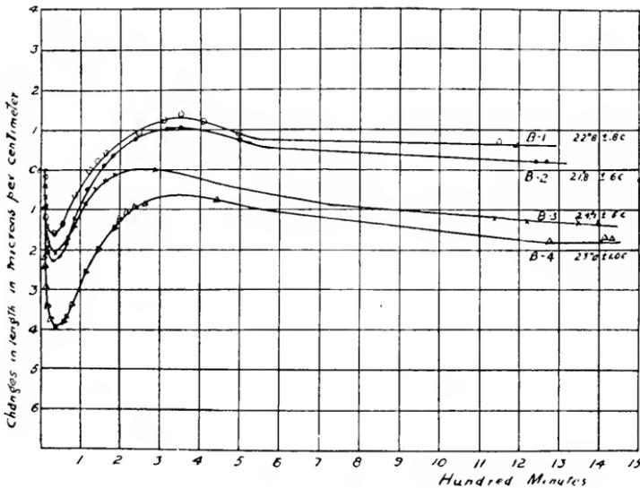
FIG. 342.—Setting changes in amalgam maintained at nearly the same temperature.
