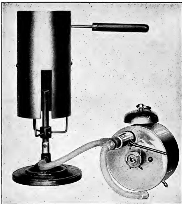
FIG. 232.—Taggart automatic gas apparatus for burning out the wax.<sup>1</sup>
