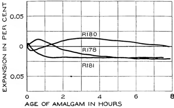
FIG. 341.—Typical reaction expansion curve (R180) and modifications caused by increase of packing pressure.
