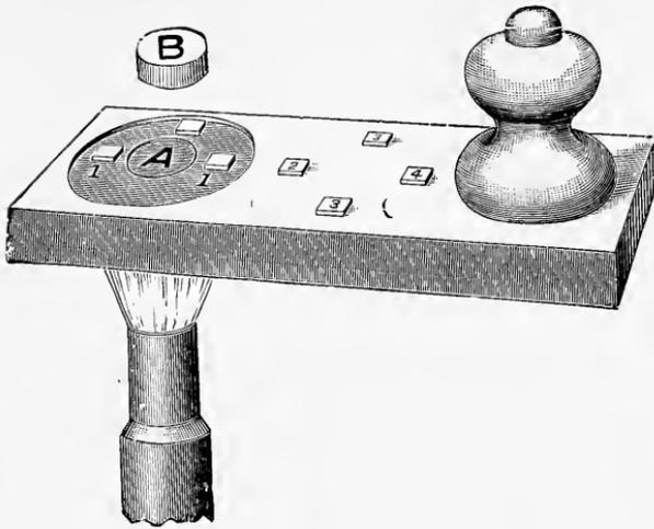
FIG. 354.—Thermoscopic heater for gutta-percha.
