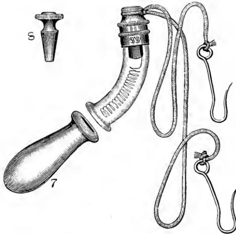
FIG. 405.—Tube electrode.
