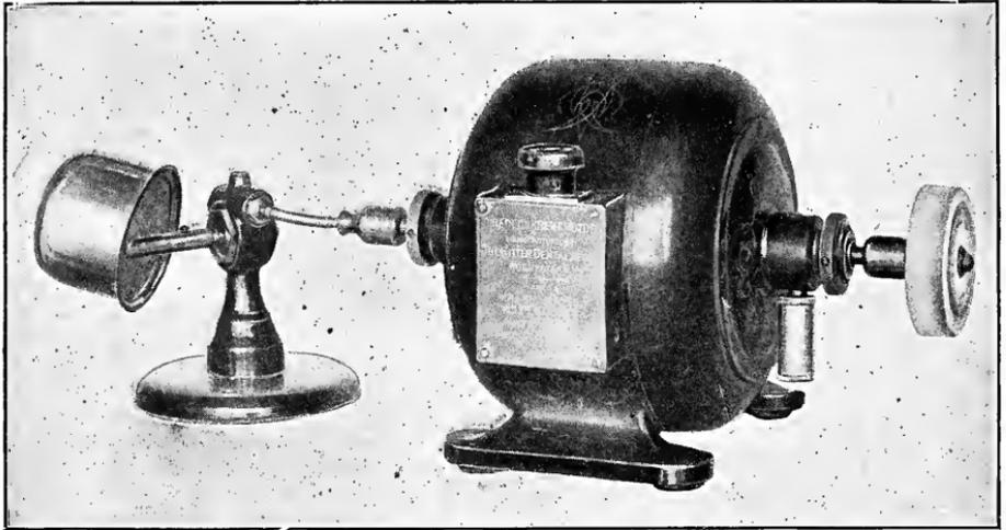
FIG. 228.—Automatic mixer for investing material and water attached to ordinary laboratory lathe. (Suggested by Taggart.)
