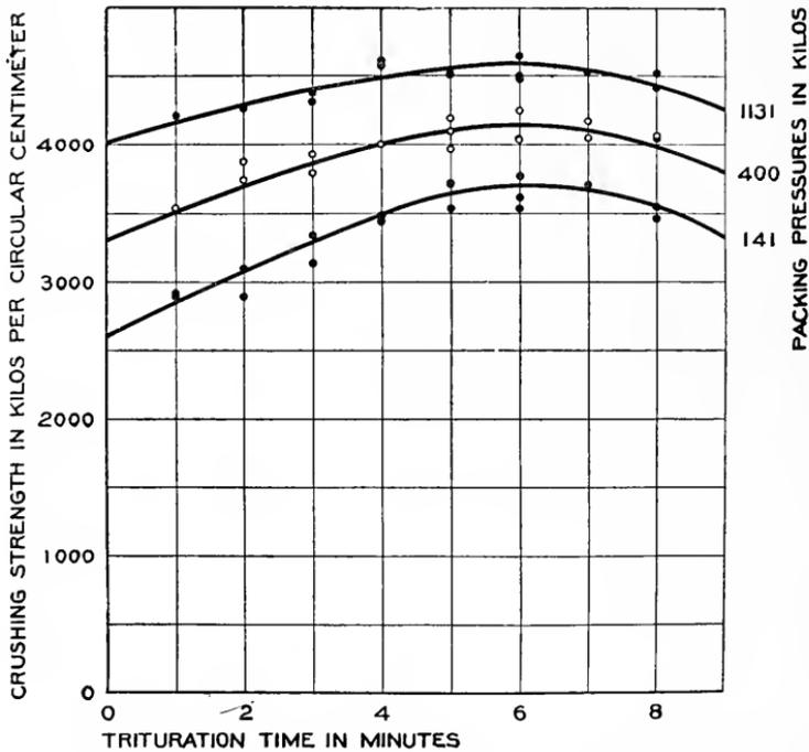
FIG. 348.—Gain in crushing strength produced by increasing trituration time.
