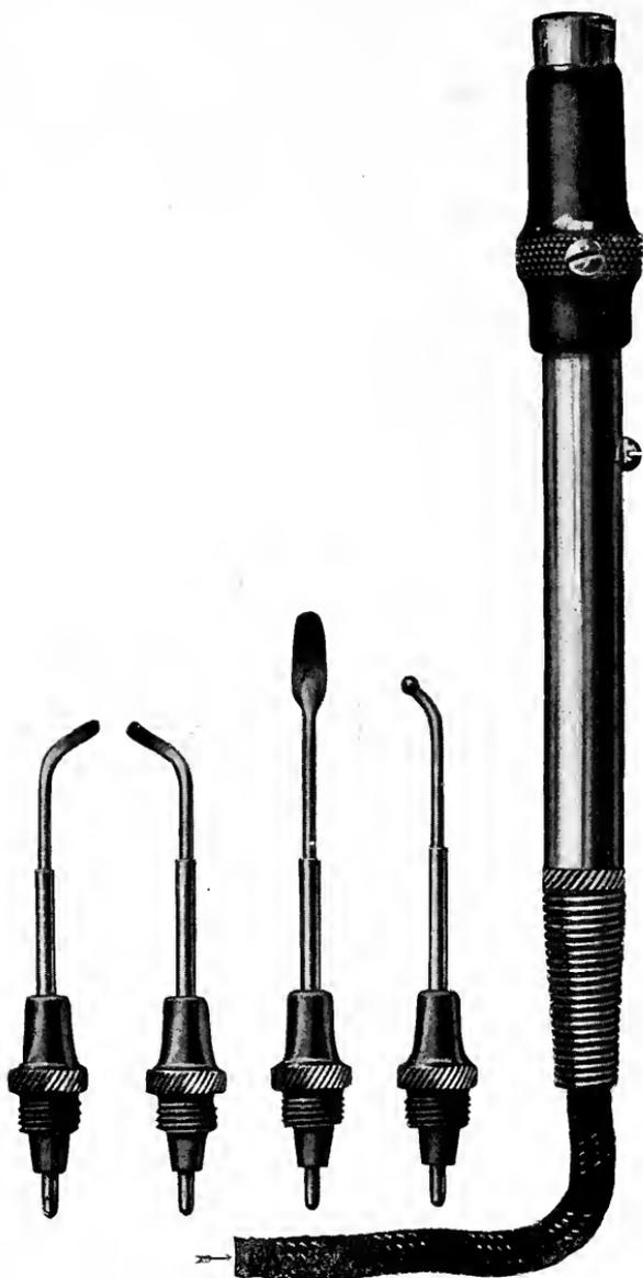
FIG. 356.—Trimmer for gutta-percha heated by electricity.
