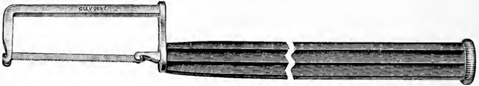
FIG. 188.—G. V. Black's adjustable saw frame.
