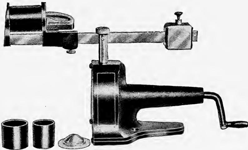
FIG. 234.—Monson's centrifugal casting machine.
