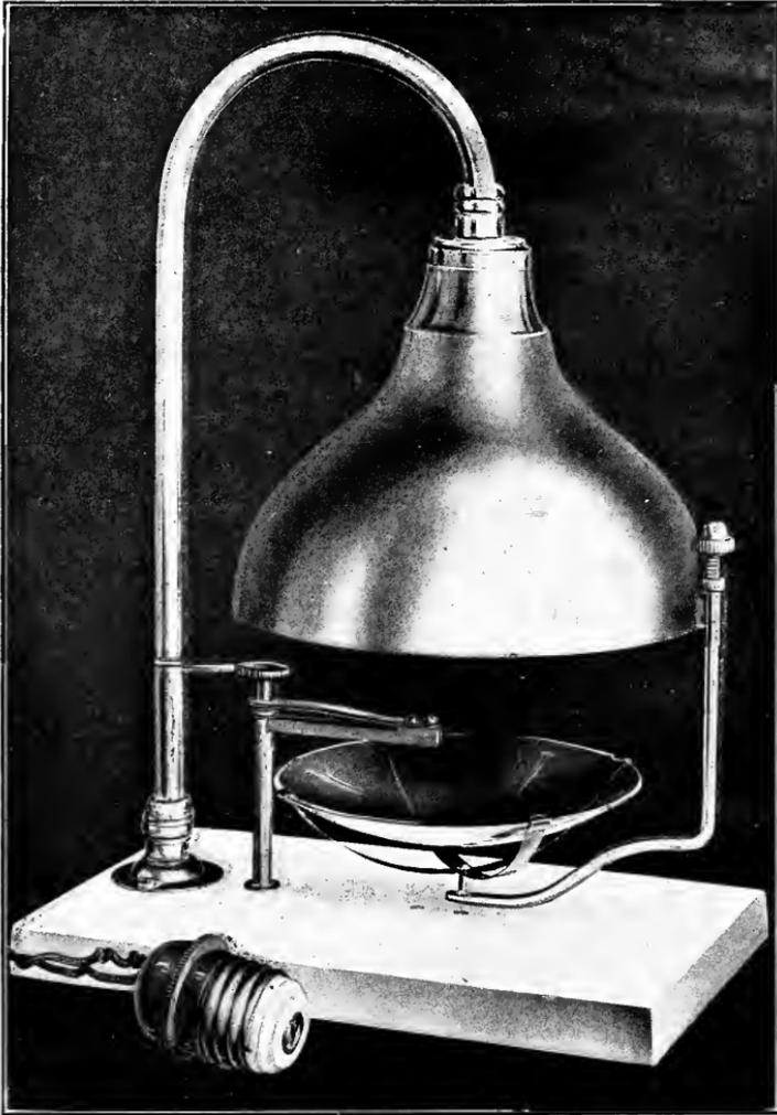
FIG. 223.—Taggart automatic heater for casting wax.
