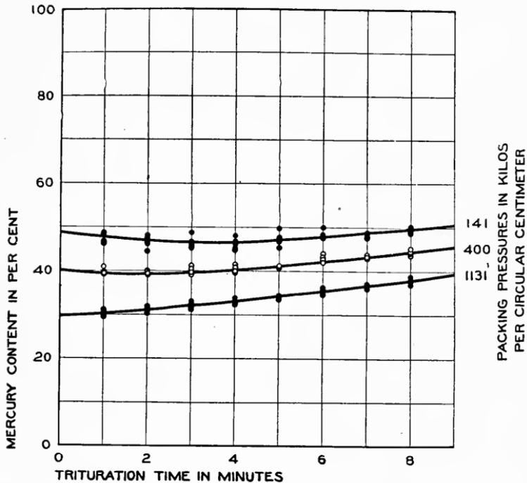
FIG. 353.—Percentage of mercury in an amalgam filling is less when high pressure has been used to pack it than when low pressure has been used.
