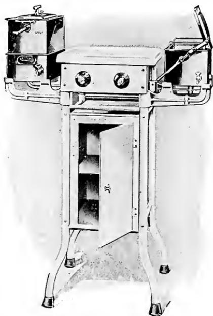
FIG. 368.—Steam chest sterilizer. Moist heat may be obtained varying from 190° F. to 215° F. and can be maintained for an indefinite period. It is necessary to maintain this temperature at least thirty minutes and is safer to sterilize three successive days before using the materials under sterilization. Especially useful for materials used in root-canal operations as Fig. 367.
