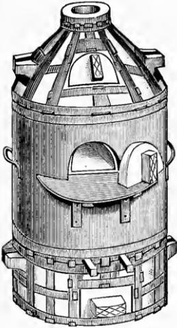
FIG. 336.—Old style coke furnace.
