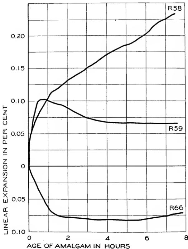
FIG. 343.—Effects of changing size of alloy particles.
