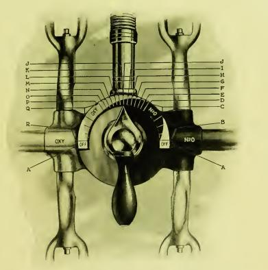
Figure 12. The A. C. Clark valve regulator, indicating the ascending and descending mixtures of nitrous oxid and oxygen as the handle is turned to left or right.
