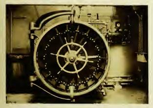
Large autoclave for sterilization, with live steam under pressure, of syringes and other containers, and ampuls containing hypodermic solutions.
