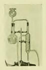
Figure 1. Silverman's apparatus for distilling water.
