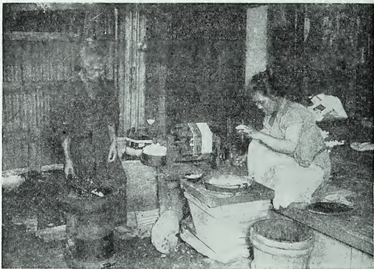
Top, sorting and weighing cocoons in preparation for the market. Bottom, hand reeling of silk in the home. A pan of hot water placed over a charcoal burner affords a means of softening the gum.
