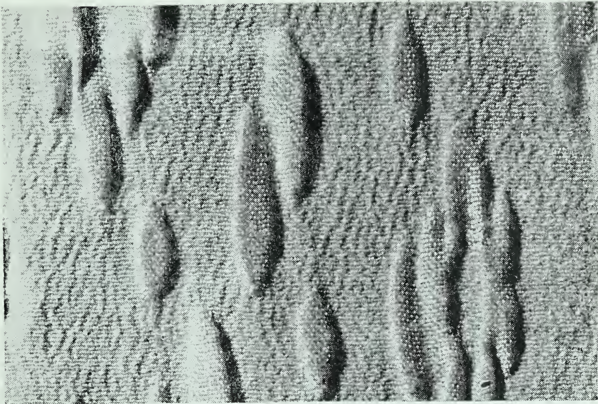
Matelassé. Raised design produced with a third set of yarns.
