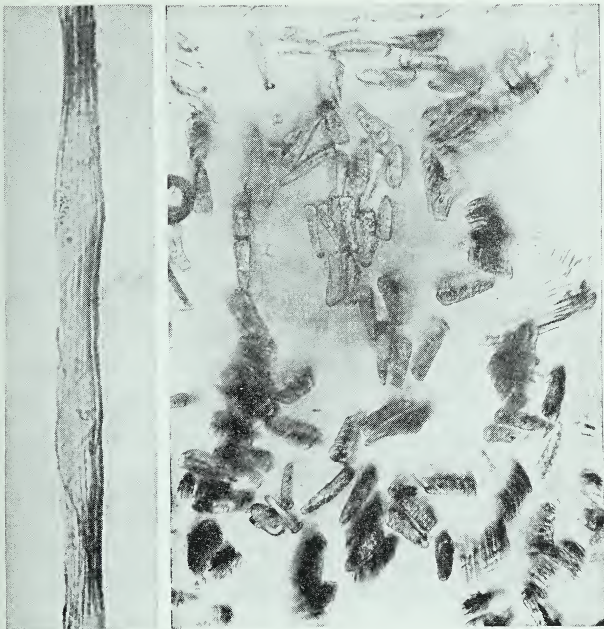
Photomicrographs of longitudinal and cross sections of wild silk. Note width of fiber as shown in cross section.
