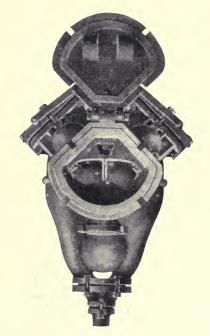
Fig. 38. "Free-way" Pulsometer Pump.
