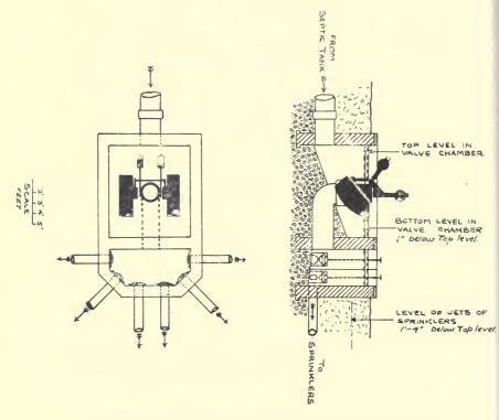
Fig. 43A. Showing Intermitting Valve Dosing to Six Sprinklers.
