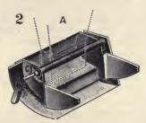
Fig. 5A. Mechanism of Moule's "Chucker" Action Closet.
