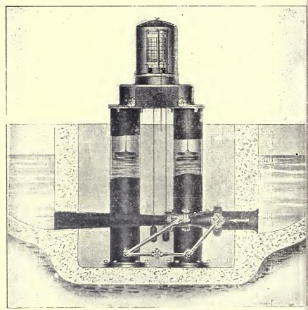
Fig. 30. Kent's "Venturi" Meter.
