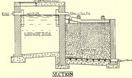
Fig. 22A. Section of Farrer's Single-section Distributor.
