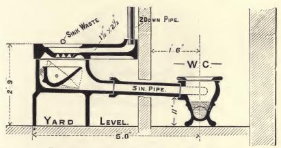
Fig. 6A. Section of Duckett's Slop Water-closet.
