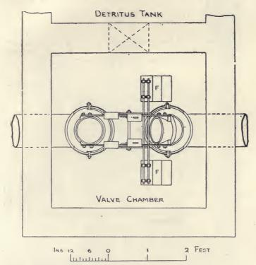
Fig. 37. Plan of Automatic "Cut-out" Valve.
