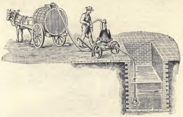
Fig. 8. Honig & Mock's Single-acting Diaphragm Pump.
