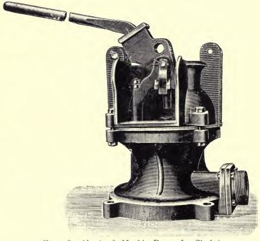
Fig. 28. Honig & Mock's Pump for Sludging.
