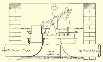
Fig. 37A. Section of Automatic "Cut Out" Valve.
