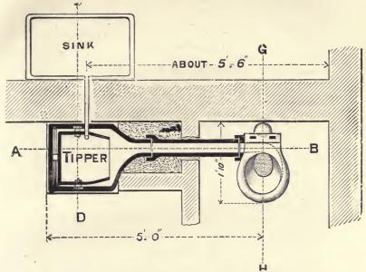
Fig. 6. Plan of Duckett's Slop Water-closet.
