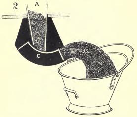
Fig. 5. Moule's "Chucker" Action Closet.
