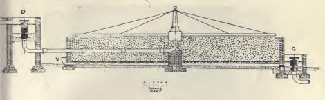
Fig 43B. Showing Dosing and Aeration of Filters by Intermitting Valves.
