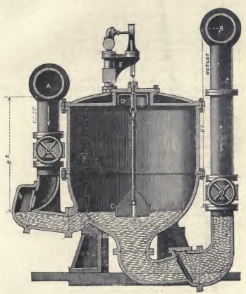
Fig. 37B. Section of "Shone" Ejector.
