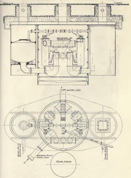
Fig. 37c. "Coombs" Pneumatic Ejector.
