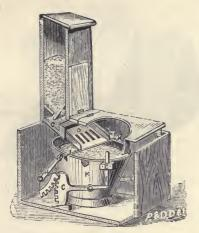
Fig. 4. British Sanitary Co.'s Self-acting Earth Closet,
