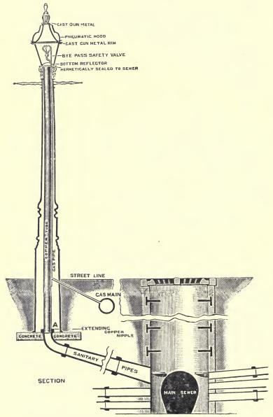
Fig. 12. Section, Webb's System of Sewer Ventilation.
