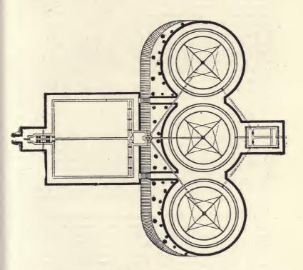
Fig. 51. General Arrangement of Three "Filters."
