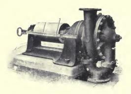
Fig. 39. Tan-gyro Centrifugal Pump.
