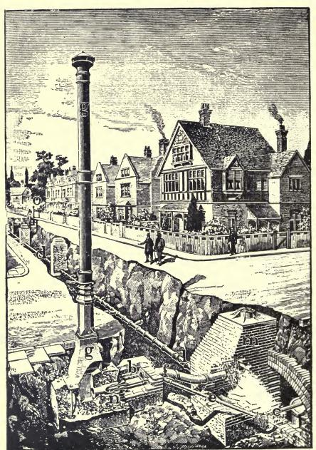
Fig. 11. Shone & Ault's Sewer Ventilating System.
