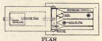
Fig. 22. Plan of Farrer's Single-section Distributor.
