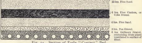
Fig. 14. Section of Early "Contact" Bed.
