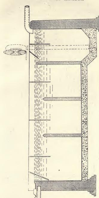
Longitudinal Section of Stoddart's Continuous Filter, 15. Fig.
