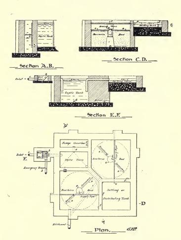
Fig. 24. Detailed Plan of Installation for Country Mansion.
