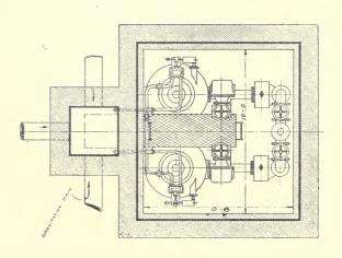
Fig. 37F. Two "Coombs" Ejectors in Brick Chamber.
