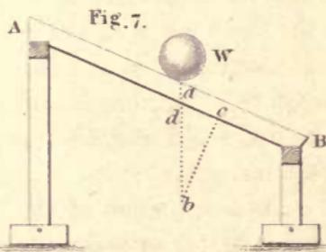
*of which are represented in magnitude and direction by two sides of a triangle, the third side will represent the magnitude and direction of the other force.*
